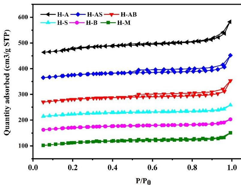
Figure S8. N<sub>2</sub> adsorption/desorption isotherms of ZSM-5 samples.
