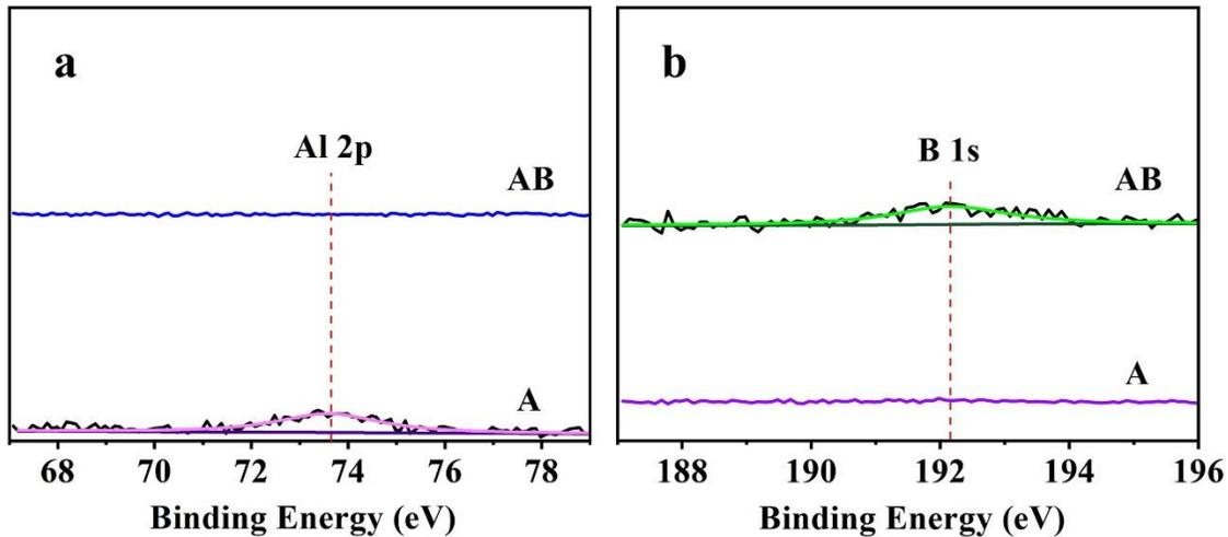
**Figure S7.** XPS spectra of (a) Al 2p and (b) B 1s peaks for ZSM-5 samples
