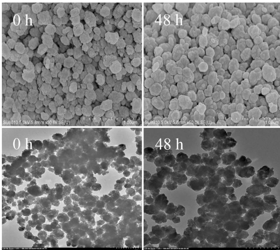
**Figure S1.** SEM and TEM images of A sample before and after TPAOH treatment
