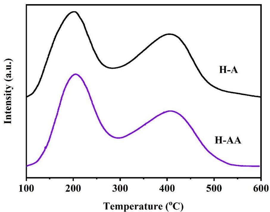
Figure S13. NH<sub>3</sub>-TPD profiles of H-A and H-AA samples
