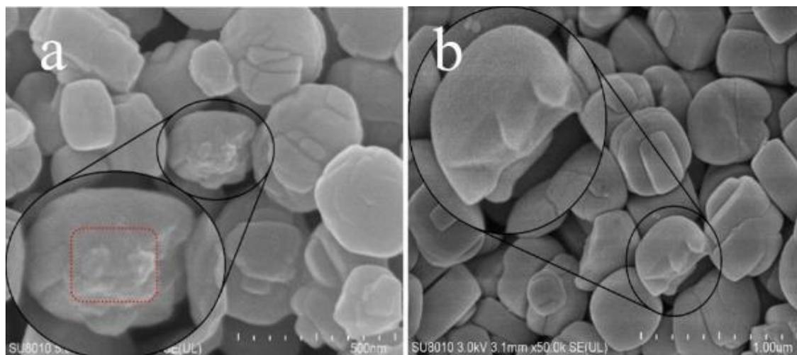
**Figure S5.** SEM images of fractured particles of (a) AB sample and (b) B sample.
