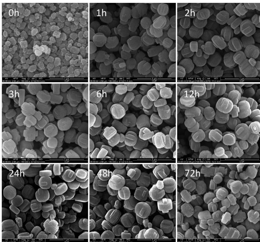
**Figure S4.** SEM images of AB sample at different crystallization time.
