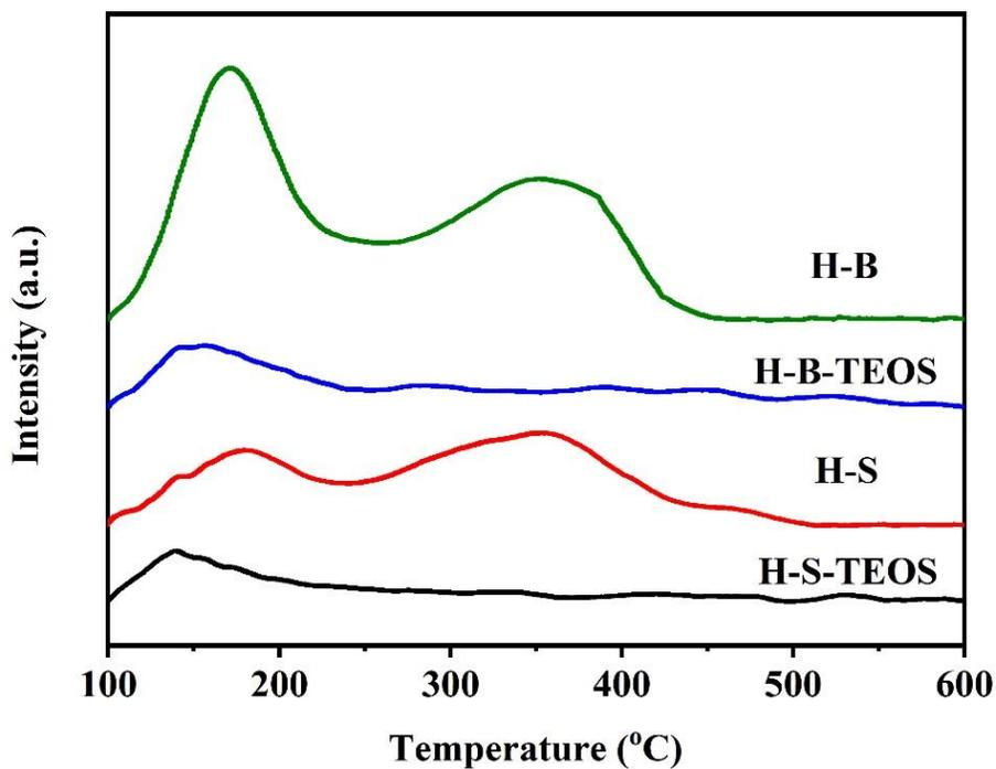
Figure S9. NH<sub>3</sub>-TPD profiles of ZSM-5 samples
