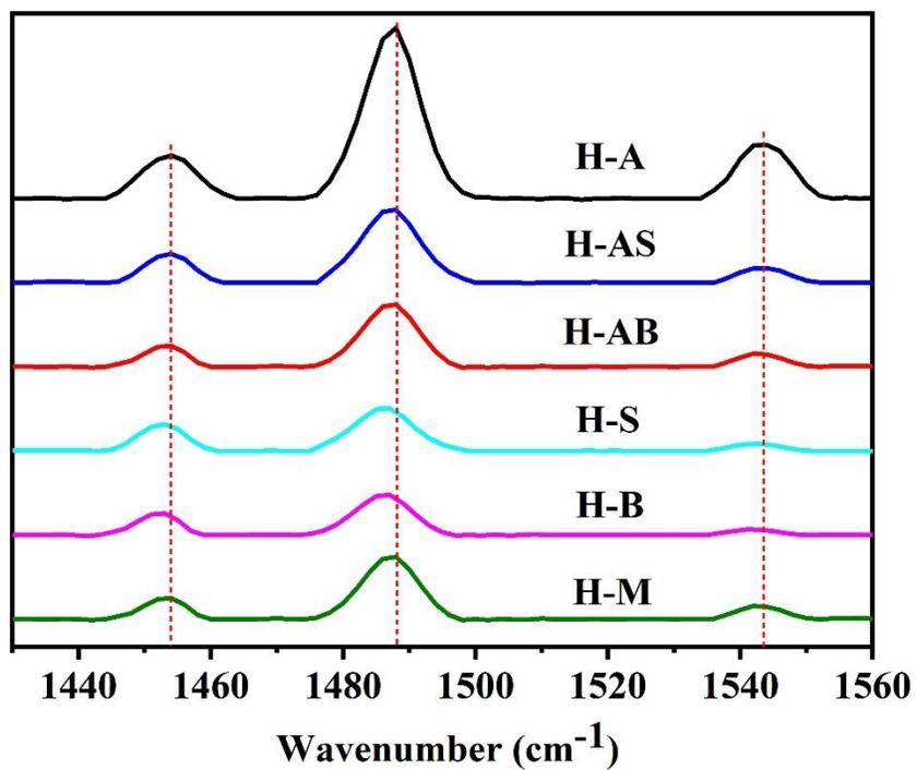
Figure S11. Py-IR spectra of ZSM-5 samples at 350 °C
