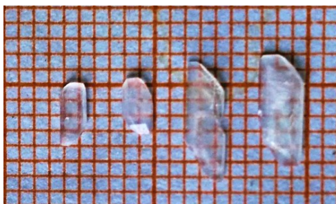
Figure S1 The block crystal of compound 1.
