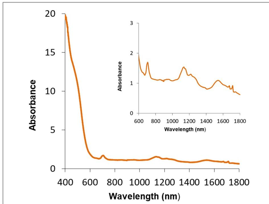
**Figure S1.** Room temperature UV-vis-NIR absorption spectra for complex  $[\text{U}\{\kappa^3\text{-H(R)B(tim}^{\text{Me}}\}_2\}_3\text{I}]$  **6-I** in acetonitrile.
