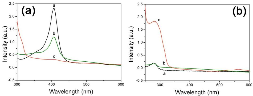
Fig. S8 Curve a is the UV-vis spectrum of  $0.4 \text{ mg mL}^{-1}$  of the BSA and BSA mixture (a), BSA (b) before adsorption by  $C@CoNi/500$ . Curve b is the UV-vis spectrum of supernatant of, BSA and BSA mixture (a), BSA (b) after adsorbed by  $C@CoNi/500$ . Curve c is the UV-vis spectrum of desorption solution of the adsorbed protein by  $C@CoNi/500$  in, BSA and BSA mixture (a), BSA (b) using concentration of  $0.2 \text{ g mL}^{-1}$  of dimethyl imidazole solution as the eluent.
