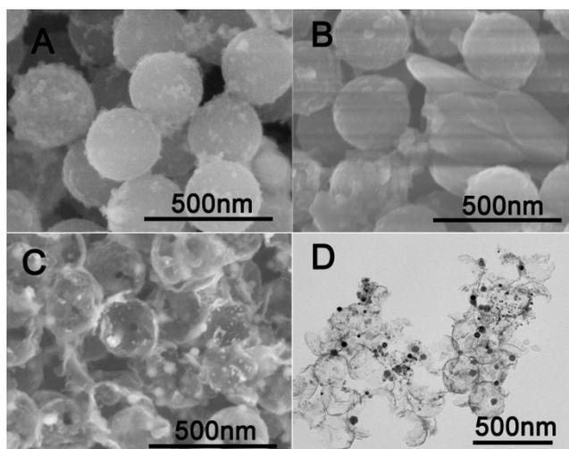
Fig. S3 SEM images of CPS@Ni-Al (A); CPS@Ni-Al@PDA (B); C@NiAl (C) and TEM image of C@NiAl (D).
