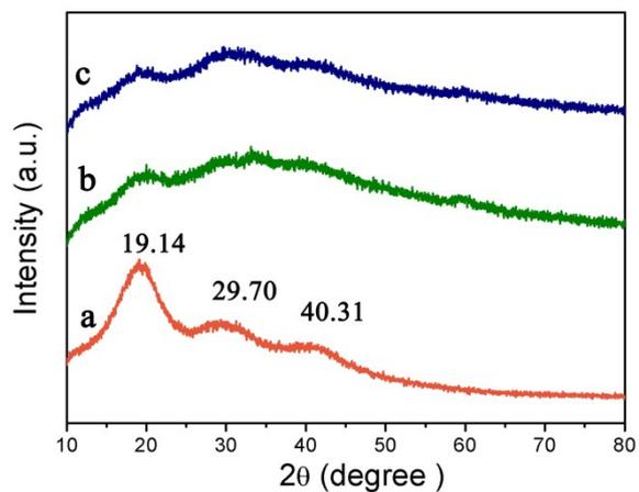
Fig . S2 XRD diffraction patterns of CPS (a); CPS@Ni-Co (b) and CPS@Ni-Co@PDA (c).
