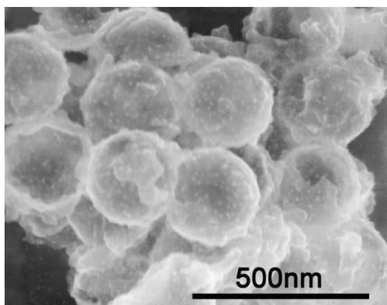
Fig. S7 SEM images of C@CoNi/500 after five catalytic reaction
