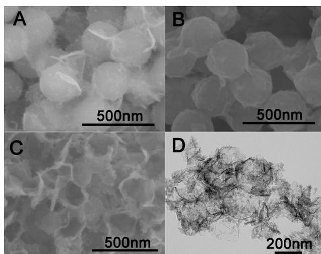
Fig. S4 SEM images of CPS@Co-Mn (A); CPS@Co-Mn@PDA(B); C@CoMn (C) and TEM image of C@CoMn (D).
