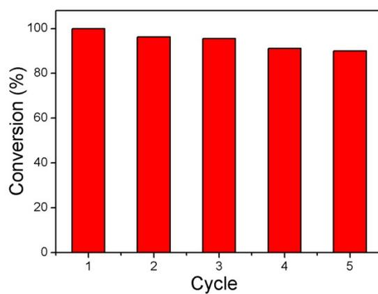
Fig. S6 The reusability of C@CoNi/500 as the catalyst for the reduction of 4-NP with NaBH<sub>4</sub>.
