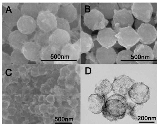
Fig. S5 SEM images of CPS@Ni-Mn (A); CPS@Ni-Mn@PDA (B); C@NiMn (C) and TEM image of C@NiMn (D).
