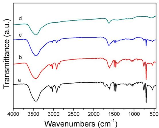
Fig. S1 FT-IR spectra of CP (a); CPS@Ni-Co (b); CPS@Ni-Co@PDA (c) and C@CoNi/500 (d).
