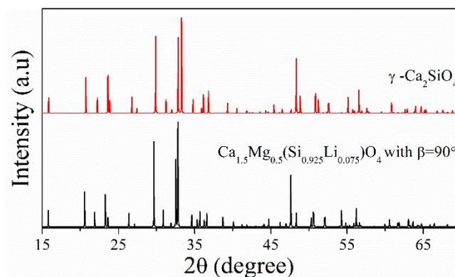
**Figure S2.** X-ray diffractograms of  $\gamma$ -Ca<sub>2</sub>SiO<sub>4</sub> and Ca<sub>1.51(1)</sub>Mg<sub>0.49(1)</sub>Si<sub>0.925(5)</sub>Li<sub>0.075(5)</sub>O<sub>4</sub> with  $\beta = 90^\circ$ .
