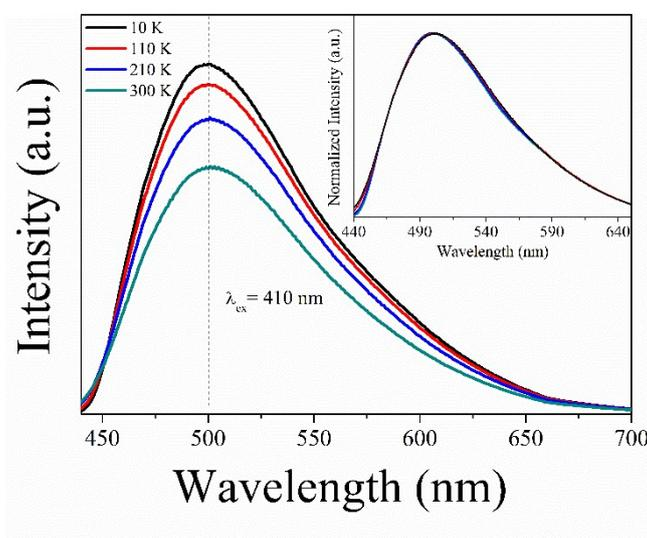
**Figure S5.** The low-temperature emission spectra ( $\lambda_{\text{ex}} = 410$  nm) of the CMSL:0.005Ce phosphor.
