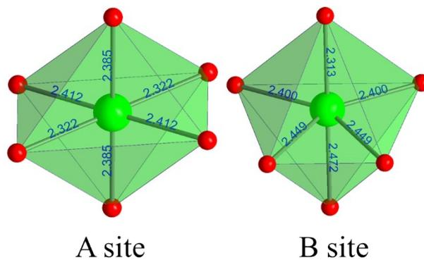
**Figure S3.** Coordination polyhedra of two kinds of Ca sites in  $\gamma$ -Ca<sub>2</sub>SiO<sub>4</sub>. The green spheres correspond to Ca, and the red spheres to O. The average coordination distances of A and B sites are 2.352 Å and 2.359 Å, respectively.
