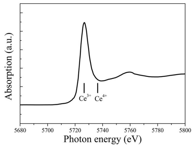
**Figure S6.** Ce LIII-edge XANES spectrum of CMSL:0.01Ce fine powder. The positions of  $\text{Ce}^{3+}$  and  $\text{Ce}^{4+}$  are marked. There is no evidence for  $\text{Ce}^{4+}$  in this sample.
