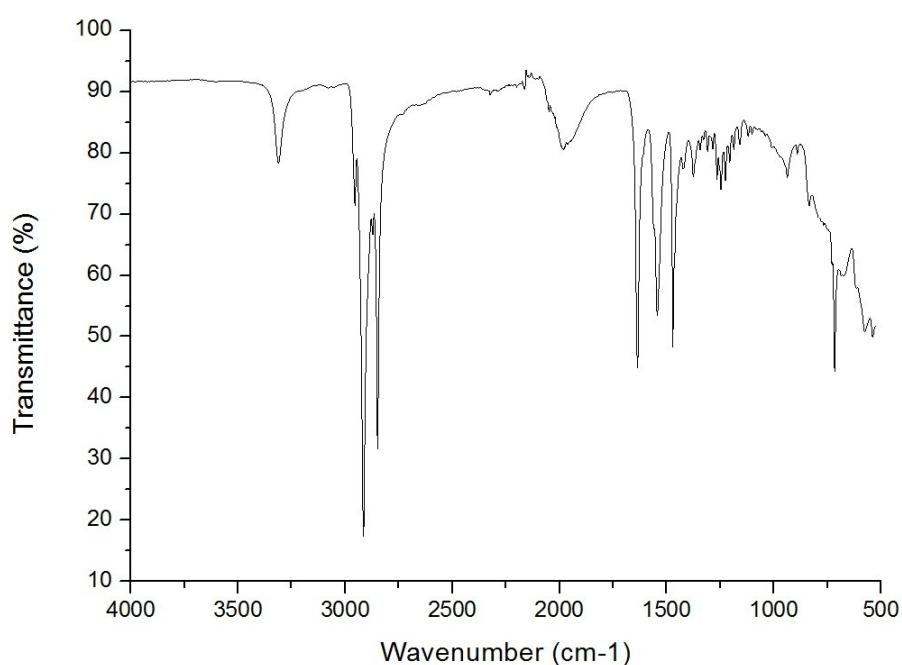
Figure S21. IR spectrum of the NPs prepared from **2b** in the presence of 1 equiv. HDA and 1 equiv. PA at 200°C.
