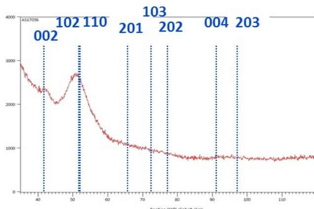
Figure S22. Powder XRD of iron germanide NPs prepared from **2b** in the presence of 1 equiv. HDA and 1 equiv. of PA at 200°C.
