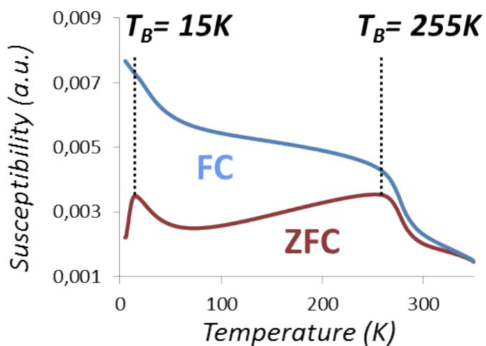
Figure S7. VSM of the NPs prepared from **2a** in the presence of 0.5 equiv. HDA at 200°C.
