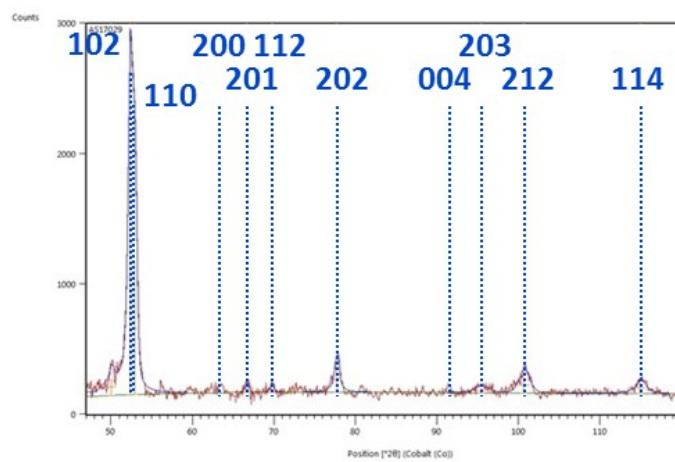
Figure S6. XRD diffractogram of the NPs prepared from **2a** in the presence of 0.5 equiv. HDA at 200°C.
