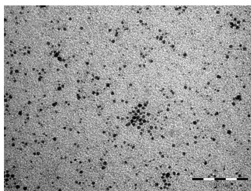
Figure S19. TEM pictures of the NPs prepared from **2b** in the presence of 1 equiv. PA at 200°C.
