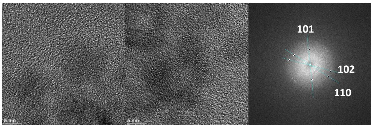
Figure S23 HRTEM and SAED of iron germanide NPs prepared from **2b** in the presence of 1 equiv. HDA and 1 equiv. of PA at 200°C.
