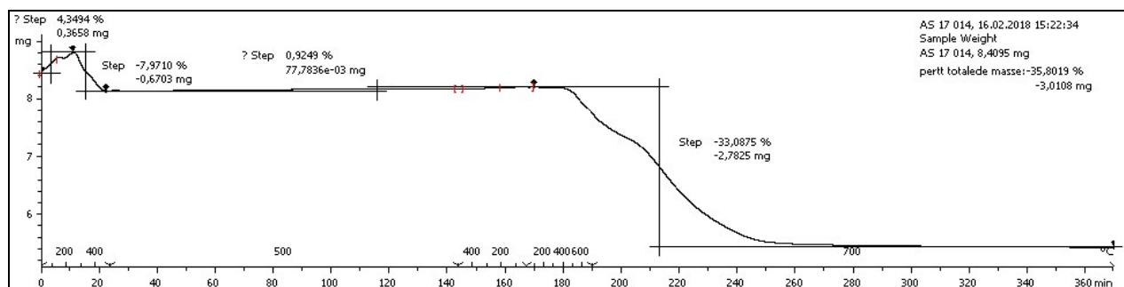
Figure S4. Thermal gravimetric analyses of the NPs prepared from **2a** in the presence of 0.5 equiv. HDA at 200°C.
