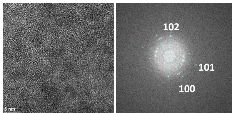
Figure S20. HRTEM and SAED pictures of the NPs prepared from **2b** in the presence of 1 equiv. PA at 200°C.
