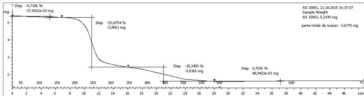
Figure S1. Thermal gravimetric analyses of complex **2a**.
