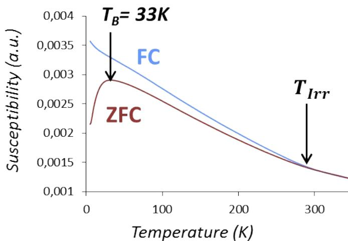
Figure S9. VSM of iron germanide NPs prepared from **2a** in the presence of 1 equiv. HDA and 1 equiv. of PA at 200°C.
