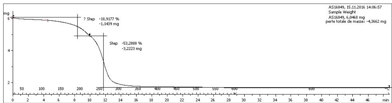
Figure S15. Thermal gravimetric analyses of complex **2b**.
