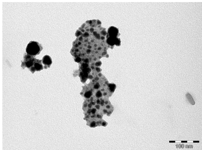
Figure S2. TEM pictures of the NPs prepared from **2a** in the presence of 0.5 equiv. HDA at 200°C.
