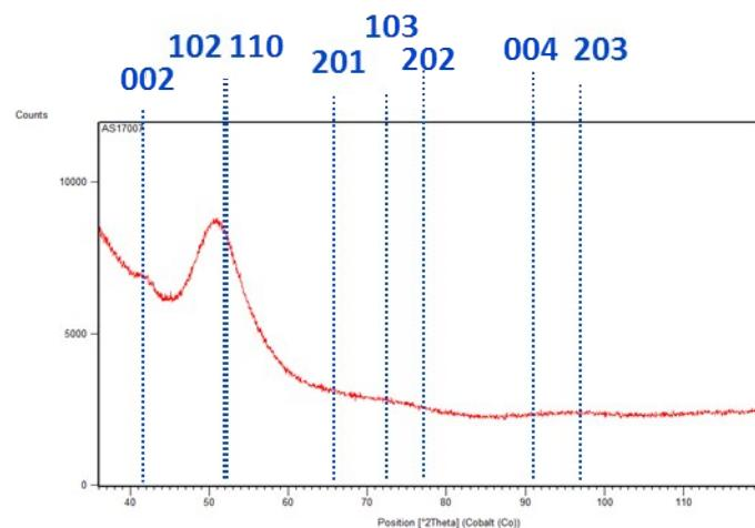
Figure S18. XRD diffractogram of the NPs prepared from **2b** in the presence of 0.5 equiv. HDA at 200°C.
