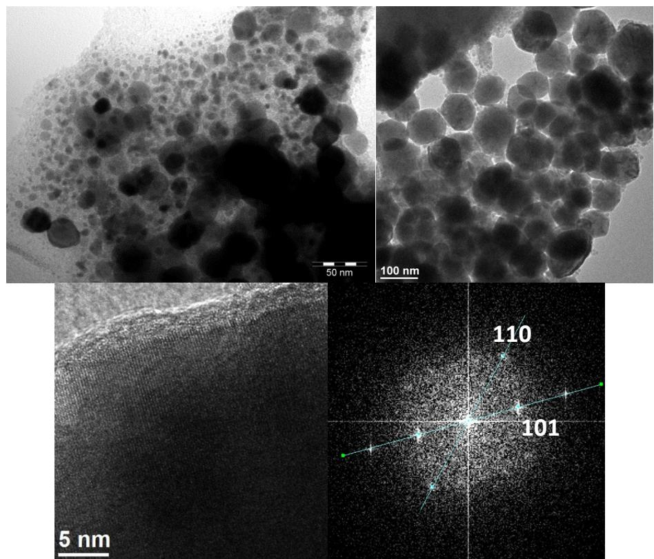
Figure S8. TEM, HRTEM pictures and SAED pattern for NPs of the NPs prepared from **2a** in the presence of 1 equiv. HDA and 1 equiv. PA at 200°C.
