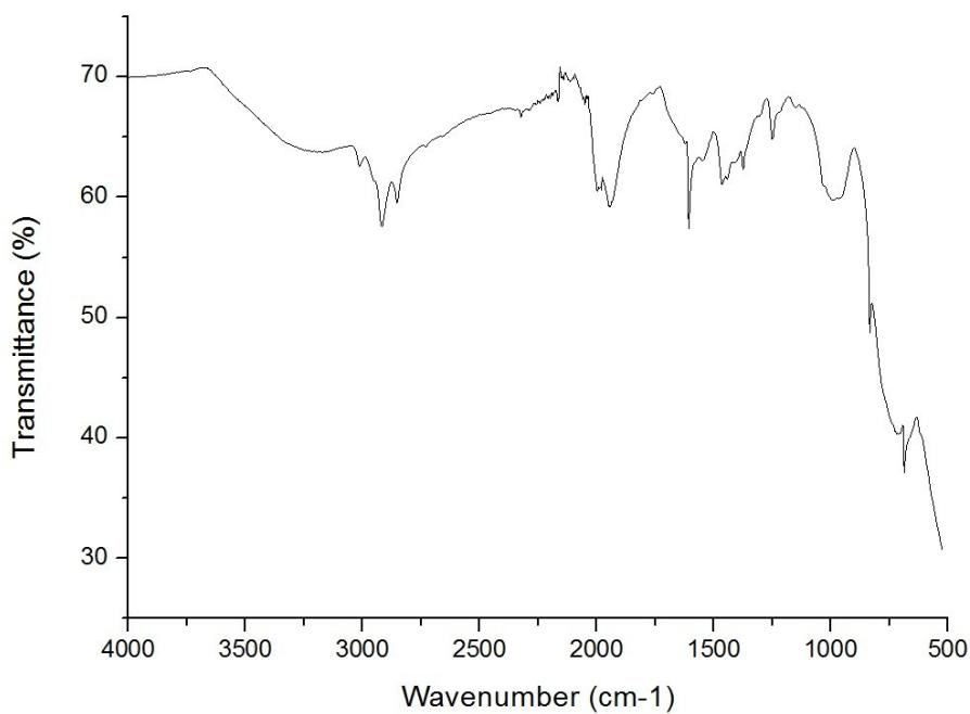
Figure S17. IR spectrum of the NPs prepared from **2b** in the presence of 0.5 equiv. HDA at 200°C.
