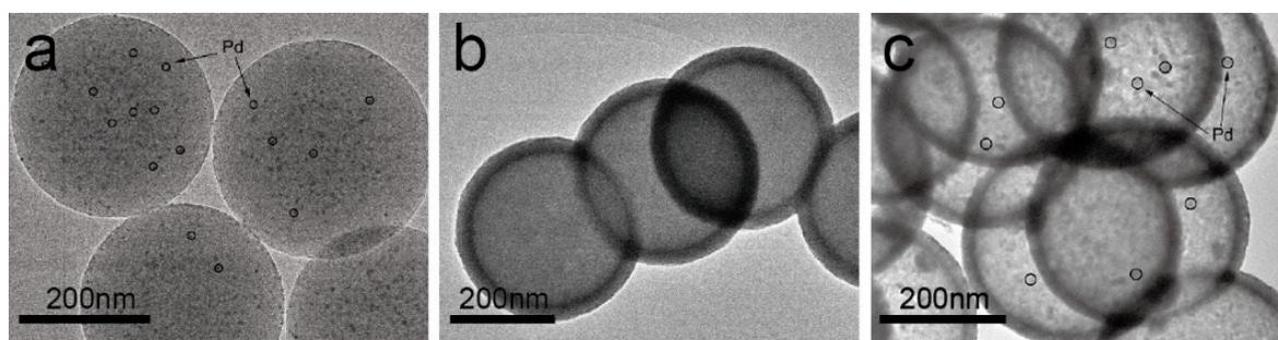
Figure.S5. TEM images of products obtained at each stage during the whole process for preparing yolk-shell structured  $\text{Pd}@\text{ZrO}_2$  nanocatalyst, (a) RF/Pd after annealing in Ar, (b) RF/Pd@ZrO<sub>2</sub> (c) Pd@ZrO<sub>2</sub>
