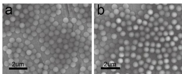
Figure.S1. SEM images of PS before (a) and after (b) zirconium oxide surface coating
