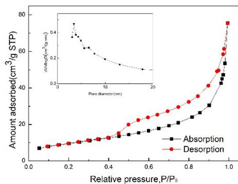
Figure.S7. Nitrogen adsorption-desorption isotherms and pore size distribution of Pd@ZrO<sub>2</sub>
