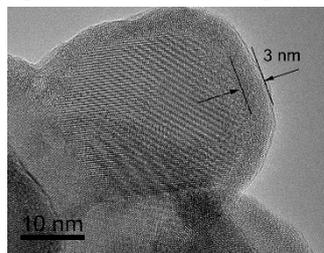
Figure.S3. TEM image of  $\text{TiO}_2@\text{ZrO}_2$
