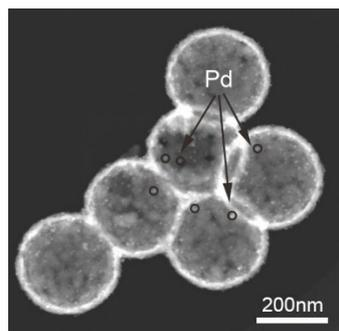
Figure.S6. A DF-STEM image of Pd@ZrO<sub>2</sub>
