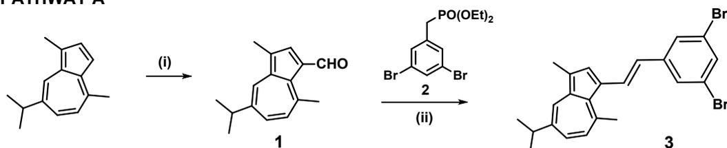
Reagents and conditions: (i)  $\text{POCl}_3$ , 1,2-dichloroethane, DMF, rt then  $80^\circ\text{C}$ , 20 min; (ii) *t*-BuOK, THF, Ar,  $0^\circ\text{C}$ , then rt, 15 h.
