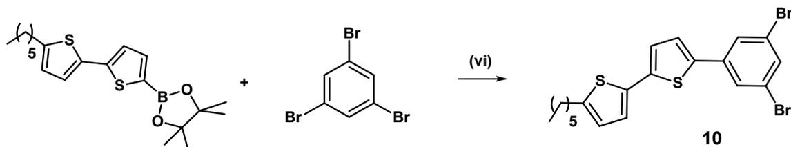
Reagents and conditions: (vi)  $\text{Pd}(\text{PPh}_3)_4$ ,  $\text{Na}_2\text{CO}_3$ , THF/ $\text{H}_2\text{O}$ ,  $90^\circ\text{C}$ , 24 h.
