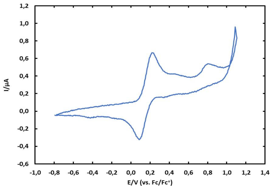
**Figure S16.** Cyclic Voltammogram of Au-Ru complex **1c**.
