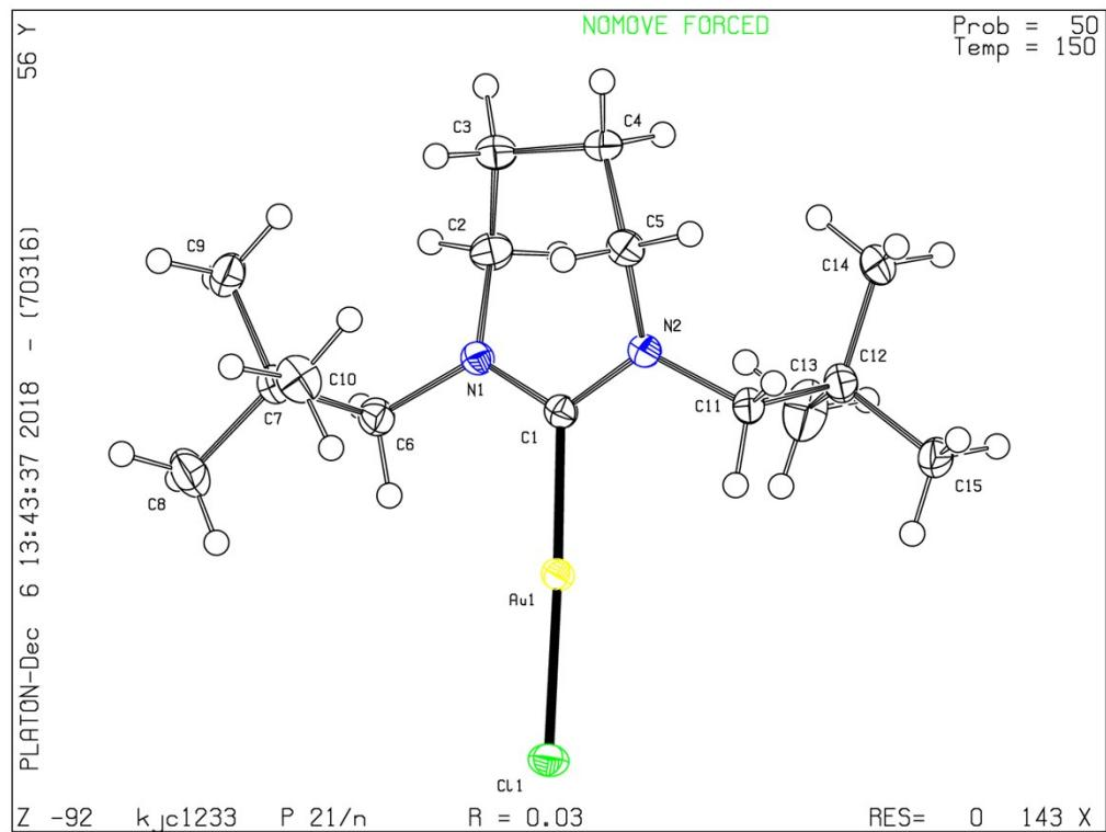
Figure 8: Platon representation of the structure of compound 8.
