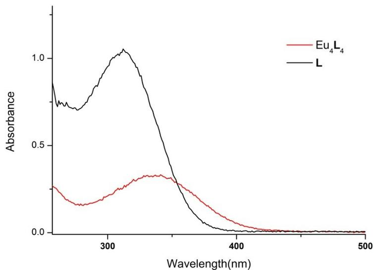
**Figure S30.** UV-Vis spectra of **L** ( $1 \times 10^{-5}$  M in DMSO) and  $\text{Eu}_4\text{L}_4(\text{OTf})_{12}$  ( $0.25 \times 10^{-5}$  M in  $\text{CH}_3\text{CN}$ )
