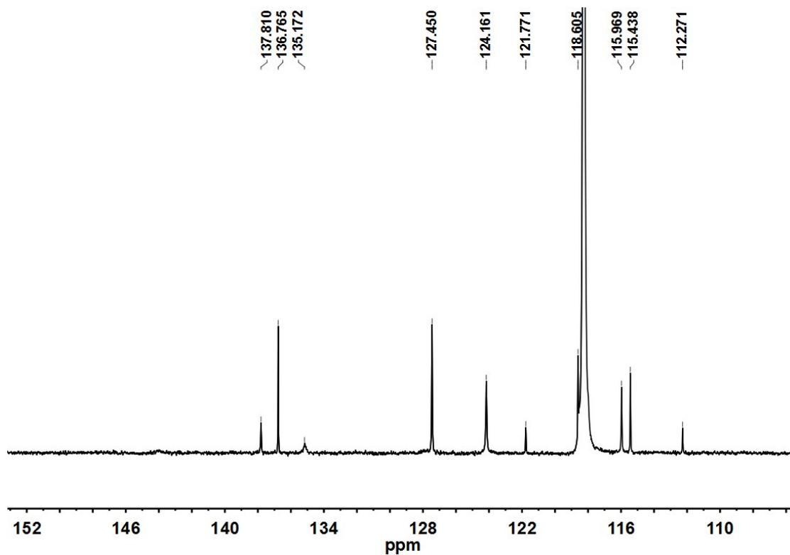
**Figure S22.**  $^{13}\text{C}$  NMR spectrum of the self-assembly complex of  $\text{L}'$  and  $\text{Eu}(\text{OTf})_3$  (100 MHz,  $\text{CD}_3\text{CN}$ , 298 K).
