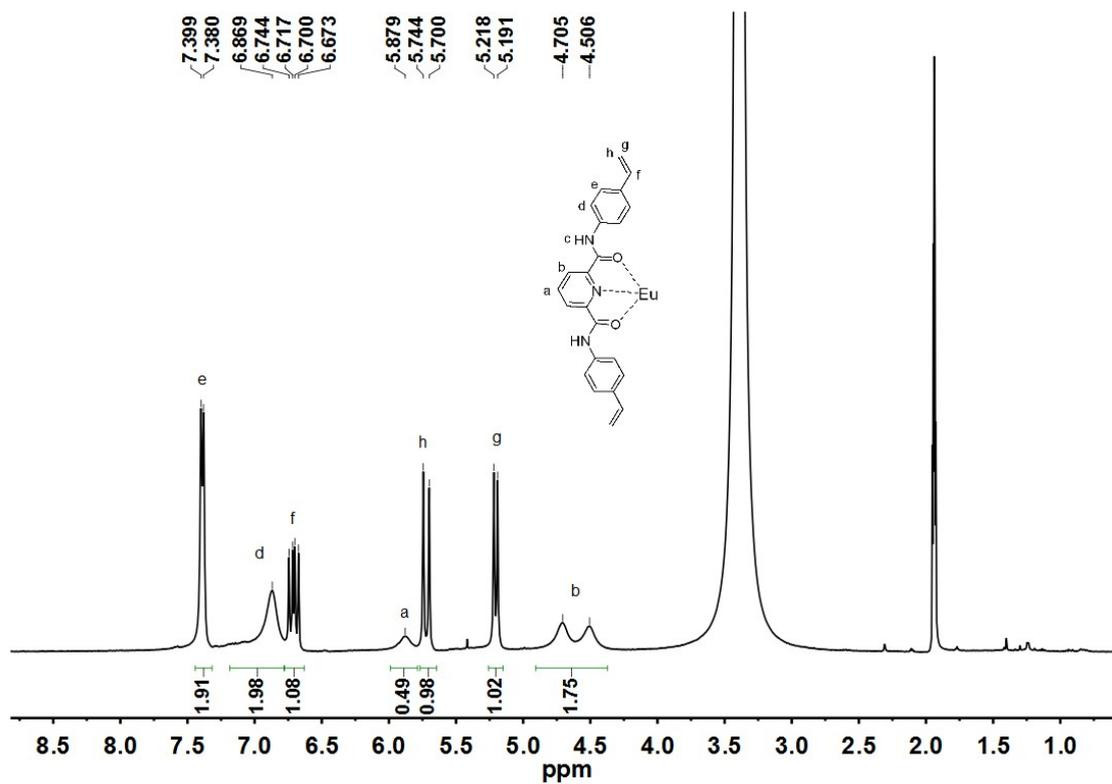
**Figure S21.**  $^1\text{H}$  NMR spectrum of the self-assembly complex of  $\text{L}'$  and  $\text{Eu}(\text{OTf})_3$  (400 MHz,  $\text{CD}_3\text{CN}$ , 298 K).
