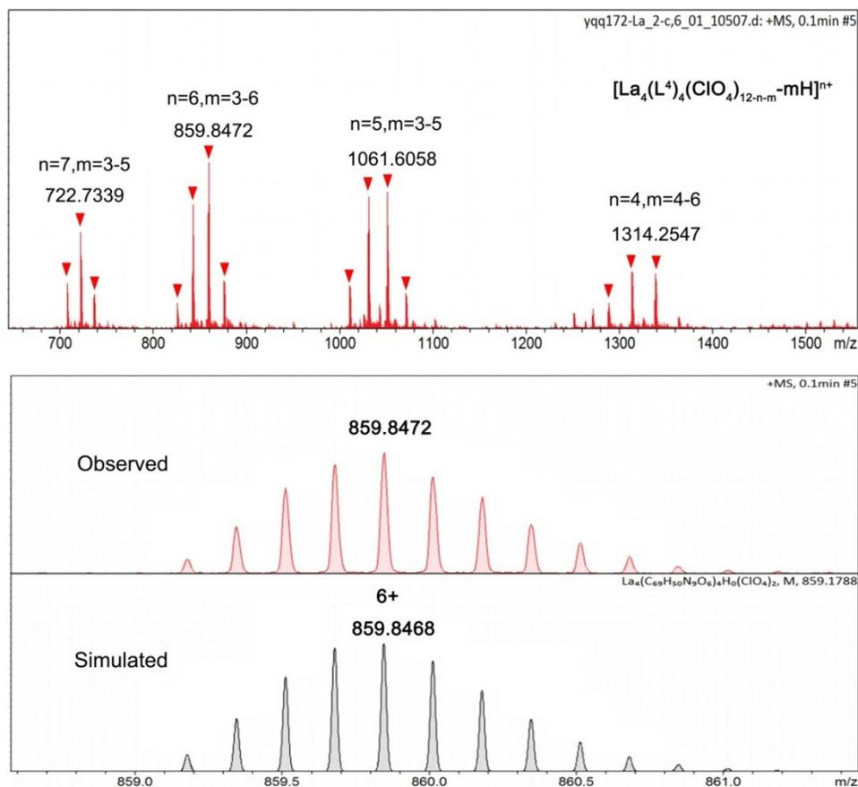
**Figure S20.** ESI-TOF-MS of the self-assembly complex of **L** and  $\text{La}(\text{ClO}_4)_3 \cdot 6\text{H}_2\text{O}$ .
