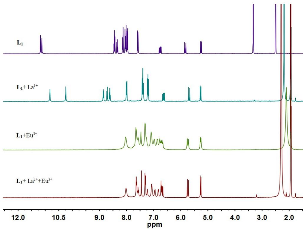
**Figure S23.**  $^1\text{H}$  NMR spectra for the mixed-metal self-sorting studies of  $\text{Ln}_4(\text{L})_4$  (400 MHz,  $\text{CD}_3\text{CN}$ , 298 K).
