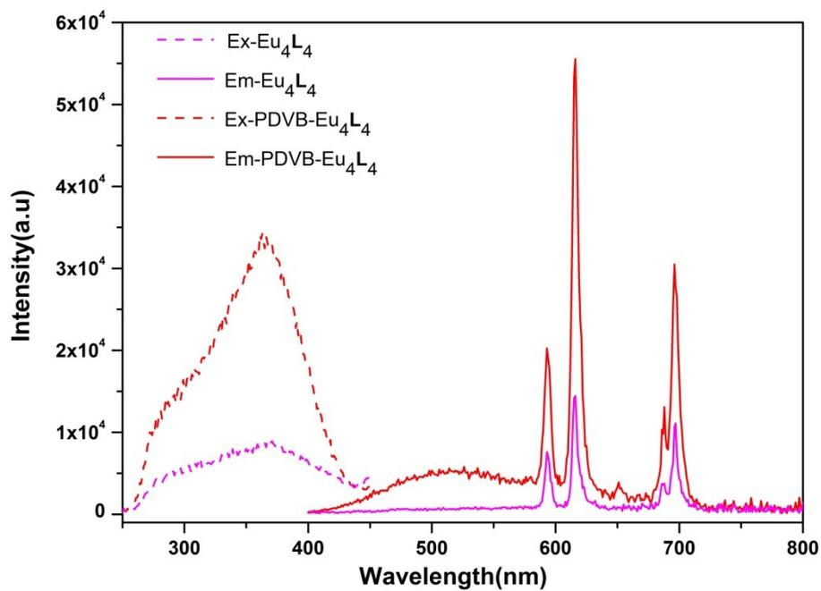
**Figure S31.** Excitation spectrum ( $\lambda_{\text{em}} = 615 \text{ nm}$ ) and emission spectrum ( $\lambda_{\text{ex}} = 369 \text{ nm}$  for PDVB- $\text{Eu}_4\text{L}_4$  and  $\lambda_{\text{ex}} = 366 \text{ nm}$  for PDVB- $\text{Eu}_4\text{L}_4$ ) of  $\text{Eu}_4\text{L}_4(\text{OTf})_{12}$  and PDVB- $\text{Eu}_4\text{L}_4$  in solid (298K).
