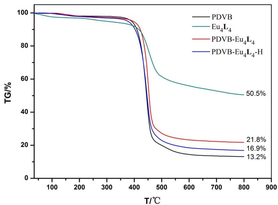
Figure S29. TGA profiles of PDVB, Eu<sub>4</sub>L<sub>4</sub>, PDVB-Eu<sub>4</sub>L<sub>4</sub>, PDVB-Eu<sub>4</sub>L<sub>4</sub>-H.
