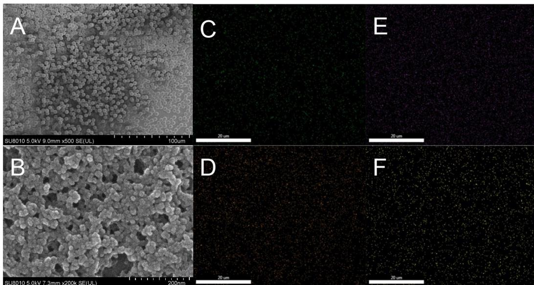
**Figure S25.** SEM images of A) PDVB and B) PDVB-Eu<sub>4</sub>L<sub>4</sub>; EDS mapping of C) N, D) S, E) F and F) Eu of PDVB-Eu<sub>4</sub>L<sub>4</sub>
