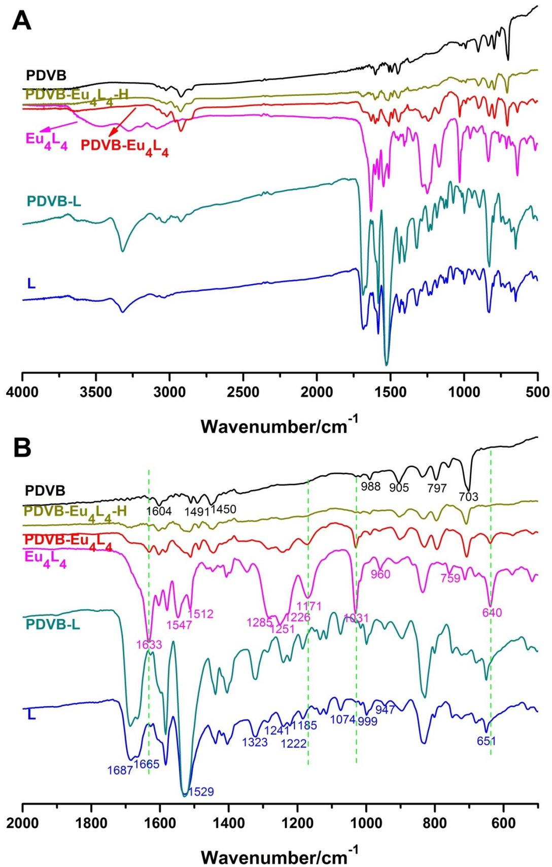
**Figure S27.** FT-IR spectra (A) and partial enlarged FT-IR spectra of L, PDVB-L, Eu<sub>4</sub>L<sub>4</sub>(OTf)<sub>12</sub>, PDVB-Eu<sub>4</sub>L<sub>4</sub>, PDVB-Eu<sub>4</sub>L<sub>4</sub>-H, and PDVB.
