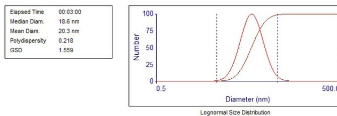
**Figure S26.** DLS size distribution by Volume of PDVB-Eu<sub>4</sub>L<sub>4</sub>.
