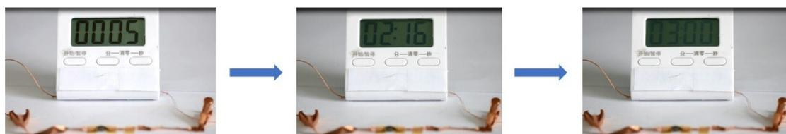
Fig. S9 Photograph of a timer powered by one ZmSC for three minutes.
