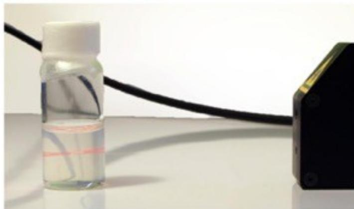
*In situ DLS remote head measurement configuration*
