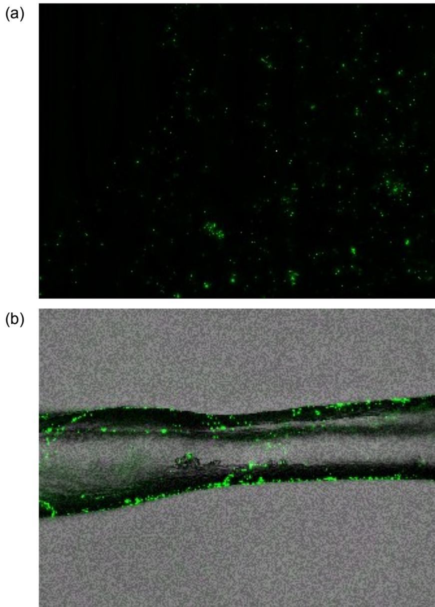
**Fig. S5** – Images of FL particles deposited on (a) RO membrane surface and (b) feed spacer. They were obtained in the feed stream at 10 cm from the entrance of ESPA2 RO element after the test. Images were taken at x400 magnification using Fluorescence Microscope BZ-X800 (KEYENCE Co., Osaka, Japan).
