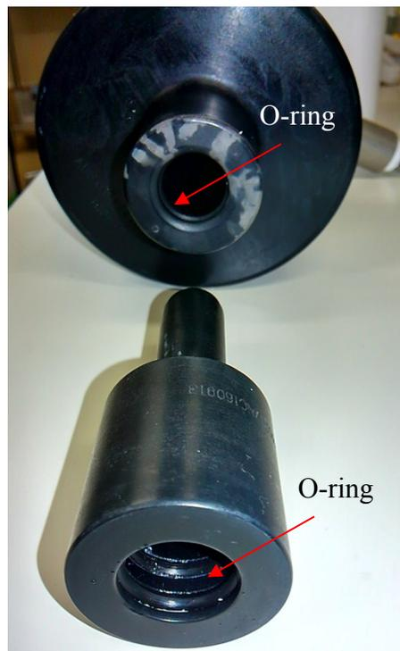
**Fig. S3** – O-rings located at the end-cap of pressure vessels.
