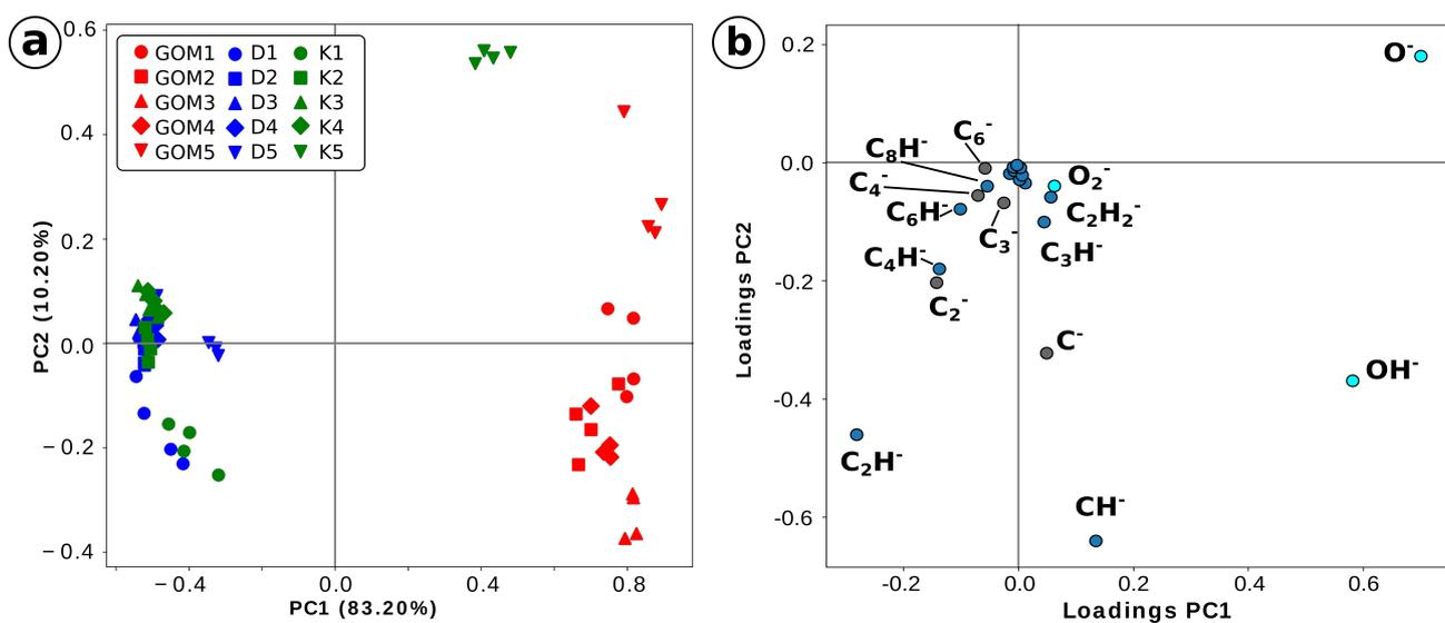
Figure S5: Score plot of PC2 vs PC1 for negative ions of soot samples obtained from gasoline engine and laboratory flames – (a). Corresponding loadings plot of the first two principal components – (b). For sample description see Table 1.
