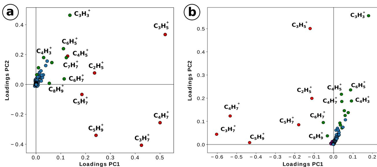
Figure S6: Loadings corresponding to the contribution of different species to PC1 and PC2 derived from mass spectra of soot samples produced by a single cylinder engine. (a) – Analysis of GOM, GOH, GEF and GEO samples, (b) – GEF and GEO samples. Aliphatic species are shown in red, fragments - in green, aromatic species - in blue and high mass high H/C compounds in purple.
