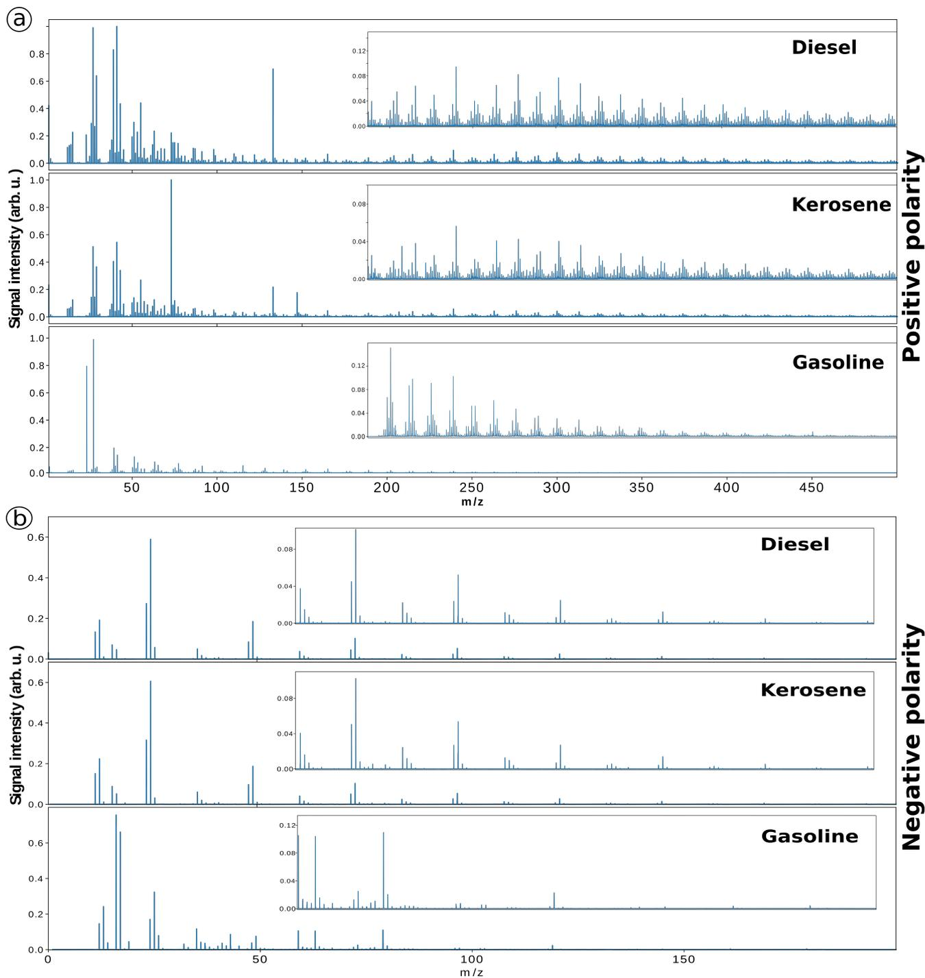
Figure S2: Comparison between mass spectra of diesel (D2), kerosene (K2) and gasoline (GOM1) soot obtained with SIMS in positive (a) and negative polarity (b). All the spectra were normalised to the highest intensity peak, for visual purpose only.
