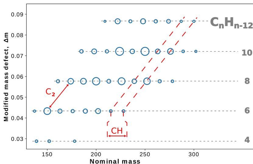
Figure S4: Kendrick mass defect plot obtained from the mass spectrum of miniCAST soot, *C2* sample. *CH* was taken as the base unit. For the ease of visualisation, only hydrocarbons are shown. The size of the data points is proportional to the corresponding peak area normalised to the total ion count.
