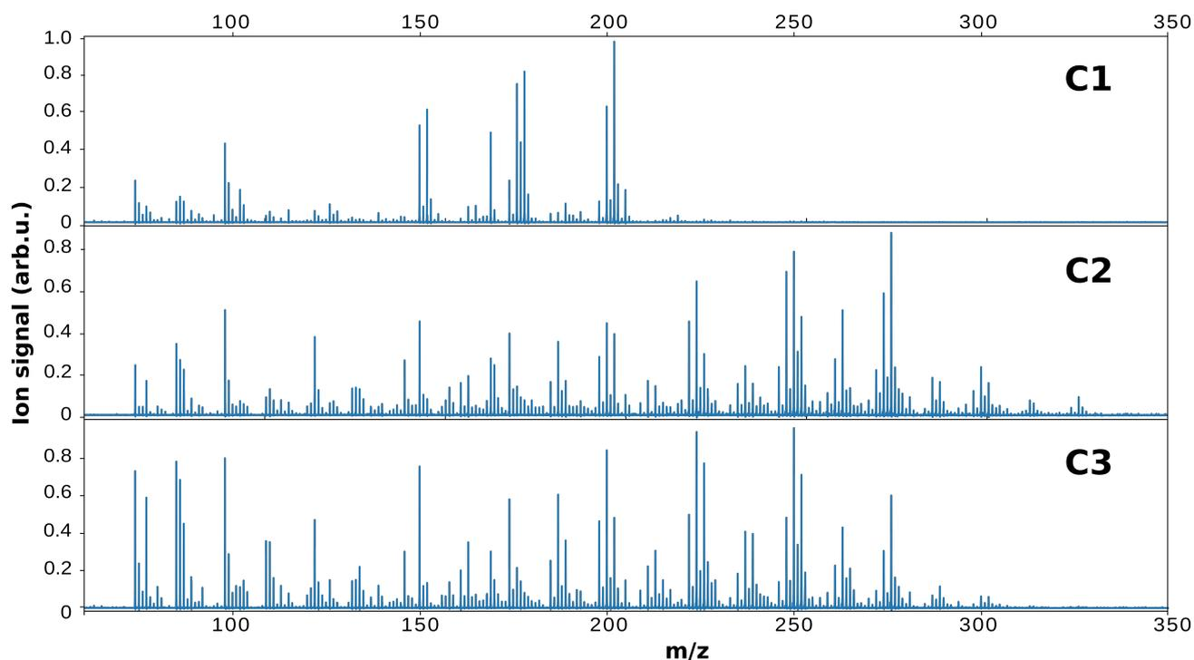
Figure S1: Comparison of mass spectra of miniCAST soot samples obtained with L2MS. All the spectra were normalised to the highest intensity peak, for visual purposes only.
