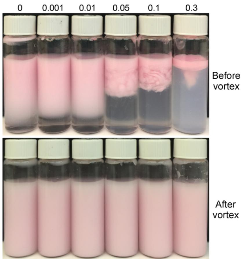
**Figure S4.** Visual appearance of samples after adding CNC-stabilized Pickering emulsions (containing Nile red in the sunflower oil) into CNF suspension of 0, 0.001, 0.01, 0.05, 0.1, or 0.3 wt% concentration. The top row includes the samples without vortexing (otherwise used to disperse the emulsions). The bottom row shows the samples after vortex homogenization. The CNF concentration is indicated on top of each sample.
