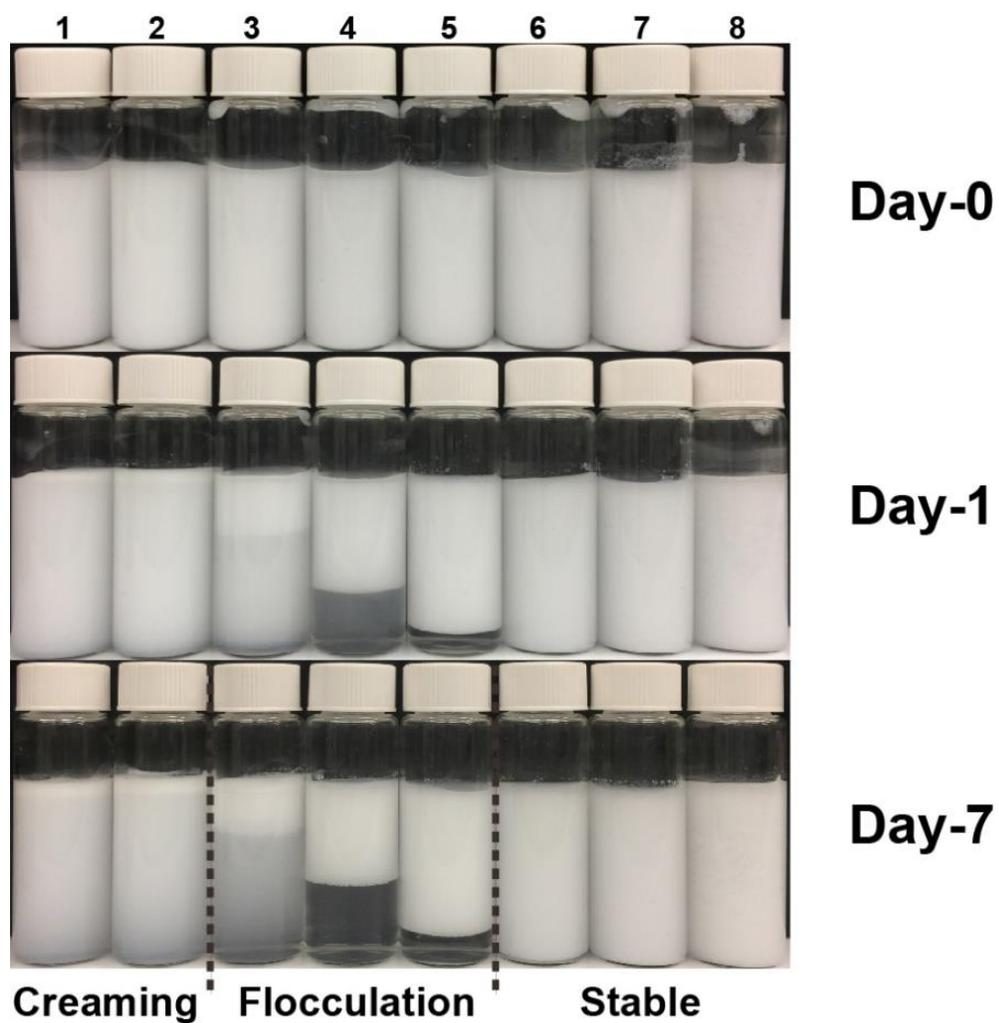
**Figure S7.** Visual appearance of Pickering emulsions (1.0 wt% sunflower oil) produced by one-step addition of nanocelluloses. The CNF concentration used was 0, 0.001, 0.01, 0.03, 0.05, 0.075, 0.1, or 0.3 wt % (corresponding to numerals 1-8, from left to right). The dotted lines are added to differentiate the three stability regimes. All the samples were stored at ambient temperature.
