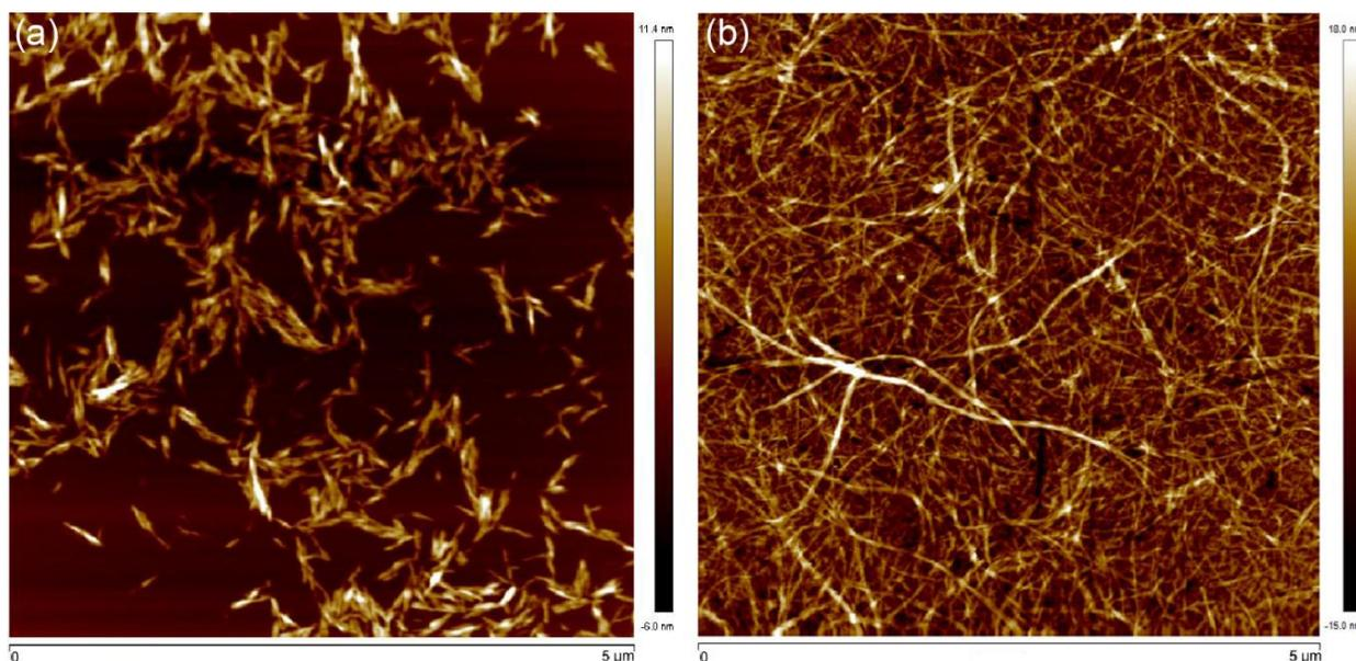
**Figure S1.** AFM height images of (a) CNCs and (b) CNF coatings. The scanning area is  $5 \mu\text{m} \times 5 \mu\text{m}$ . CNCs and CNF were coated onto mica via spin coating method.
