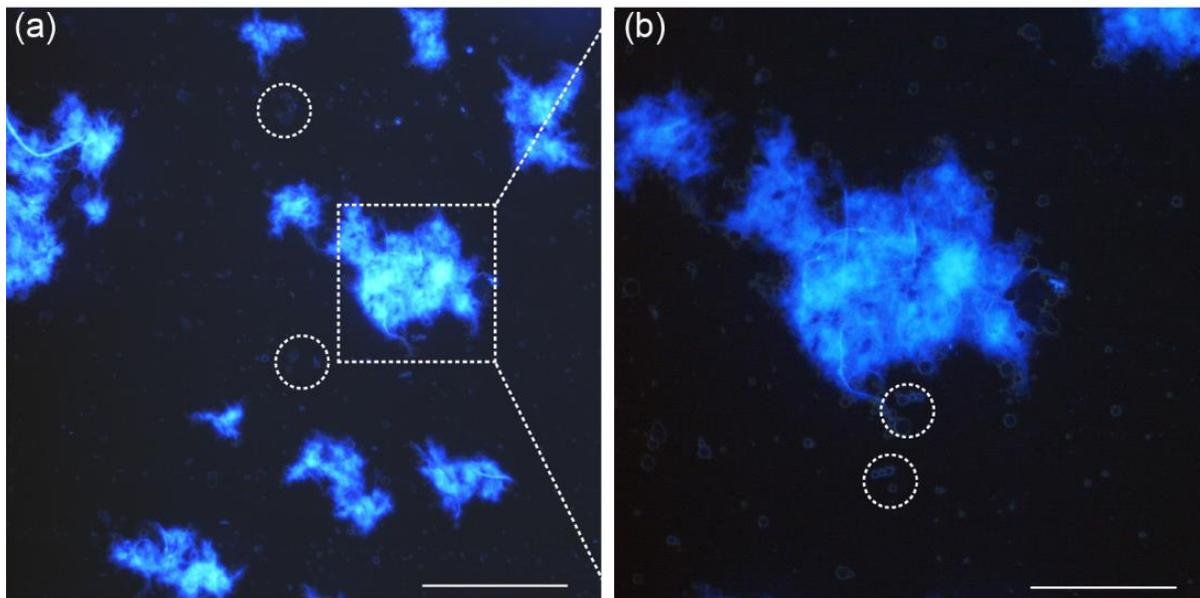
**Figure S2.** Fluorescent images of CNF flocs formed in the aqueous phase in Pickering emulsions. CNF concentration was 0.1 wt%. CNF and CNCs were dyed by Calcofluor white to blue, and oil droplets kept unstained. The dotted circle in (a) and (b) indicated the flocculated droplets. The scale bar in (a) and (b) are 100 and 50  $\mu\text{m}$ , respectively
