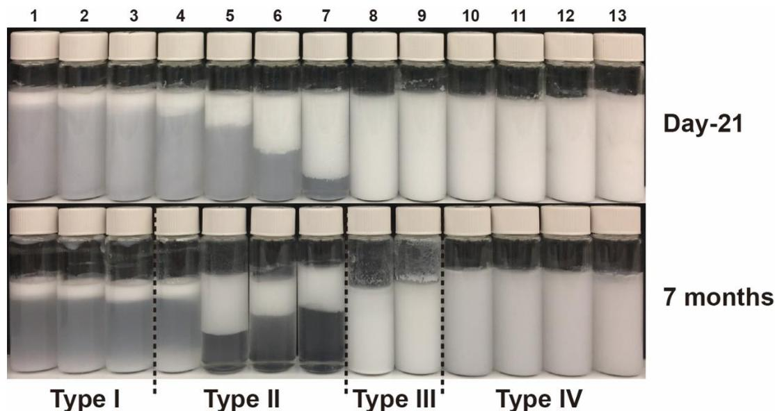
**Figure S6.** Visual appearance of CNC-stabilized Pickering emulsions containing 1.0 wt% sunflower oil with added CNF at concentrations of 0, 0.001, 0.005, 0.01, 0.03, 0.05, 0.075, 0.1, 0.2, 0.3, 0.5, 0.75, or 1.0 wt % (from left to right, numerals 1-13, respectively). The emulsion samples were stored for **21 days** and **7 months**, respectively. The dotted lines are used to differentiate the four stability regimes. All the samples were stored at ambient temperature.
