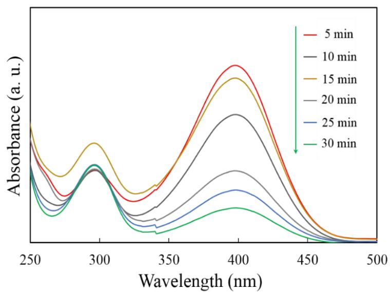
**Fig. S8.** UV-vis spectra for the catalytic reduction of nitrophenol using MRN-Pd catalysts.
