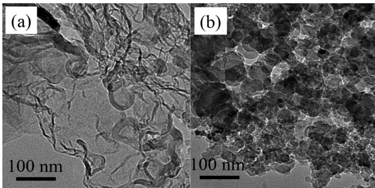
**Fig. S3.** TEM images of (a) carbon and (b) carbon-supported Pd NPs catalysts.
