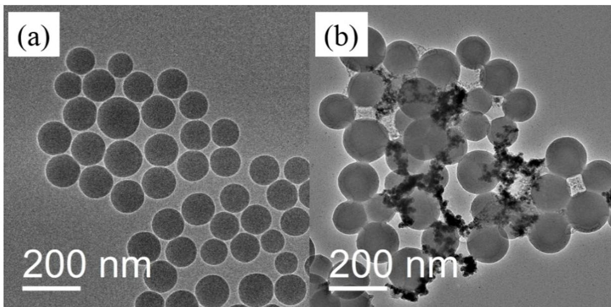
**Fig. S4.** TEM images of (a) silica NPs and (b) silica NPs supported Pd NPs catalysts.
