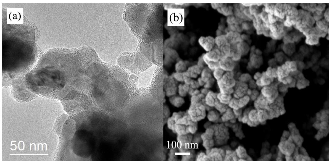
**Fig. S11.** (a) TEM image, and (b) FESEM image of the MRN–Pd catalysts after recycling.
