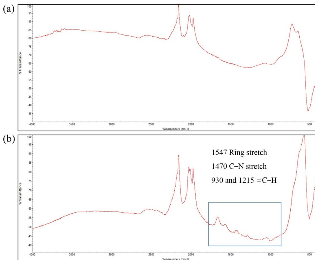
**Fig. S12.** FT-IR spectrum of (a) iron nanoparticles, and (b) the MRN-Pd catalysts after recycling.
