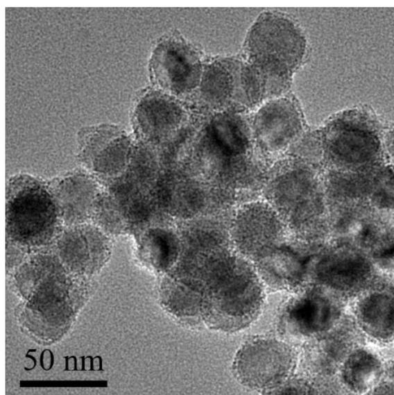
**Fig. S9.** TEM image of the iron oxide nanocomposite catalyst.
