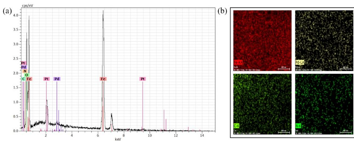
**Fig. S10.** (a) EDX spectrum, and (b) EDX map of iron, carbon, nitrogen, and Pd of the MRN–Pd catalysts after recycling.
