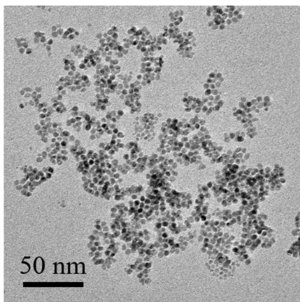
**Fig. S2.** TEM image of Pd NPs synthesized using Pluronic copolymer P123 catalysts.
