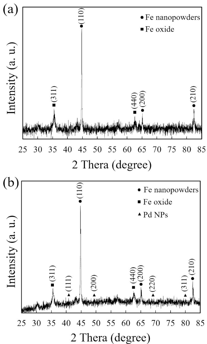
**Fig. S7.** XRD patterns of (a) iron nanoparticles and (b) MRN-Pd catalysts.
