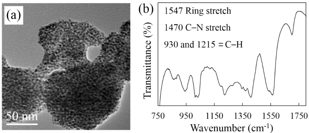
**Fig. S1.** (a) TEM image and (b) FT-IR spectrum of polypyrrole-supported Pd NPs catalysts.
