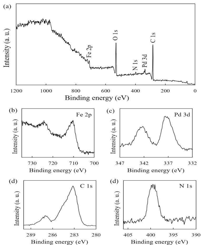
**Fig. S14.** XPS analysis (a) survey scan, (b) Fe 2p, (c) Pd 3d, (d) C 1s, and (e) N 1s for the MRN–Pd catalysts after recycling.
