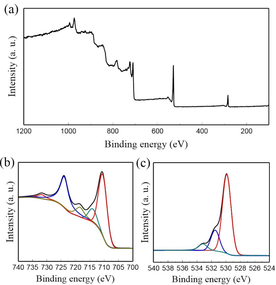
**Fig. S5.** XPS analysis of (a) survey scan, (b) Fe 2p and (c) O 1s for iron nanopowders.
