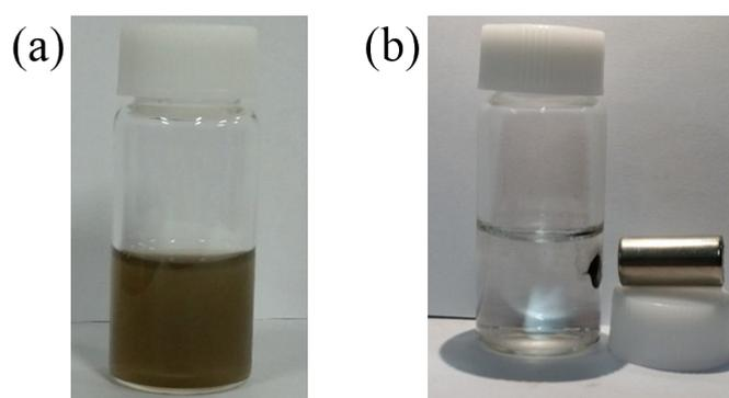
**Fig. S15.** Photographs of MRN–Pd catalysts kept under the reductive condition for five months; (a) before magnetic separation and (b) after magnetic separation.
