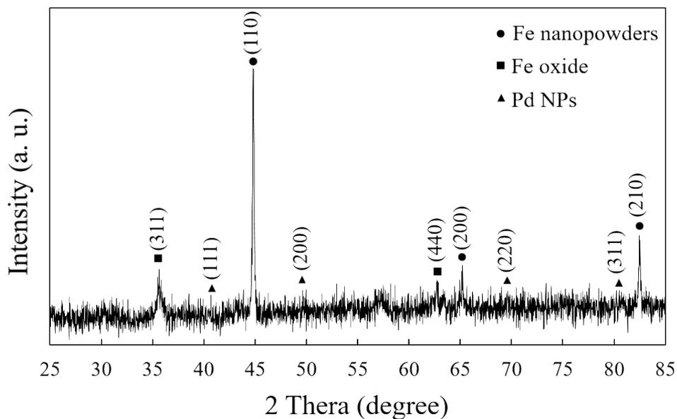
**Fig. S13.** XRD pattern of the MRN-Pd catalysts after recycling.
