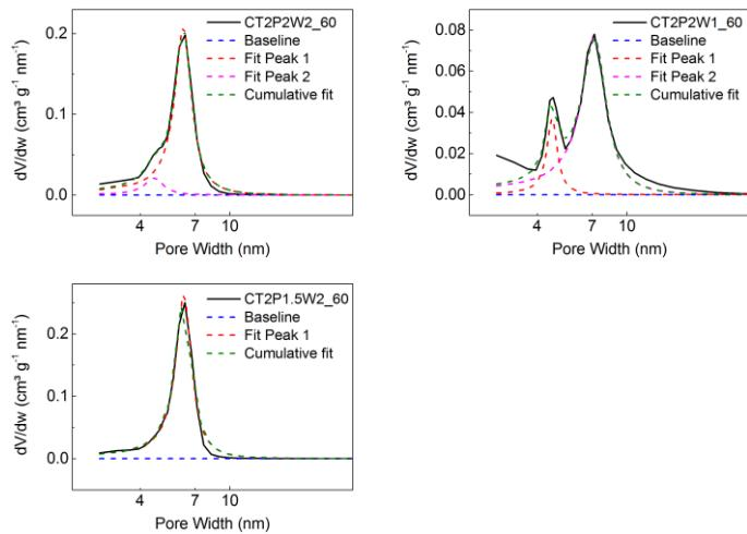
**Figure S7.** Examples of deconvolution into Lorentzian contributions performed on the PSDs of CT2P2W2\_60, CT2P2W1\_60 and CT2P1.5W2\_60 samples.
