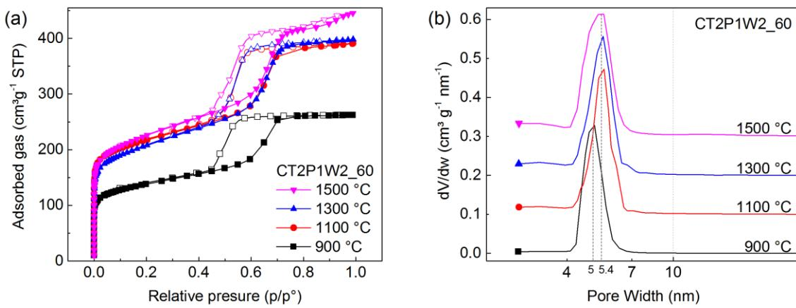
**Figure S8.** (a) N<sub>2</sub> adsorption-desorption isotherms and (b) corresponding PSDs for CT2P1W2\_60 pyrolyzed at different temperatures. For easier viewing, the PSDs curves were shifted with respect to each other by 0.1 cm<sup>3</sup> g<sup>-1</sup> nm<sup>-1</sup>.
