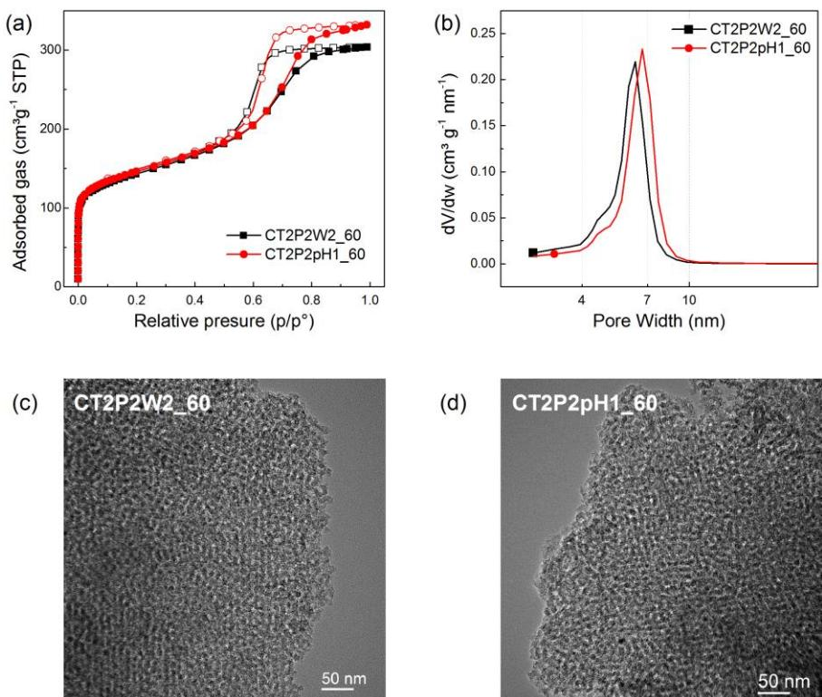
**Figure S5.** Comparison between CT2P2W2\_60 and CT2P2pH1\_60: (a) N<sub>2</sub> adsorption-desorption isotherms; (b) PSDs; and (c,d) TEM images.
