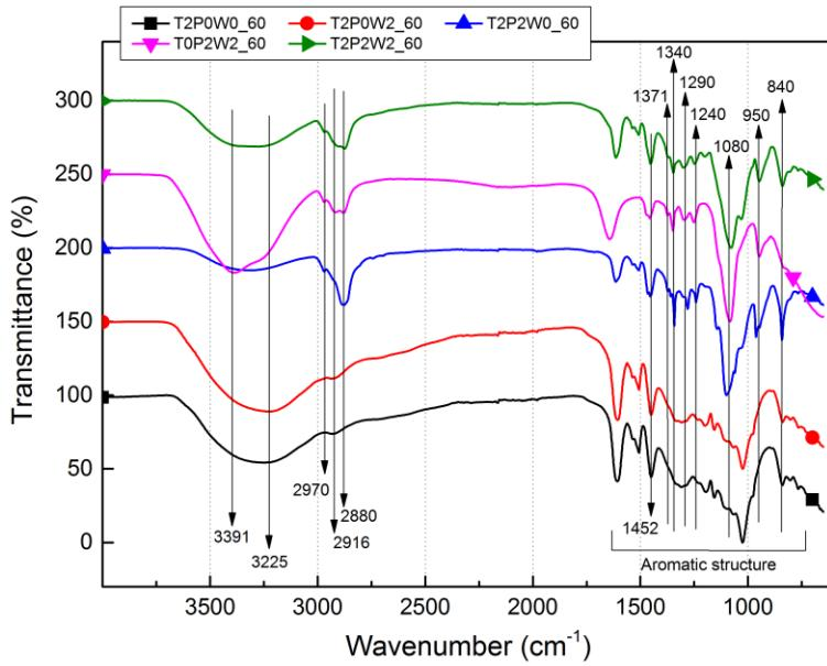
**Figure S1.** FTIR spectra of T2P2W2\_60 and reference samples. The data were normalized with respect to a common peak ( $1452\text{ cm}^{-1}$ ) and, for easier viewing, the spectra were shifted with respect to each other by 50% of transmittance.
