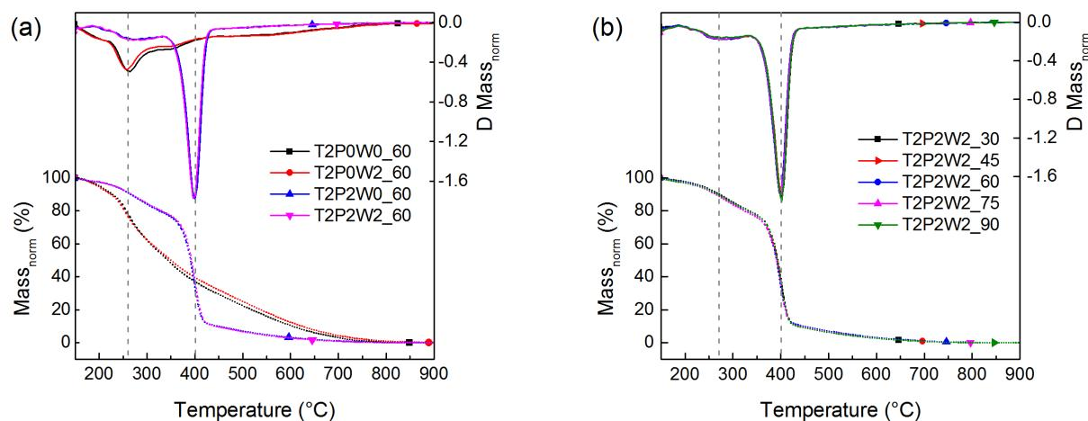
**Figure S3.** Absolute (left scale) and differential (right scale) normalized mass losses of: (a) T2P2W2\_60 and reference samples; and (b) samples T2P2W2<sub>t</sub> prepared at various milling times *t*, ranging from 30 to 90 min. The normalization was performed after removing the mass loss attributed to the evaporation of water.
