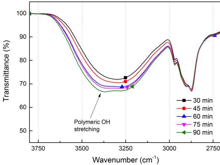
**Figure S2.** Detailed view of the FTIR spectra of samples T2P2W2<sub>t</sub> synthesized during different milling times  $t$ , ranging from 30 to 90 min. For comparison, the data were normalized with respect to a common peak ( $1452\text{ cm}^{-1}$ ).
