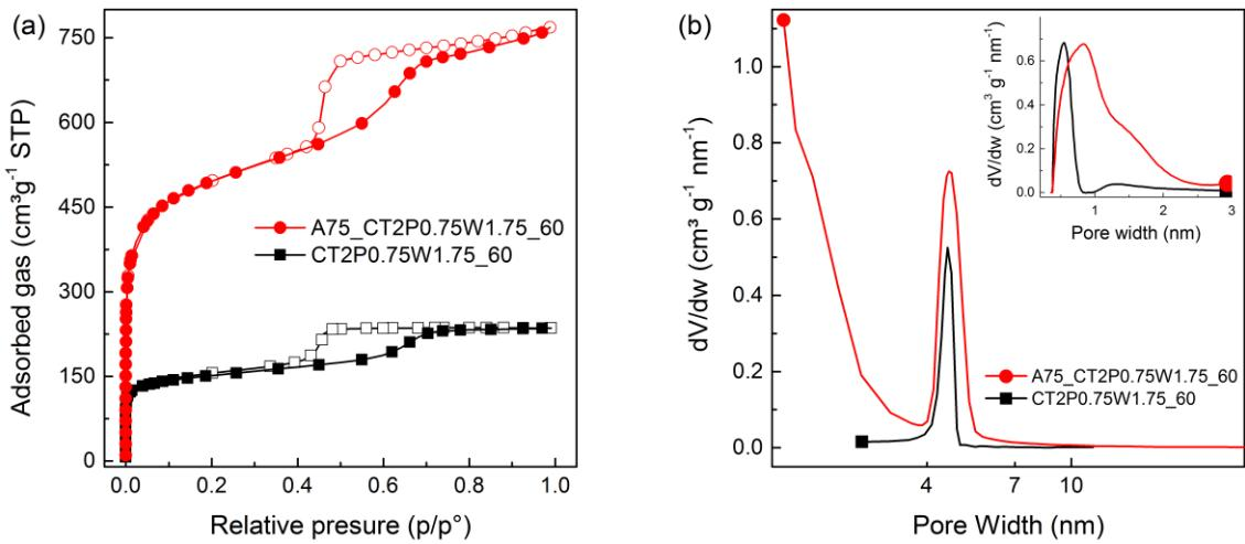
**Figure S10.** (a) N<sub>2</sub> adsorption-desorption isotherms, and (b) corresponding PSD for one OMC before (CT2P0.75W1.75\_60) and after (A75\_CT2P0.75W1.75\_60) activation with CO<sub>2</sub> for 75 min at 900°C. The inset in (b) shows the DFT PSD in the micropore range for both materials.
