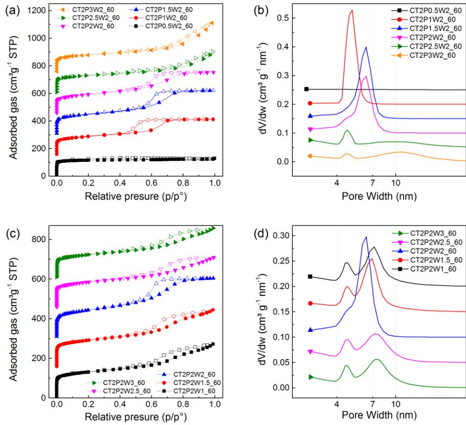
**Figure S6.** (a,c) N<sub>2</sub> adsorption-desorption isotherms and (b,d) corresponding PSDs of carbon materials synthesized using 60 min of milling and various P:W weight ratios. For easier viewing, the curves were shifted with respect to each other by 150 cm<sup>3</sup> g<sup>-1</sup> STP for isotherms and by 0.05 cm<sup>3</sup> g<sup>-1</sup> nm<sup>-1</sup> for PSDs.
