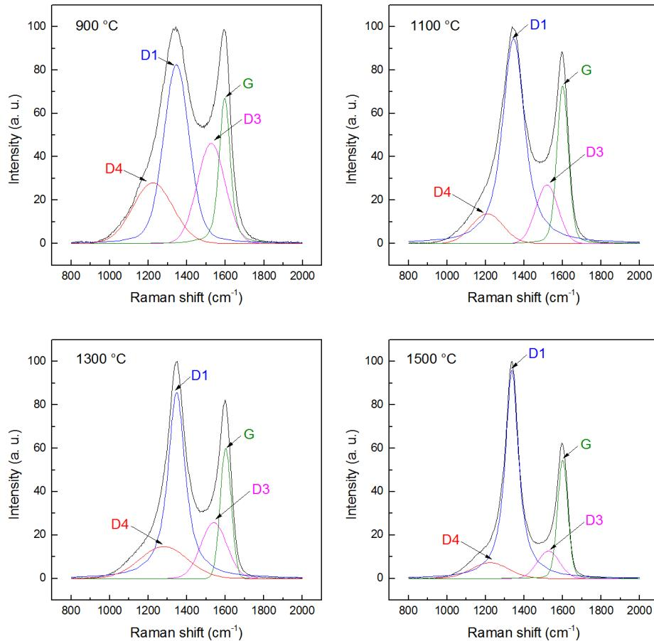
**Figure S9.** Raman spectra of CT2P1W2\_60 pyrolyzed at different temperatures, and corresponding D<sub>1</sub>, D<sub>3</sub>, D<sub>4</sub> and G bands.
