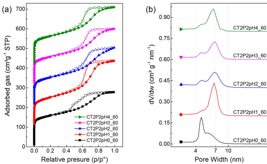
**Figure S4.** (a) N<sub>2</sub> adsorption-desorption isotherms and (b) corresponding PSDs of carbon materials CT2P2pHx\_60, synthesized by using aqueous solutions of HCl at pH ranging from 0 to 4 instead of water, and a milling time of 60 min. For easier viewing, the curves were shifted with respect to each other by 105 cm<sup>3</sup> g<sup>-1</sup> STP for isotherms and by 0.2 cm<sup>3</sup> g<sup>-1</sup> nm<sup>-1</sup> for PSDs.
