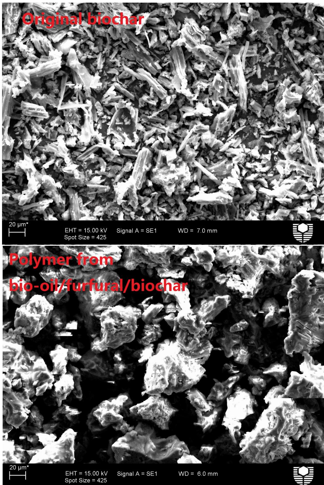
**Figure S4** SEM images of biochar and the polymer produced from bio-oil/furfural/biochar.
