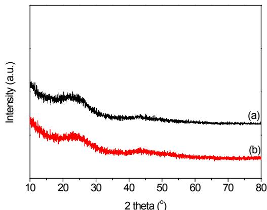
Fig. S7 XRD patterns of (a) fresh  $\text{Co}_1\text{Zn}_{99}\text{-ZIF-800-H}_2$  and (b) 4 times reused  $\text{Co}_1\text{Zn}_{99}\text{-ZIF-800-H}_2$ .
