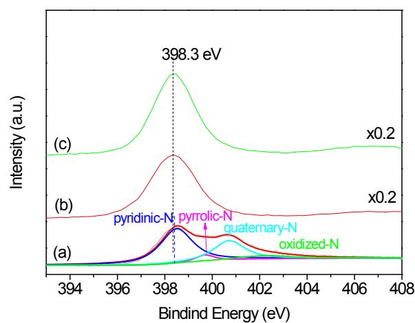
Fig. S5 N1s XPS spectra of (a)  $\text{Co}_1\text{Zn}_{99}\text{-ZIF-800-H}_2$ , (b)  $\text{Co}_1\text{Zn}_{99}\text{-ZIF}$  and (c)  $\text{Co}_5\text{Zn}_{95}\text{-ZIF}$ .
