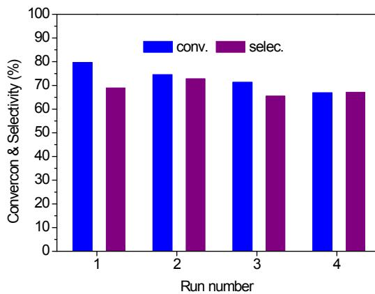
Fig. S6 Recycle of  $\text{Co}_1\text{Zn}_{99}\text{-ZIF-800-H}_2$  for selective oxidation of EB with  $\text{O}_2$  at high conversion.
