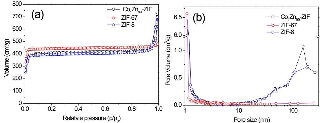
Fig. S2 (a) Nitrogen sorption isotherms and (b) pore size distribution of Co<sub>x</sub>Zn<sub>100-x</sub>-ZIF materials.
