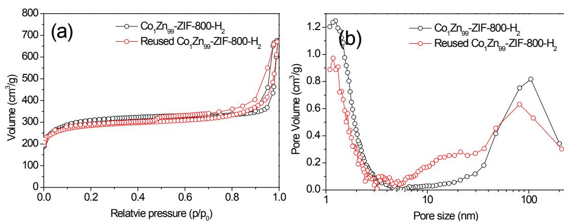
Fig. S8 (a) Nitrogen sorption isotherms and (b) pore size distribution of fresh and 4 times reused  $\text{Co}_1\text{Zn}_{99}\text{-ZIF-800-H}_2$ .
