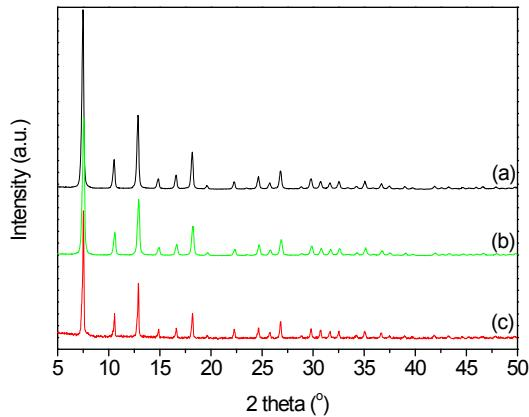
Fig. S1 XRD patterns of (a) ZIF-8, (b) Co<sub>1</sub>Zn<sub>99</sub>-ZIF and (c) ZIF-67.
