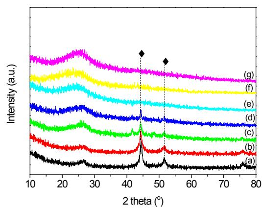
Fig. S4 XRD patterns of (a) ZIF-67-800-Ar, (b)  $\text{Co}_{50}\text{Zn}_{50}\text{-ZIF-800-Ar}$ , (c)  $\text{Co}_{10}\text{Zn}_{90}\text{-ZIF-800-Ar}$ , (d)  $\text{Co}_5\text{Zn}_{95}\text{-ZIF-800-Ar}$ , (e)  $\text{Co}_{2.5}\text{Zn}_{97.5}\text{-ZIF-800-Ar}$ , (f)  $\text{Co}_1\text{Zn}_{99}\text{-ZIF-800-Ar}$  and (g)  $\text{Co}_{0.2}\text{Zn}_{99.8}\text{-ZIF-800-Ar}$ .
