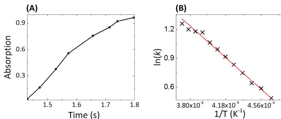
Fig. ESI 2. Determination of the order of reaction by analysing the slopes using the parameters from Arrhenius equation ( $E_a$ ,  $k$ ,  $T$ ,  $t$ ). (A) Abs. vs time. data for CaF formation at 2,400 °C and (B) Arrhenius plot  $\ln(k)$  vs  $1/T$  for CaF in a range of temperatures from 1,900 °C to 2,400 °C.
