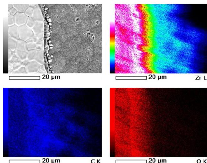
Fig. ESI 7. SEM micrograph of Zr-nano coated graphite and the corresponding EDX elemental mapping for Zr, C, and O taken at 5 kV. A ZrO atomic ratio of 1:2 was quantified by EDX standardless analysis.
