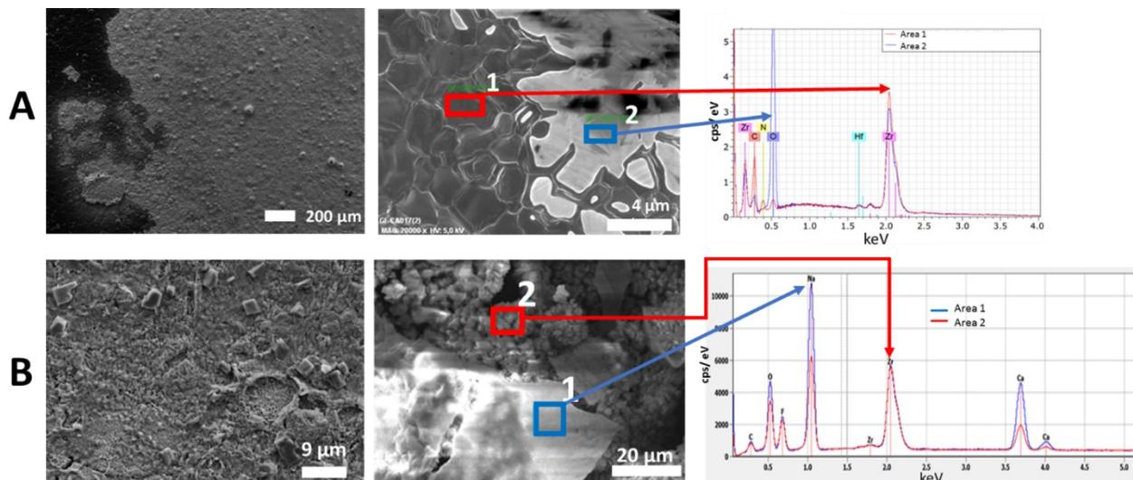
Fig. ESI 3. (A) SEM micrographs of a zirconium-coated graphite furnace P1 (overview and at higher magnification) and their corresponding EDX spectra at 5 kV for two apparently different areas. (B) SEM micrographs of the transition state P2 (overview and zoom and higher magnification) with their corresponding EDX spectra at 20 kV for two apparently different areas.
