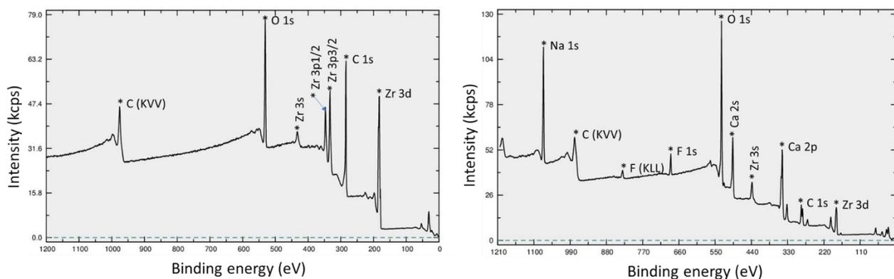
Fig. ESI 5. (Left) Wide scan XPS of a zirconium-coated platform P1. (Right) Wide scan XPS of the transition state P2: a zirconium coated platform after pyrolysis of NaF and  $\text{Ca}(\text{NO}_3)_2$  at  $900^\circ\text{C}$ .
