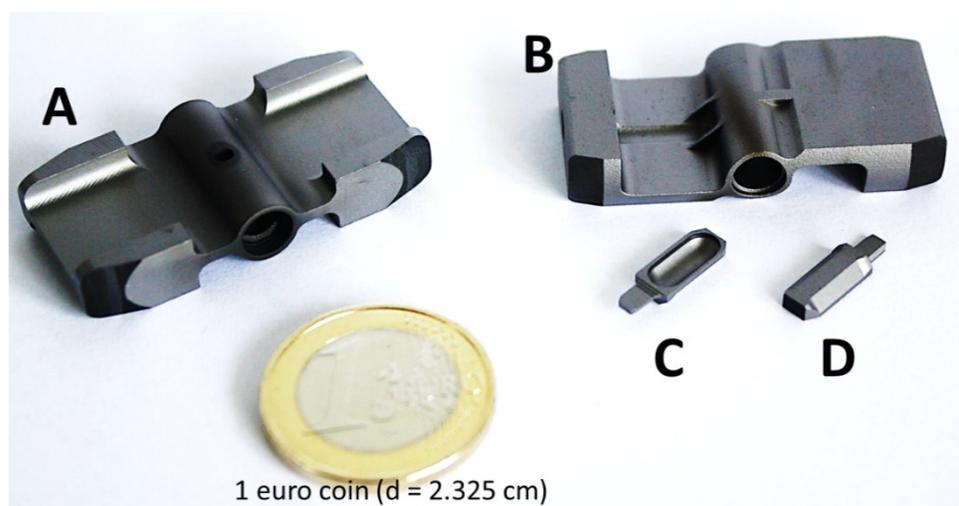
Fig. ESI 1. (A) Graphite tube with the incorporated platform used in HR-CS-AAS. (B) Graphite tube without platform used in solid sampling AAS. (C) Graphite platform for solid sampling, this platform is inserted in (B) with the sample. (D) backside of graphite platform for solid sampling (area 0.2 mm x 1 mm).
