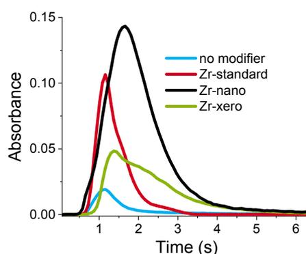
Fig. ESI 8. The effect on the preparation of ZrO modified graphite platforms on the analytical signal of CaF in HR-CS-MAS.
