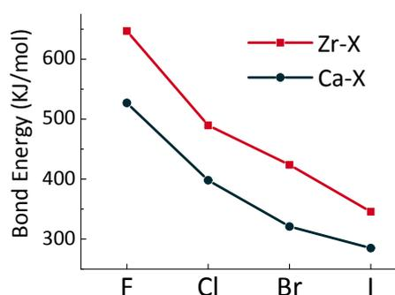
Fig. ESI 9. Tendency of bond strength for zirconium and calcium halogenides.<sup>1</sup>
