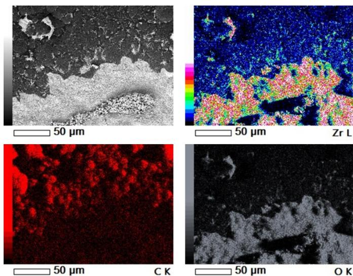
Fig. ESI 4. SEM micrograph of Zr coated graphite P1 and the corresponding EDX elemental mapping for Zr, C, and O taken at 5 kV. A ZrO atomic ratio of 1:2 was quantified by EDX standardless analysis.
