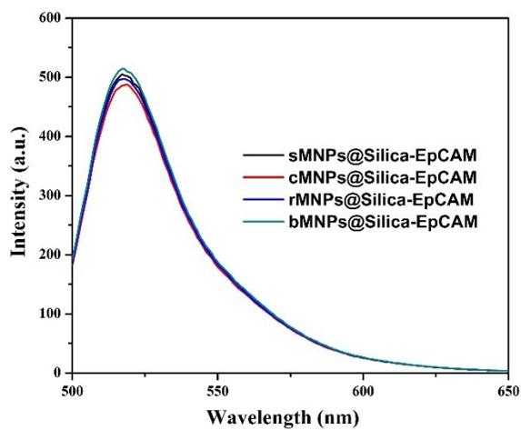
**Figure S2.** Fluorescent spectra of MNPs@Silica-EpCAM with different shapes at a same particle concentration of 100  $\mu\text{g/mL}$ .
