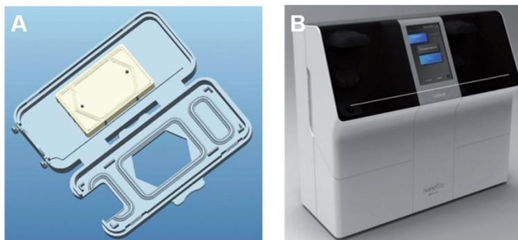
**Figure S5.** Our self-developed immunomagnetic microchip for CTCs screening. (A) Schematic drawing of the embedded microfluidic cartridge. (B) Photograph image of our CellRich™ system.
