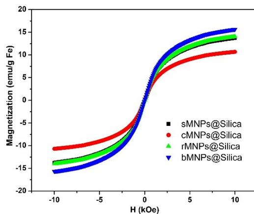
**Figure S1.** Hysteresis curves of MNPs@Silica core-shell nanoparticles with different shapes recorded at 300 K.
