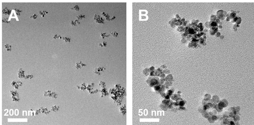
**Figure S6.** TEM images of Veridex Ferrofluid at different magnifications.
