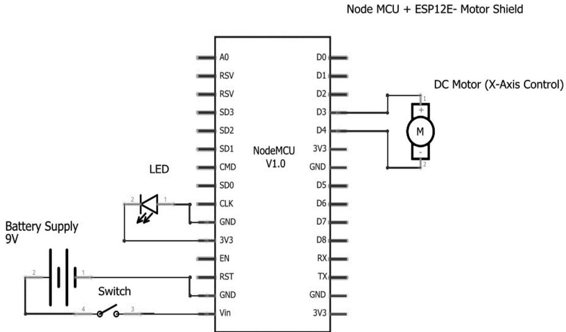
**Figure S1. Circuit diagram of the electrical enclosure of the optical system.** Wireless communication between the smartphone and the optical attachment was achieved by configuring the Single-board microcontroller (NodeMCU) as an http web server. The system includes a DC motor for automation, a LED for illumination, a 9 V battery for power source, and a switch for control purposes. All components are connected to the NodeMCU.
