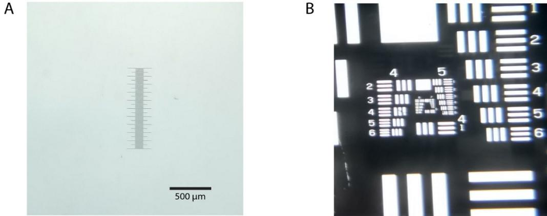
**Figure S2. Image of micrometer scale and 1951 US Air Force (USAF) resolution test chart recorded with the smartphone system.** (A) The spacing between the divisions of the stage micrometer (Omax, B00FG89F0M) is 10 μm. The dimensions of the image shown here are 642 × 642 pixels. One micron is represented by 0.226 pixels. (B) Resolution of the reported smartphone-based optical imaging system was 7 μm.
