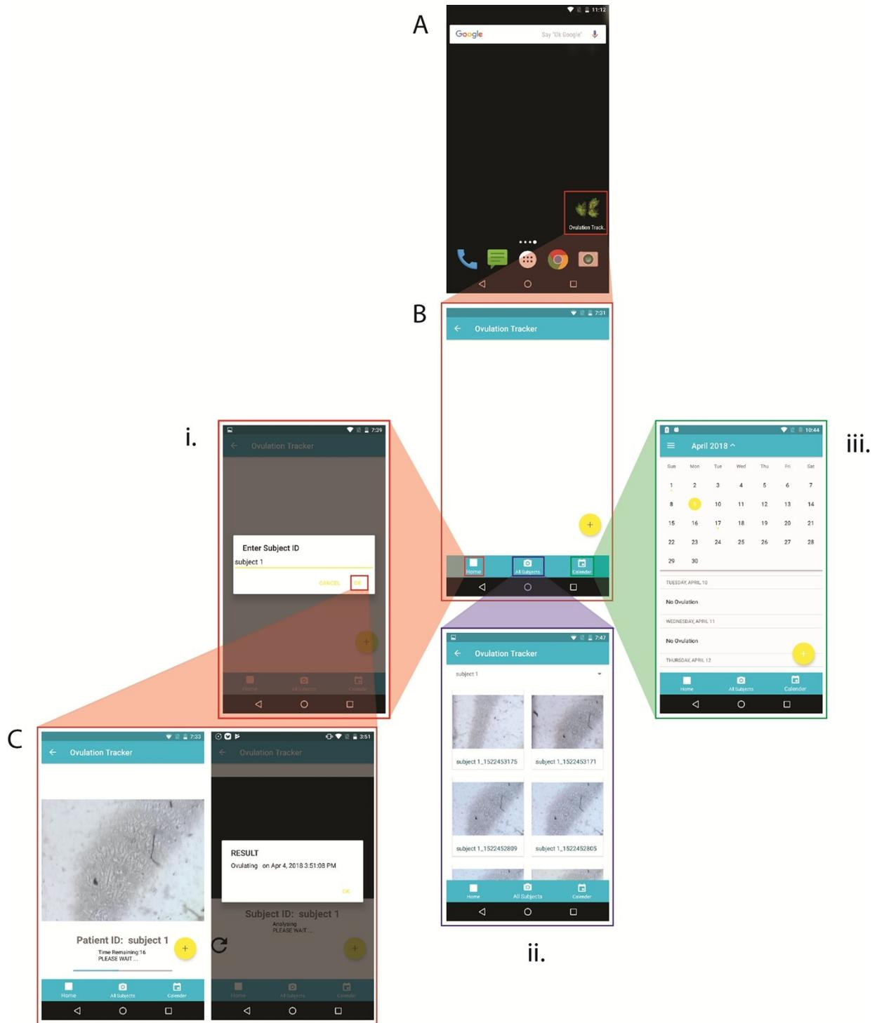
**Figure S3. Smartphone application user interface.** These figures show the process flow of the android application developed for image processing and ovulation detection. (A) The smartphone
