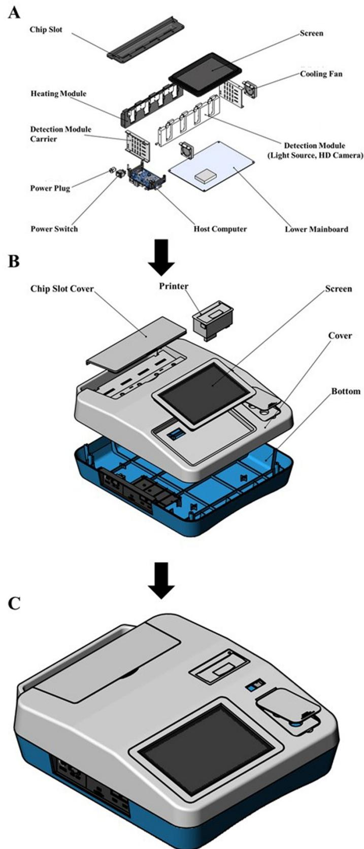
Fig. S1. The schematic drawing of the measurement instrument, A represent internal structure of the instrument, B represent external structure of the instrument, and C represent the detection instrument.
