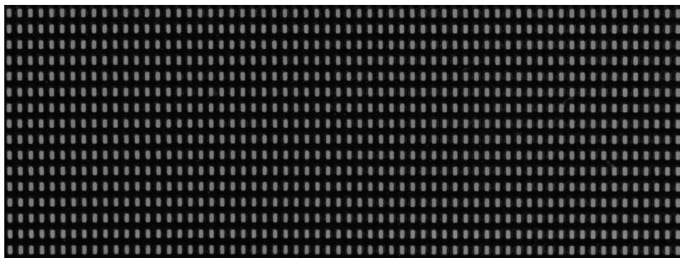
Figure S1. Fluorescent image of SD chip after sample digitization using buffer containing calcein, showing the completeness of microwell filling using the modified SD chip.
