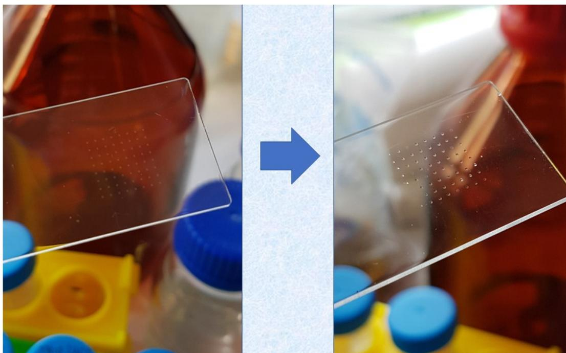
**Figure S5.** YF-Q11 hydrogel spotted microarray slide. Dry spots (left panel) instantaneously rehydrates upon immersion in water (right panel).
