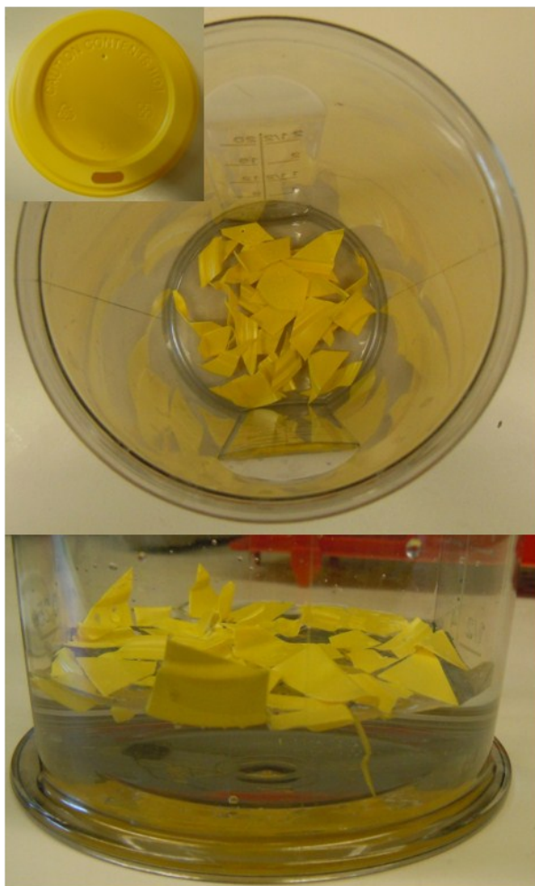
Figure S2. Production of particles using a coffee cup lid as starting material. a. showing the pieces in water from top and side view. Inset into the top view picture is a picture of the intact coffee lid. b. showing a top and side view of the mixture after 5 min treatment with the immersion blender.
