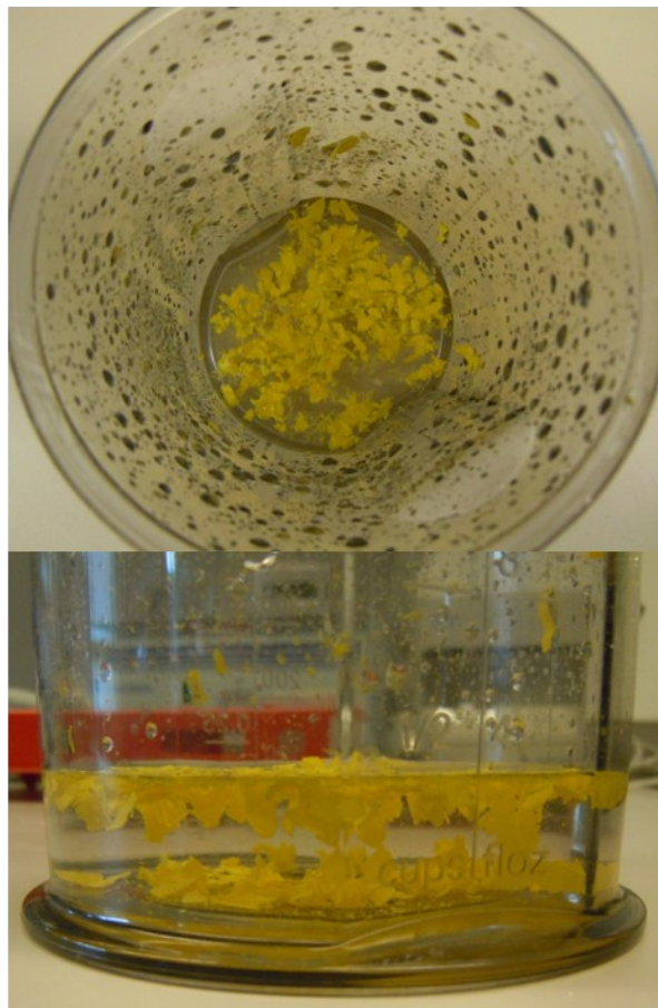
Figure S2. Production of particles using a coffee cup lid as starting material. a. showing the pieces in water from top and side view. Inset into the top view picture is a picture of the intact coffee lid. b. showing a top and side view of the mixture after 5 min treatment with the immersion blender.
