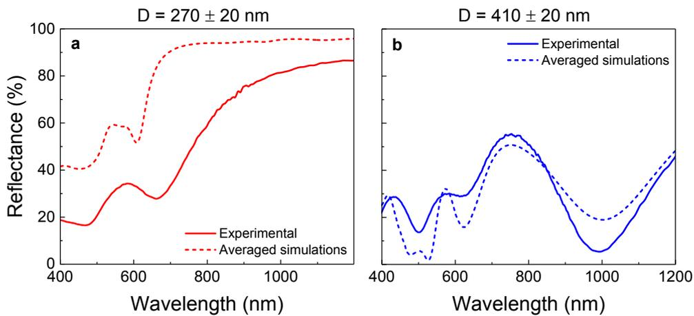
**Fig. S4** Measurements (solid lines) and averaged simulations (dashed lines) of reflectance for Au-Ni-Au films embedded with particles of diameter  $D$ . The simulated curves correspond to an average over (a) the error range of  $D$  and (b) angles of incidence ranging from 0 to 10°.
