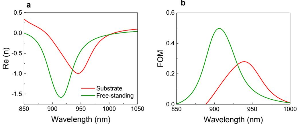
**Fig. S8** (a) Real part of the effective refractive index and (b) figure of merit of the double fishnet metamaterial with and without substrate.
