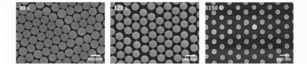
**Fig. S2.** SEM images of non-close-packed monolayers of PS beads after reduction of their diameter by oxygen plasma for different etching times of 90, 120 and 150 s.
