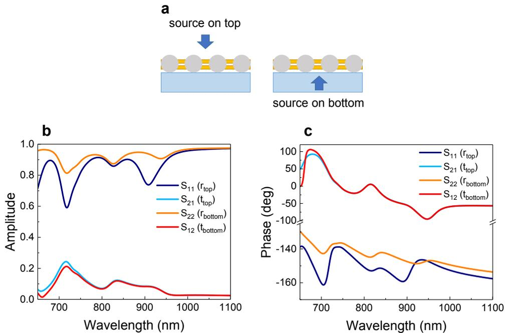
**Fig. S6** (a) Schematic illustrations of the two simulations performed for the retrieval. (b) Amplitudes and (c) phases of the simulated S-parameters for the metamaterial exhibiting -1 refractive index,
