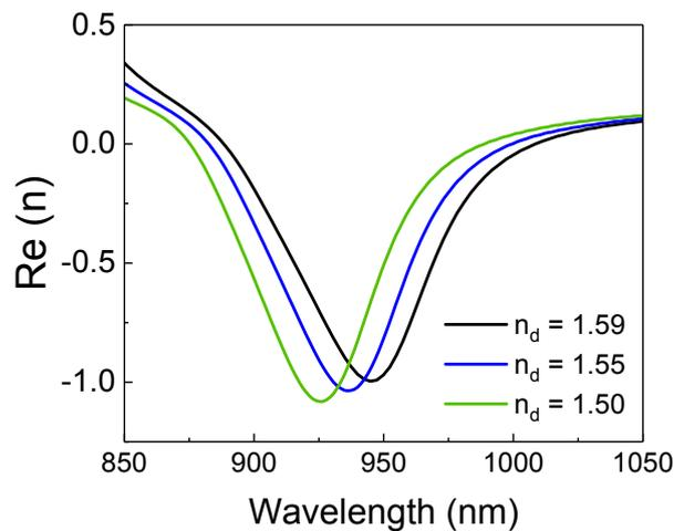
**Fig. S1.** Real part of the effective refractive index of the metamaterial when varying the dielectric index of the spheres. The main features of the structure are two 50 nm thick Au layers separated by a 25 nm wide air gap and perforated by 200 nm large spheres, with a lattice parameter of 480 nm.
