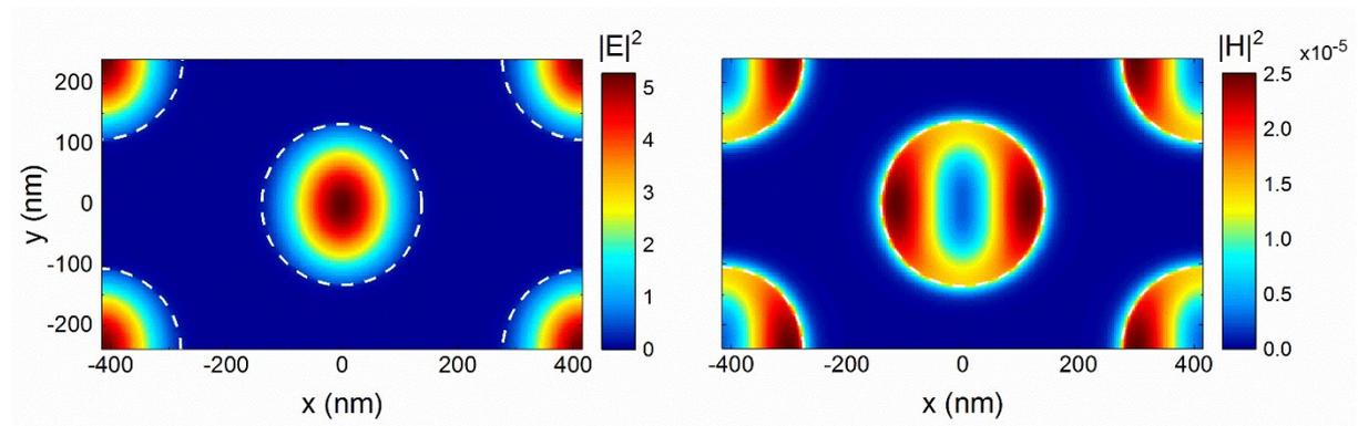
**Fig. S5.** Electric and magnetic field intensities of the multilayered nanostructure at the nickel middle plane for the minimum of reflectance ( $\lambda = 616$  nm). The unit cell consisted of  $L = 480$  nm,  $D = 270$  nm, 50 nm thick Au layers and 70 nm Ni spacer.
