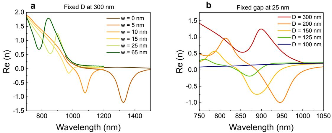
**Fig. S12** Numerical simulations of the real part of the effective refractive index when varying (a) the air gap width between the gold layers of the spheres and (b) the diameter of the beads.
