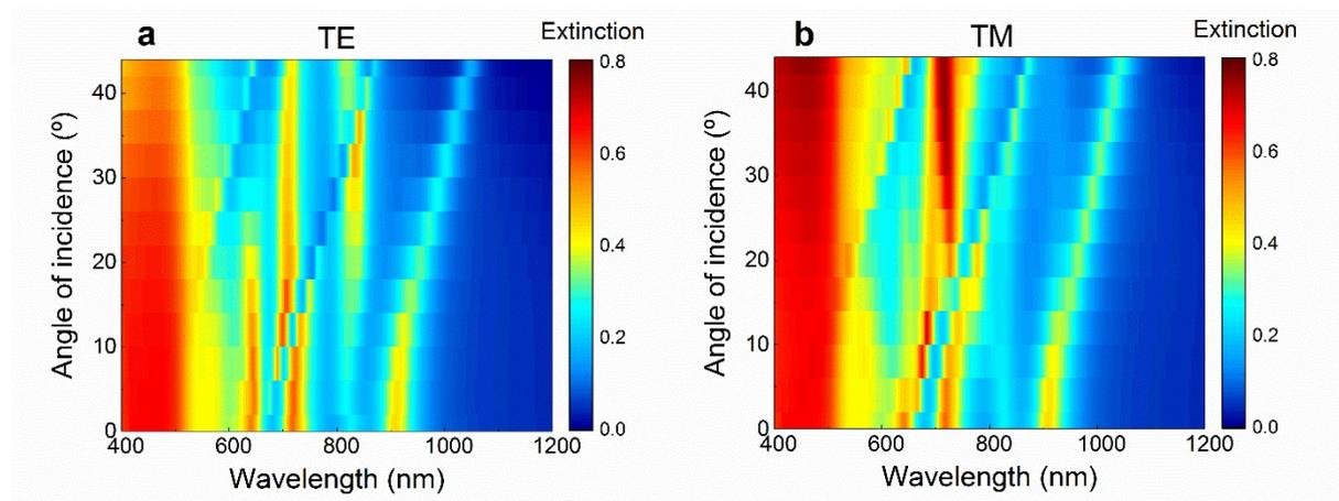
**Fig. S10** Extinction versus wavelength and angle of incidence of the structure presenting a -1 refractive index for (a) TE and (b) TM polarizations.
