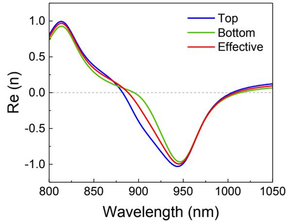
**Fig. S7** Real part of the effective refractive indices when light comes from the top, from the substrate and the correction made considering both results.
