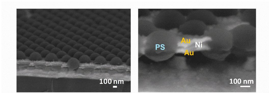
**Fig. S3.** SEM images of a multilayered nanostructure composed by etched spheres of  $D = 340$  nm, two 50 nm thick Au layers symmetrically placed regarding the monolayer axis and a 70 nm thick Ni spacer.
