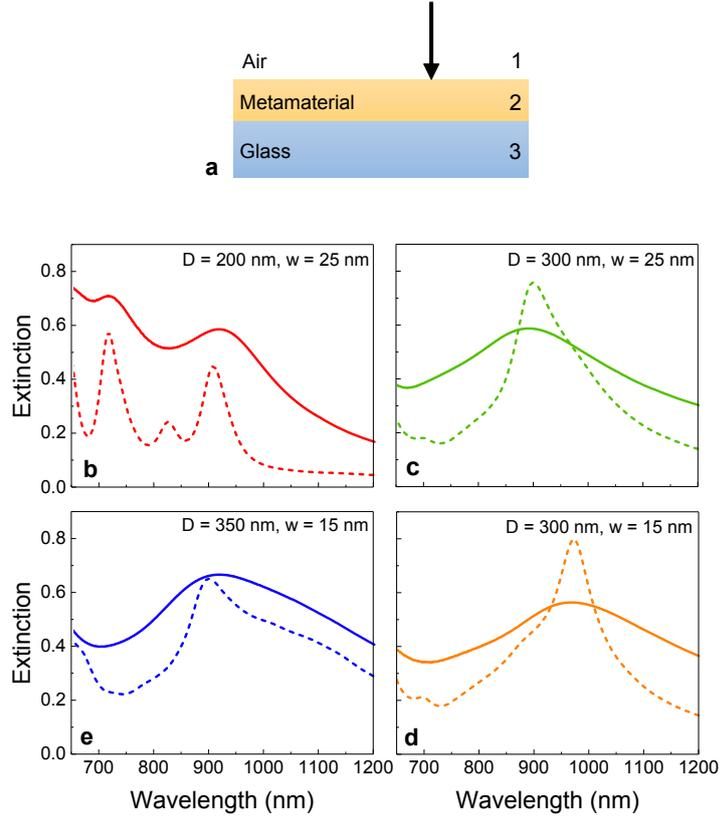
**Fig. S11** (a) Schematic illustration of the effective system adopted for Fresnel modelling. Experimental (solid lines) and calculated (dashed lines) extinction spectra of samples with (a)  $D = 200$  and  $w = 25$  nm, (b)  $D = 300$  nm and  $w = 25$  nm, (c)  $D = 300$  nm and  $w = 15$  nm and (d)  $D = 350$  nm and  $w = 15$  nm.
