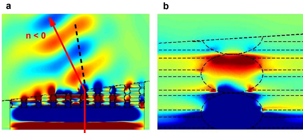
**Fig. S9** Simulated electromagnetic behaviour of a prism composed of several layers of our fishnet metamaterial. (a) Electric field propagation at the wavelength of resonance showing negative refraction. (b) Magnified plot of the electric field distribution, where negative phase propagation occurs (see supplementary movies).
