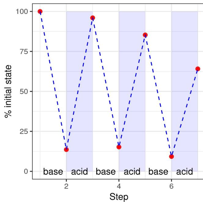
**Figure S9:** Reversibility of fluorescence quenching of **CPI** (0.2 mM) upon pH changes (acid, 3-4) or basic (*ca* 8).
