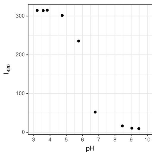
**Figure S1:** Evolution of fluorescence emission at 420 nm upon addition of NaOH (0.1 M) to a solution of **CP1** (0.2 mM) in milliQ water.  $\lambda_{\text{ex}} = 340 \text{ nm}$
