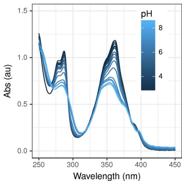
**Figure S4:** Absorbance changes after addition of small aliquots of NaOH (0.1 M) to a **CP1** (0.4 mM) in milliQ water.
