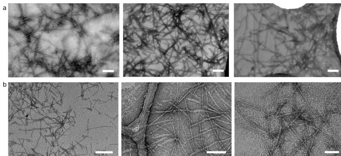
**Figure S8:** Micrographs of CP1 (0.02 % w/w) after dilution of the gel (pH *ca* 8). Samples were stained with uranyl acetate. a) STEM images. Scale bar is 100 nm; b) TEM images. Scale bars are 200 (left), 50 (center) and 50 nm (right).
