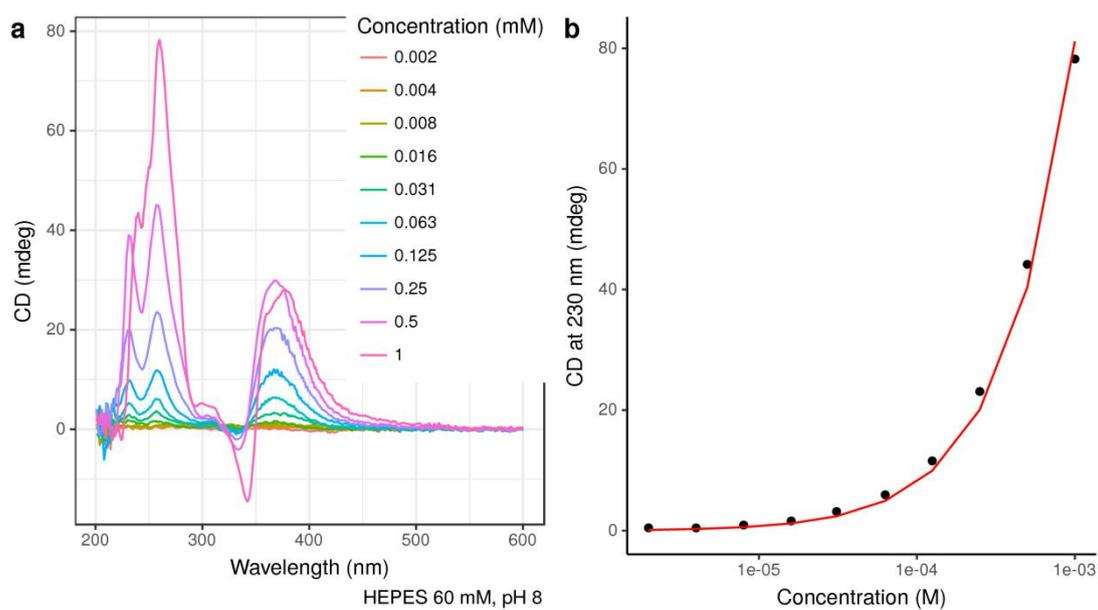
**Figure S5:** a) Circular dichroism of **CP1** at different concentrations in HEPES (60 mM) at pH 8; b) fitting to a homodimerization model. A  $K_a$  of  $4 \times 10^6 \text{ M}^{-1}$  and a molar ellipticity constant of  $820 \text{ deg cm}^{-2} \text{ dmol}^{-1}$  was obtained.
