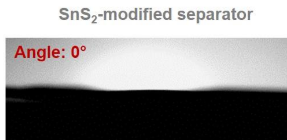
Fig. S2. Dynamic electrolyte contact angle measurements for pristine and SnS 2 -modified separator respectively.
