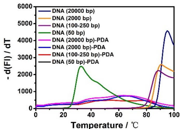
**Fig. S13** Melting curves of four different DNA and DNA templated nanoplatelets/sheets.
