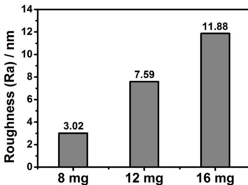
**Fig. S8** Surface roughness of DNA-PDA nanosheets synthesized at varying hsDNA/dopamine weight ratios of 1:1, 1.5:1, and 2:1, as obtained by the corresponding AFM images.
