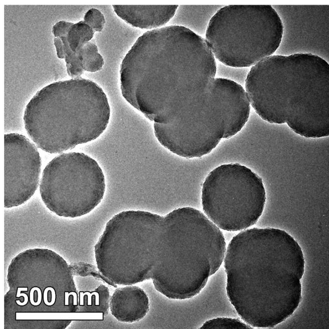
**Fig. S3** TEM images of the control polydopamine nanoparticles without the addition of DNA in the synthetic process.
