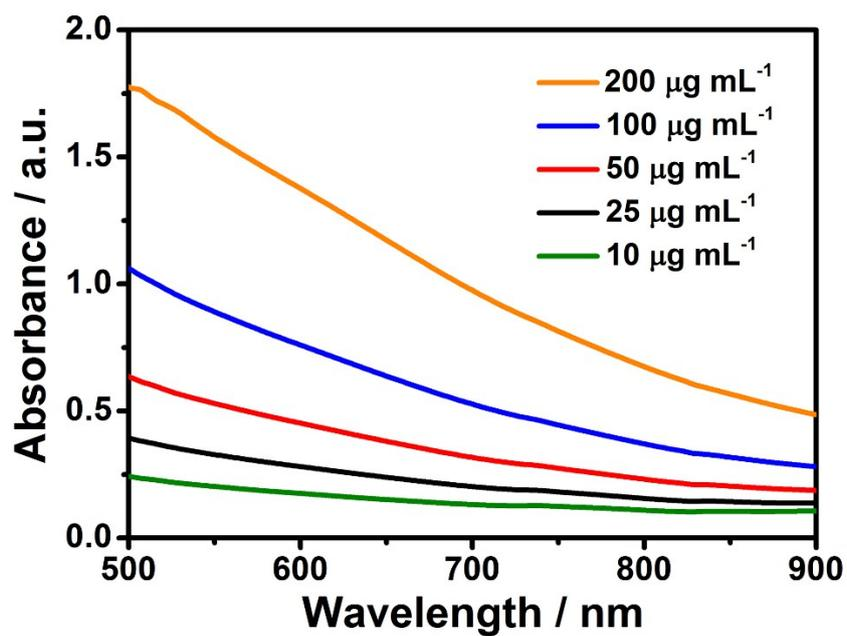
**Fig. S17** Absorbance spectra of suspensions of DNA-PDA nanosheets at varying concentrations (200, 100, 50, 25 and 10  $\mu\text{g mL}^{-1}$ ). The nanosheets were synthesized at DNA/dopamine weight ratio of 1.5:1.
