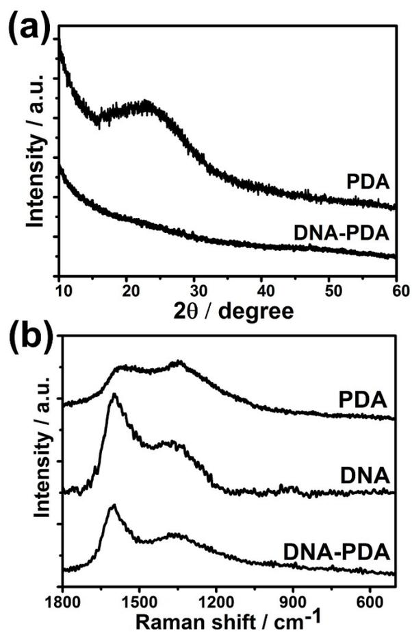
**Fig. S2** (a) X-ray diffraction spectra. (b) Raman spectra of DNA, PDA nanoparticles, and DNA-PDA nanoplatelets.
