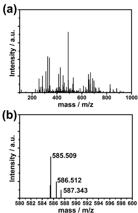
**Fig. S6** FT-ICRMS (a) and segmental magnified spectra (b) ( $m/z$  580-600) of DNA-PDA nanoplatelets synthesized at DNA/dopamine weight ratio of 0.025:1.
