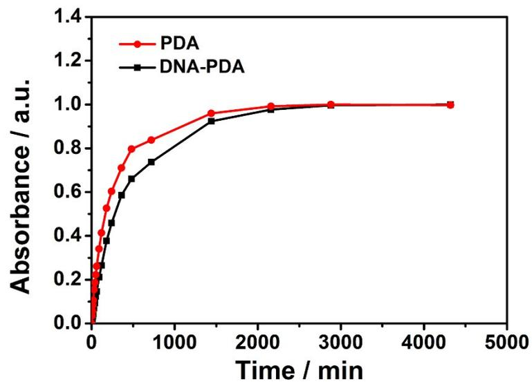
**Fig. S5** In situ evolution of PDA polymerization under different conditions by monitoring the absorbance of the synthesis solution at 400 nm over time.
