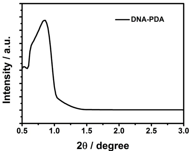
**Fig. S7** Small angle XRD pattern of DNA-PDA nanosheets synthesized at an hsDNA/dopamine weight ratio of 1.5:1.
