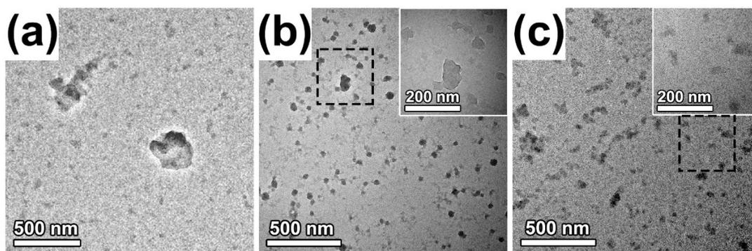
**Fig. S11** TEM images of DNA-PDA nanoplatelets synthesized with different DNA: 100-250 bp (a), ~2000 bp (b), and ~20000 bp (c). Magnified images of selected domains in (b) and (c) were presented in the insets.
