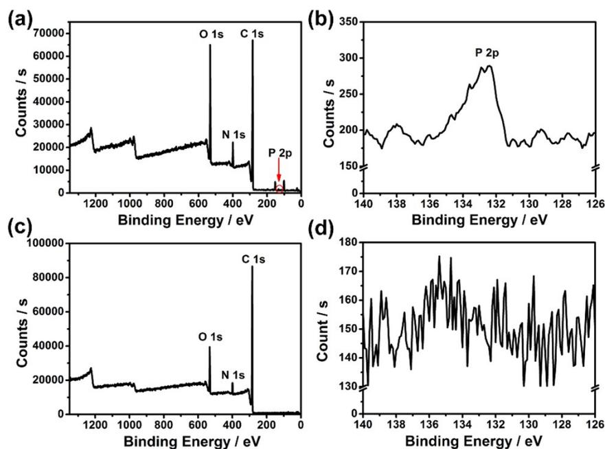
**Fig. S9** XPS survey of DNA-PDA nanosheets (a), PDA nanoparticles (c), and corresponding high-resolution scans of P2p peak from the XPS spectra of nanosheets (b) and nanoparticles (d).
