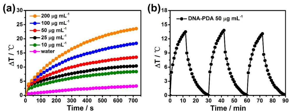
**Fig. S16** (a) Photothermal heating curves of aqueous suspensions of DNA-PDA nanosheets (200, 100, 50, 25, 10  $\mu\text{g mL}^{-1}$ , and pure water) during 808 nm laser irradiation ( $0.5 \text{ W cm}^{-2}$ , 12 min). (b) Recycling heating profiles of an aqueous suspensions of nanosheets ( $50 \mu\text{g mL}^{-1}$ ) under 808 nm laser irradiation ( $0.5 \text{ W cm}^{-2}$ , 12 min) for three laser on/off cycles. The nanosheets were synthesized at DNA/dopamine weight ratio of 1.5:1.
