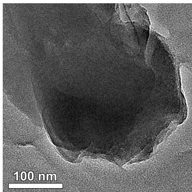
**Fig. S4** TEM image of intermediate products from the DNA-PDA nanoplatelets synthesis at the reaction time of 2 h.
