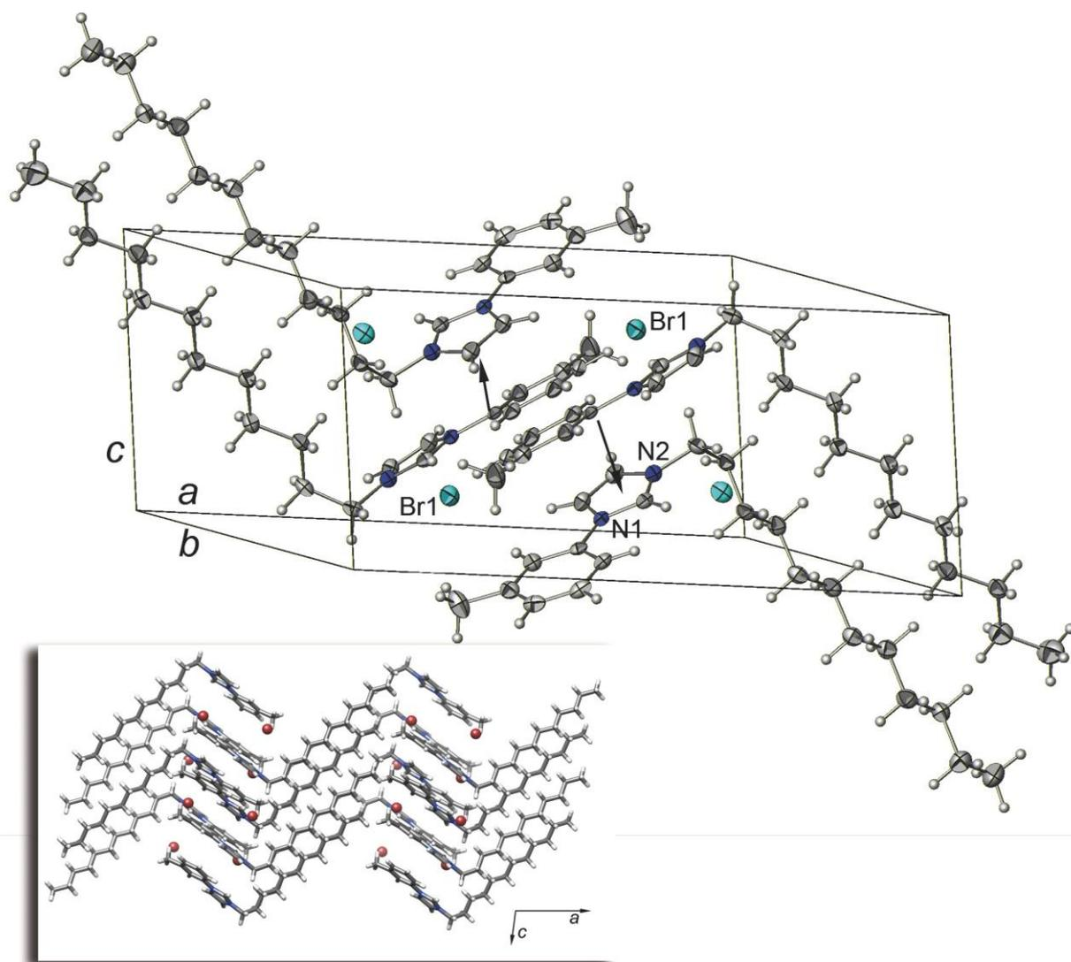
Fig X2 : ORTEP view and a packing view of compound 4\_Br. The ellipsoids enclose 90% of the electronic density. Selected weak interactions (CH- $\pi$ ) are represented with arrows.
