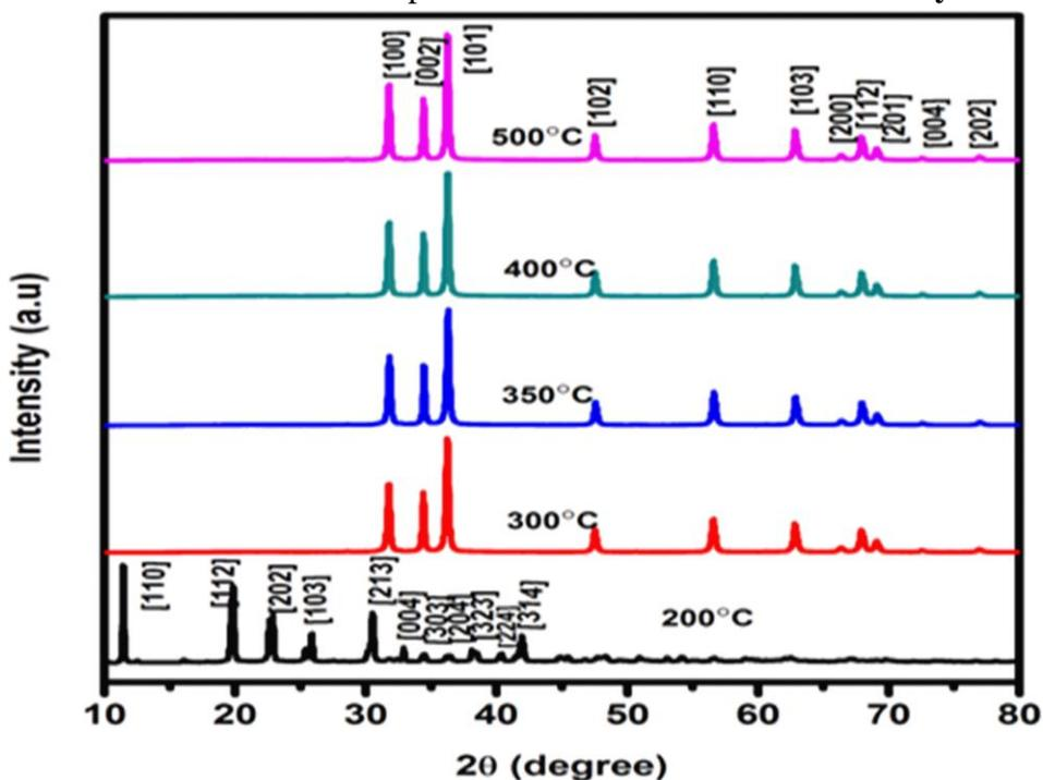
**Figure S1.** XRD patterns of as-synthesized pristine ZnO nanorods at various temperature.
