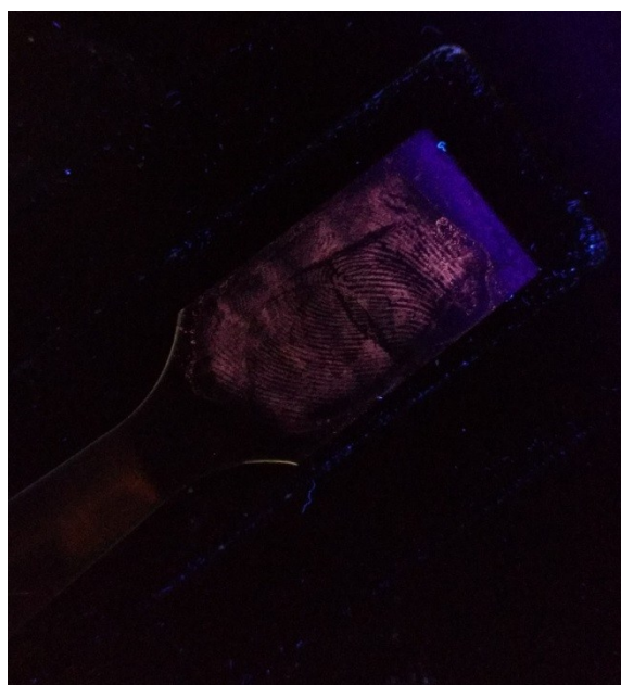
Fig. S11. LFP developed with DPSA (1 mM, 90% H 2 O-CH 3 CN) on stainless steel surface.
