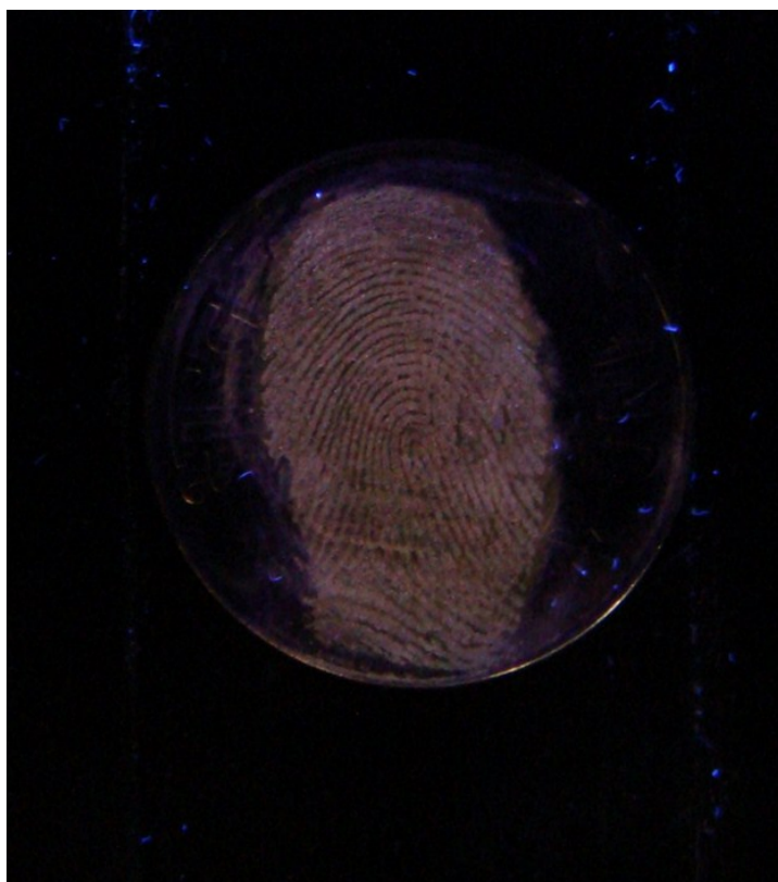
Fig. S12. LFP developed with DPSA (1 mM, 90% H 2 O-CH 3 CN) on metal coin surface.
