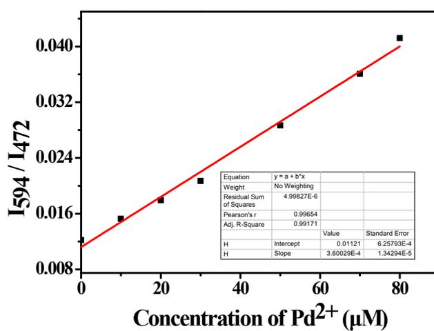
**Figure S4** The linear relationship between the fluorescence intensity ratio ( $I_{594}/I_{472}$ ) and the concentration of  $\text{Pd}^{2+}$  ( $\lambda_{\text{ex}} = 400 \text{ nm}$ ).
