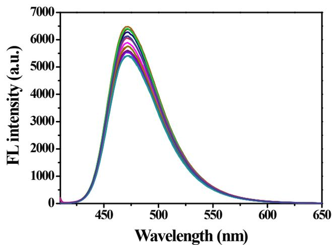
**Figure S2** The Fluorescence intensity titration profiles of Control Compound **3** (10  $\mu\text{M}$ ) in the presence of  $\text{Pd}^{2+}$  (0-150  $\mu\text{M}$ ) in PBS buffer containing 50% EtOH as a cosolvent ( $\lambda_{\text{ex}} = 400 \text{ nm}$ ).
