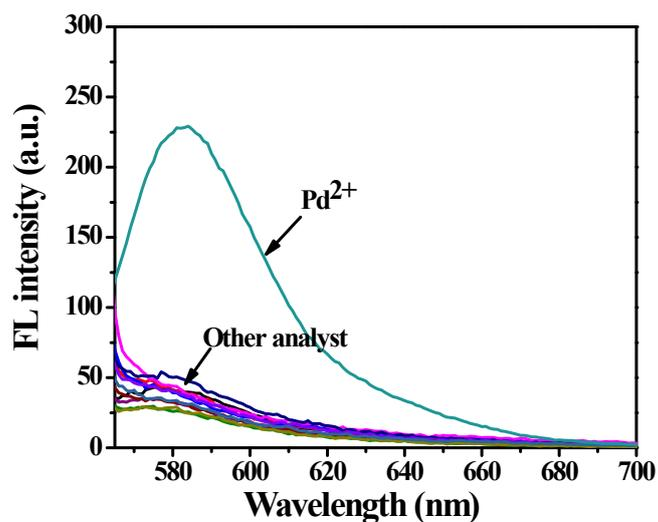
**Figure S5** The fluorescence spectra changes of probe **CR-Pd** (10  $\mu\text{M}$ ) in the presence of various analytes (50  $\mu\text{M}$ ) in PBS buffer containing 50 % EtOH as a cosolvent ( $\lambda_{\text{ex}}=550$  nm)
