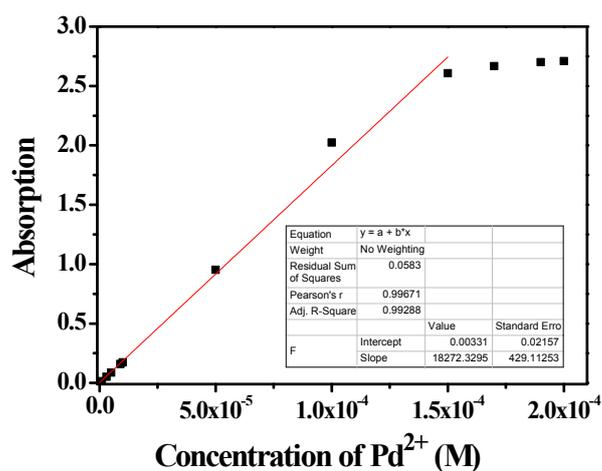
**Figure S1** The linear relationship between absorption intensity and probe **CR-Pd** concentration.
