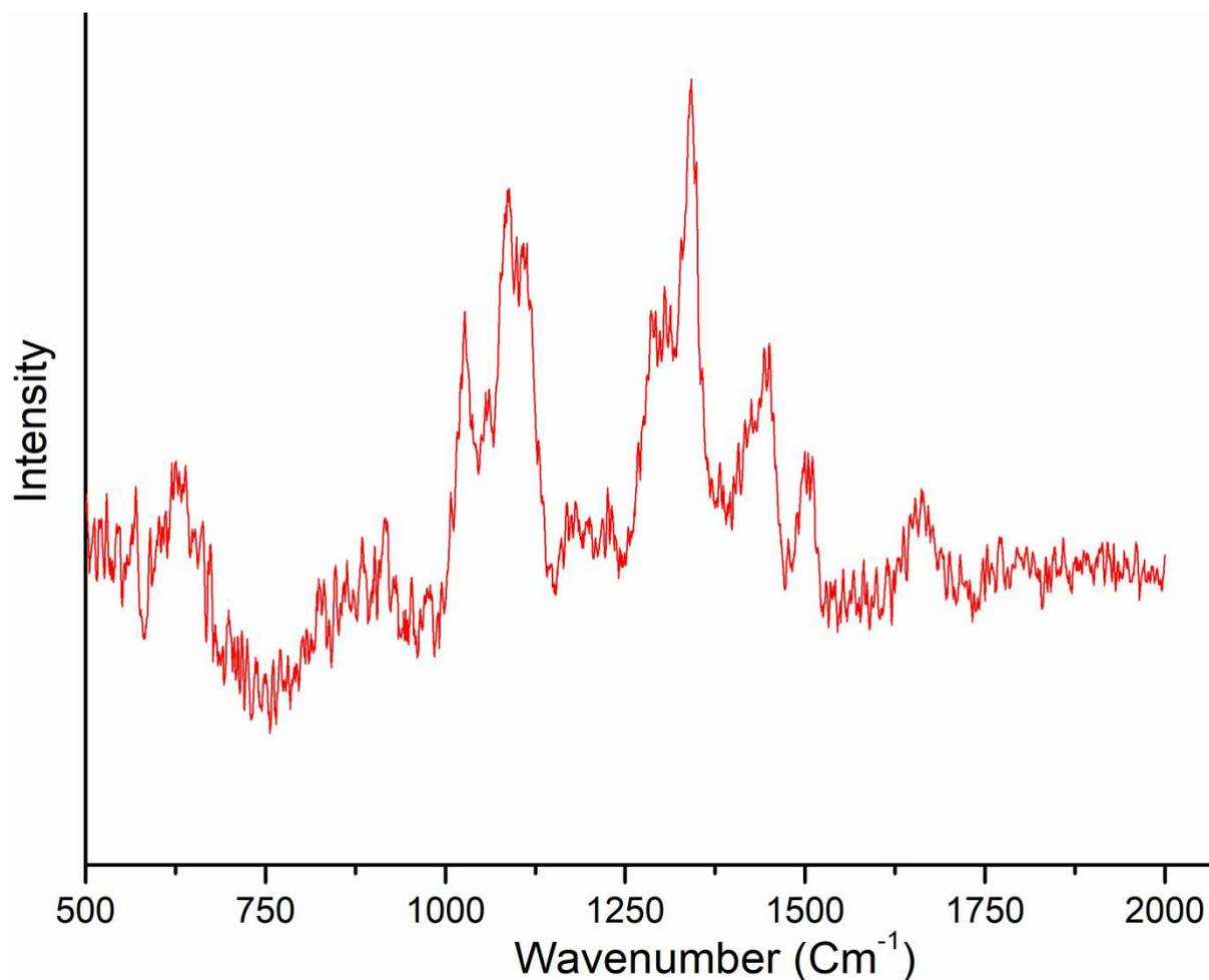
**Figure SI-1.** Raman spectrum of the crosslinked Poly(1-butyl-3-vinylimidazolium bromide) (PIL)
