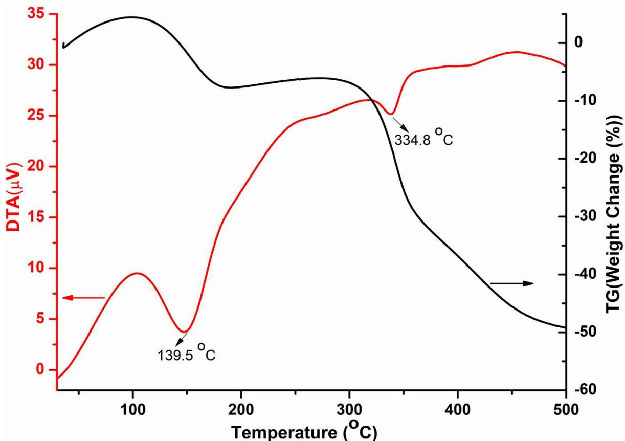
**Figure SI-2:** TG-DTA curves of the crosslinked poly(1-butyl-3-vinylimidazolium bromide) (PIL)
