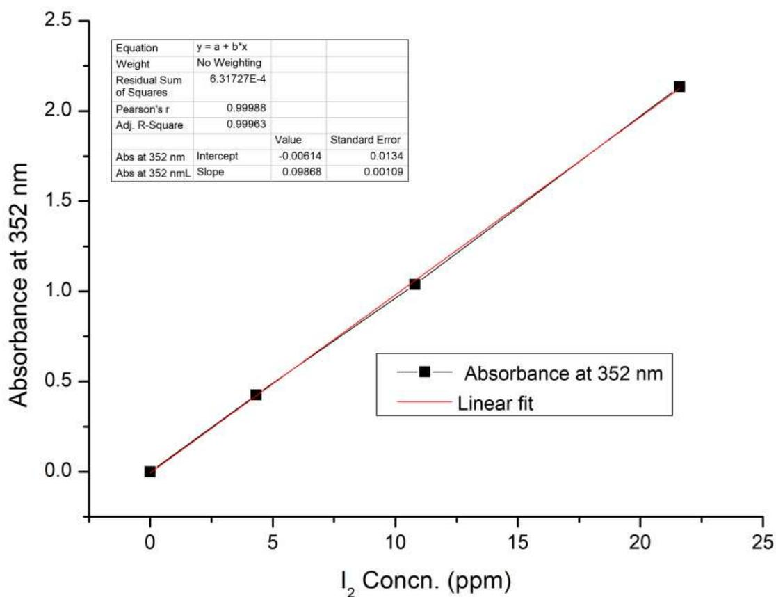
**Fig. SI-3.** Calibration curve obtained for iodine standards in the triiodide method of iodine estimation
