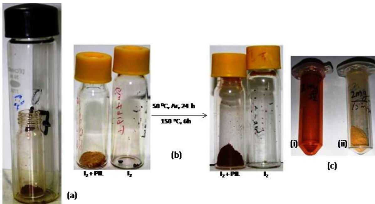
**Figure SI-4.** (a) Iodine binding by PIL from solid iodine crystals; (b) Binding and retention of iodine vapours by the PIL under heating and argon flow (c) Iodine crystals in (i) polypropylene (PP) vial, (ii) in PP vial containing PIL, both kept at room temperature
