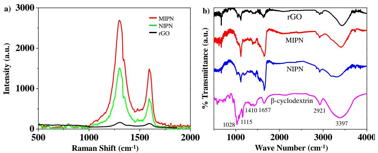
**Figure S4.** a) Raman spectra of MIPN/NIPN/rGO, showing the G band at  $\sim 1600 \text{ cm}^{-1}$  that corresponds to  $\text{sp}^2$  hybridized carbon atoms and D band at  $\sim 1300 \text{ cm}^{-1}$  that corresponds to defective  $\text{sp}^2$  hybridized carbon atoms. b) FTIR spectra of rGO, MIPN, NIPN and  $\beta$ -cyclodextrin, showing the presence of  $\beta$ -cyclodextrin in the nanocomposites.
