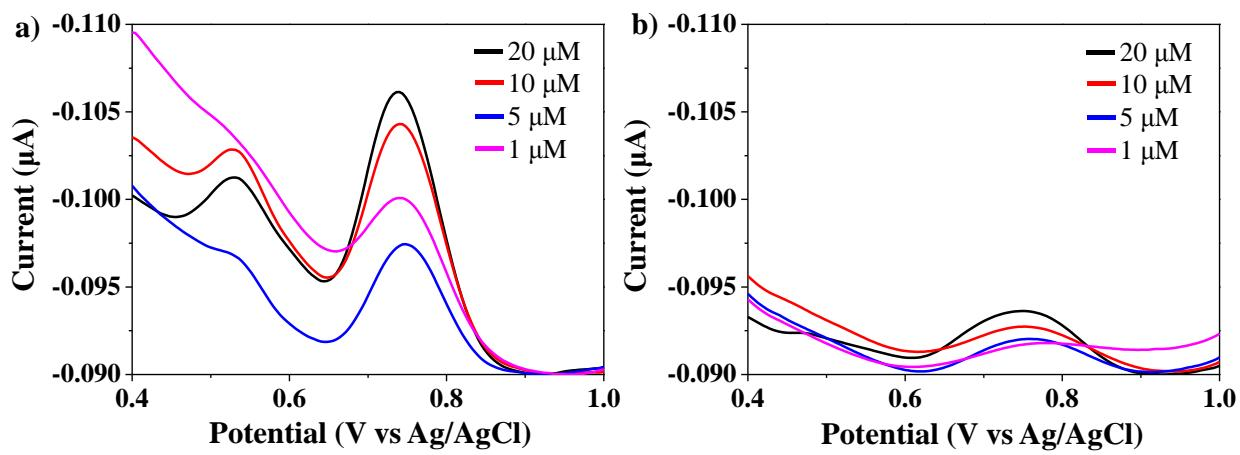
**Figure S18.** Differential pulse voltammograms at various concentration of bisphenol A using GCE modified by MIPN (a) and NIPN (b) in presence of 5  $\mu\text{M}$  phenol solution.
