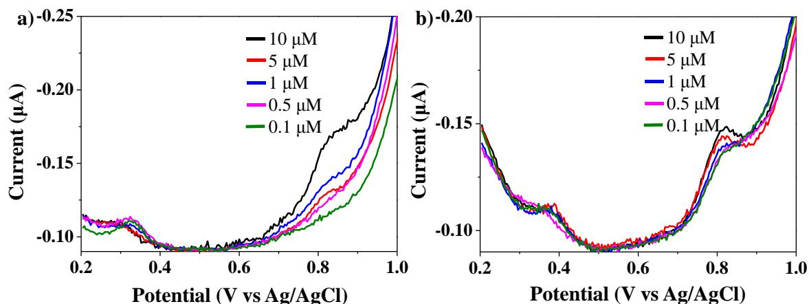
**Figure S10.** Differential pulse voltammograms at various concentration of BPAF using GCE modified by MIPN (a) and NIPN (b). The peak at  $\sim + 0.82$  V corresponds to BPAF oxidation peak.
