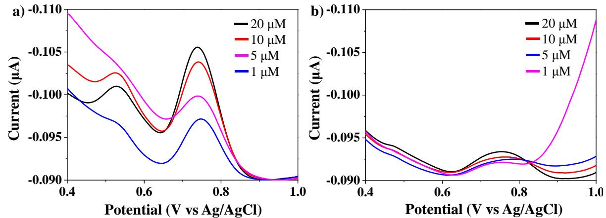
**Figure S19.** Differential pulse voltammograms at various concentration of bisphenol A using GCE modified by MIPN (a) and NIPN (b) in presence of 5  $\mu\text{M}$  resorcinol solution.
