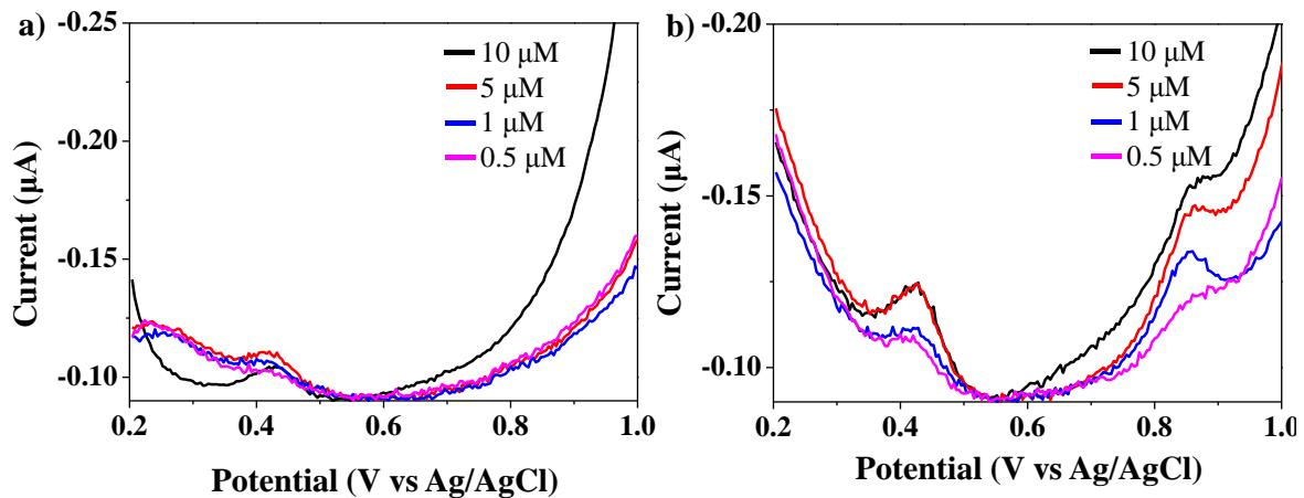
**Figure S11.** Differential pulse voltammograms at various concentration of BPB using GCE modified by MIPN (a) and NIPN (b). The peak at  $\sim + 0.85$  V corresponds to BPB oxidation peak.
