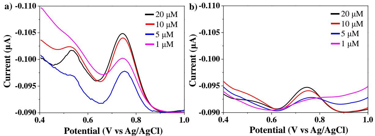
**Figure S16.** Differential pulse voltammograms at various concentration of bisphenol A using GCE modified by MIPN (a) and NIPN (b) in presence of 5  $\mu\text{M}$  BPB solution.
