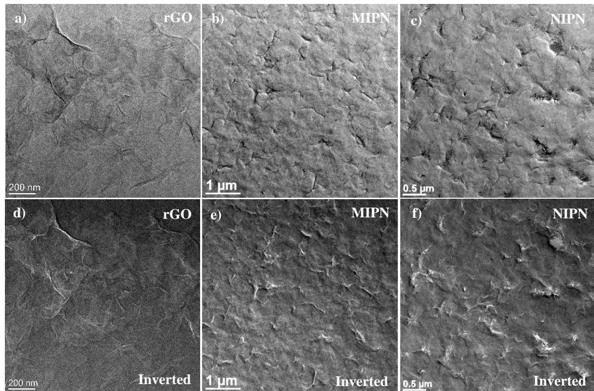
**Figure S5.** Low resolution TEM image (a-c) and corresponding inverted image (d-f) of rGO, MIPN and NIPN, showing the 3D structures of the MIPN/NIPN nanocomposites.
