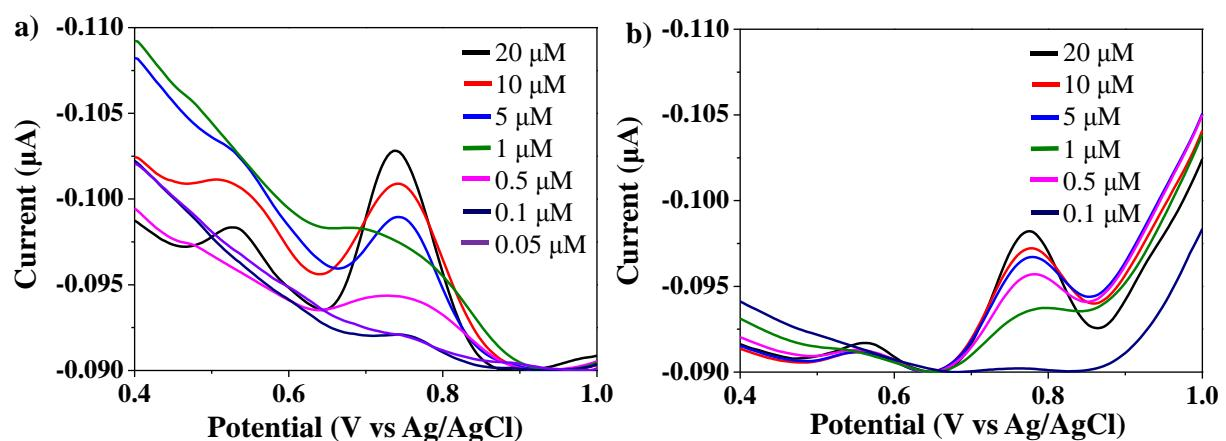
**Figure S8.** Differential pulse voltammograms at various concentration of bisphenol A in BR buffer 4.0 using GCE modified by MIPN2 (a) and NIPN2 (b). The peak at  $\sim +0.74$  V corresponds to bisphenol A oxidation peak.
