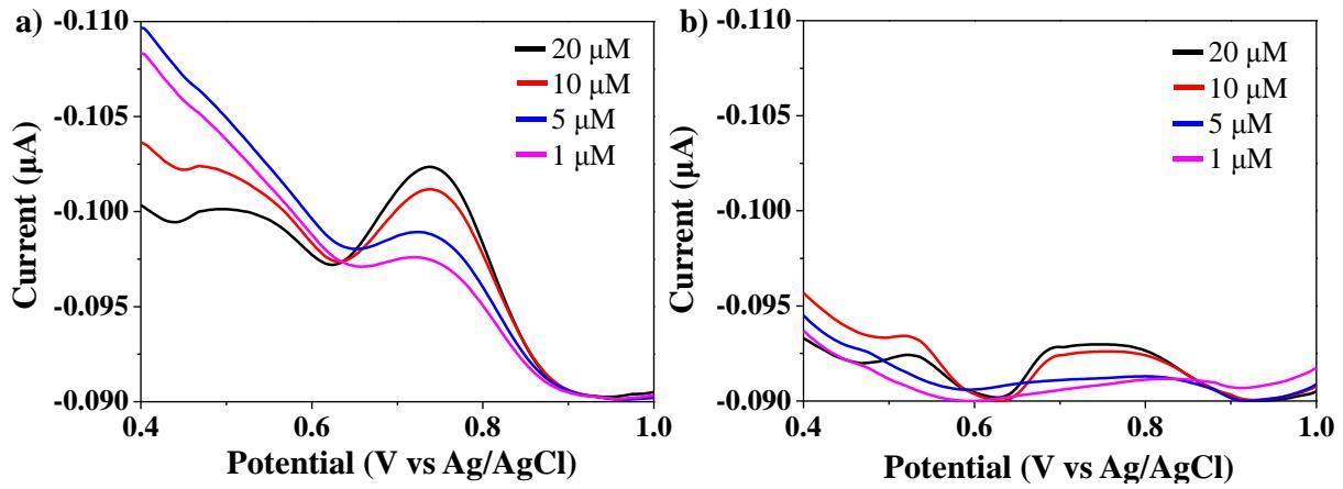
**Figure S15.** Differential pulse voltammograms at various concentration of bisphenol A using GCE modified by MIPN (a) and NIPN (b) in presence of 5  $\mu\text{M}$  BPAF solution.
