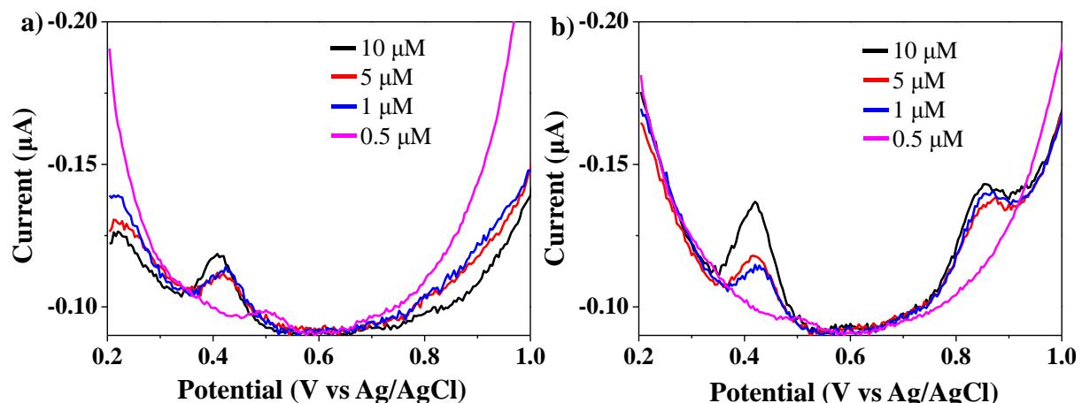
**Figure S12.** Differential pulse voltammograms at various concentration of DHBP using GCE modified by MIPN (a) and NIPN (b). The peak at  $\sim + 0.83$  V corresponds to DHBP oxidation peak.
