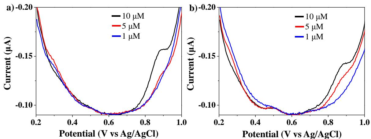
**Figure S14.** Differential pulse voltammograms at various concentration of resorcinol in BR buffer 4.0 using GCE modified by MIPN (a) and NIPN (b). The peak at  $\sim + 0.9$  V corresponds to resorcinol oxidation peak.
