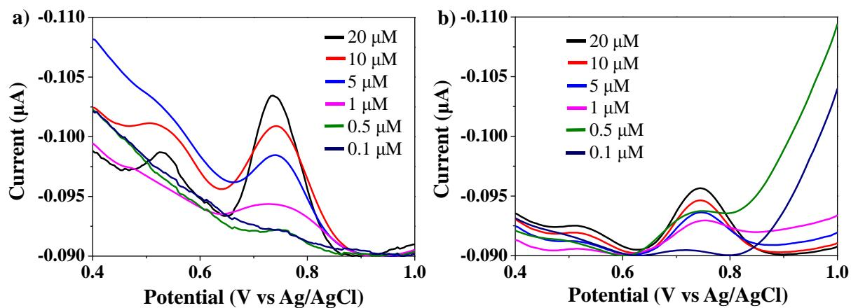
**Figure S7.** Differential pulse voltammograms at various concentration of bisphenol A in BR buffer 4.0 using GCE modified by MIPN1 (a) and NIPN1 (b). The peak at  $\sim +0.74$  V corresponds to bisphenol A oxidation peak.
