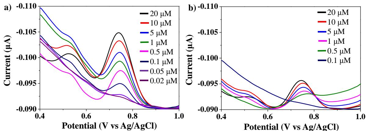
**Figure S9.** Differential pulse voltammograms at various concentration of bisphenol A in BR buffer 4.0 using GCE modified by MIPN (a) and NIPN (b) in presence of Tween 80 solution. The peak at  $\sim + 0.74$  V corresponds to bisphenol A oxidation peak.
