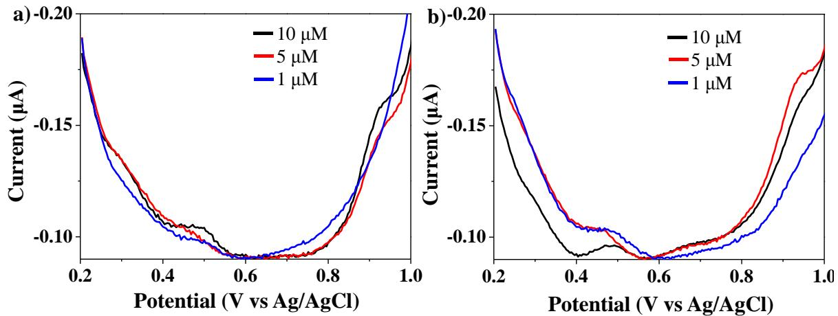
**Figure S13.** Differential pulse voltammograms at various concentration of phenol using GCE modified by MIPN (a) and NIPN (b). The band at  $\sim + 0.9$  V corresponds to phenol oxidation peak.
