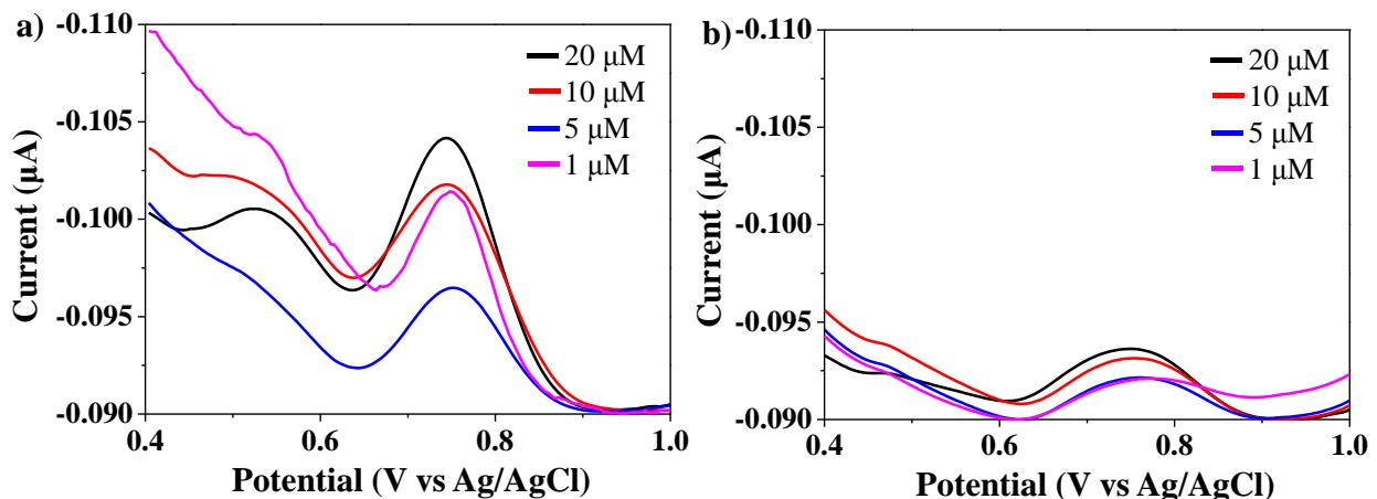
**Figure S17.** Differential pulse voltammograms at various concentration of bisphenol A using GCE modified by MIPN (a) and NIPN (b) in presence of 5  $\mu\text{M}$  DHBP solution.
