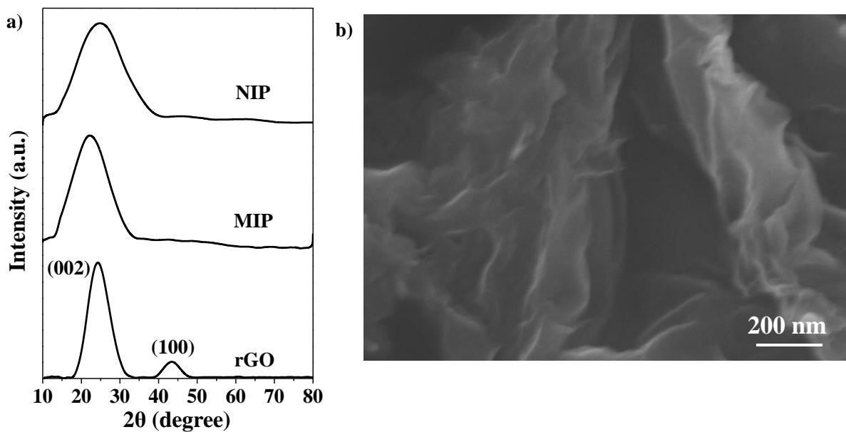
**Figure S3.** a) XRD patterns of rGO, MIPN and NIPN, showing the characteristic reflections at  $2\theta$  of  $24^\circ$  for (002) planes. The peak at  $2\theta$  of  $24^\circ$  indicates amorphous nature of the nanocomposites. b) FESEM image of reduced graphene oxide.
