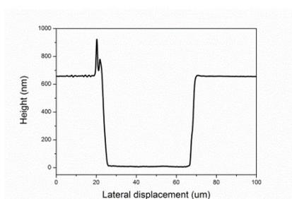
Figure S2. Profile of PMMA coating over PET
