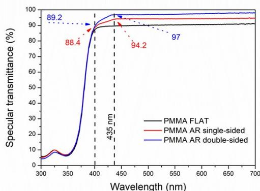
Figure S7. Reduction in transmittance due to scattering losses caused by the moth-eye topography. The spectra compares PMMA free standing films with a flat pristine surface, a film patterned on one side and with both sides patterned.
