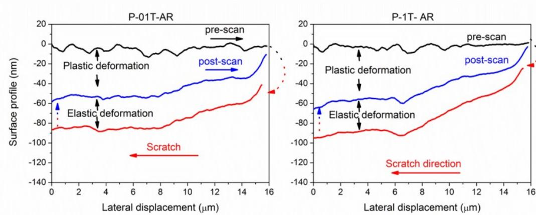
Figure S14. Normal scratch displacement profiles on P-01T-AR and on P-1T-AR substrates upon application of a constant normal force of 100  $\mu\text{N}$ .
