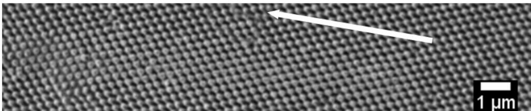
Figure S15. Scratch marks after nanoscratch tests on a P-AR and P-1T-AR substrates using a constant normal force of 100  $\mu\text{N}$ . The nanocones display plastic deformation in the scratch direction (indicated by the white arrow).
