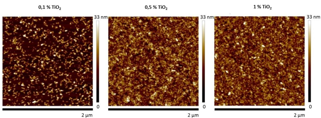
Figure S3. Morphological characterization of TiO<sub>2</sub> layer prior to imprinting.
