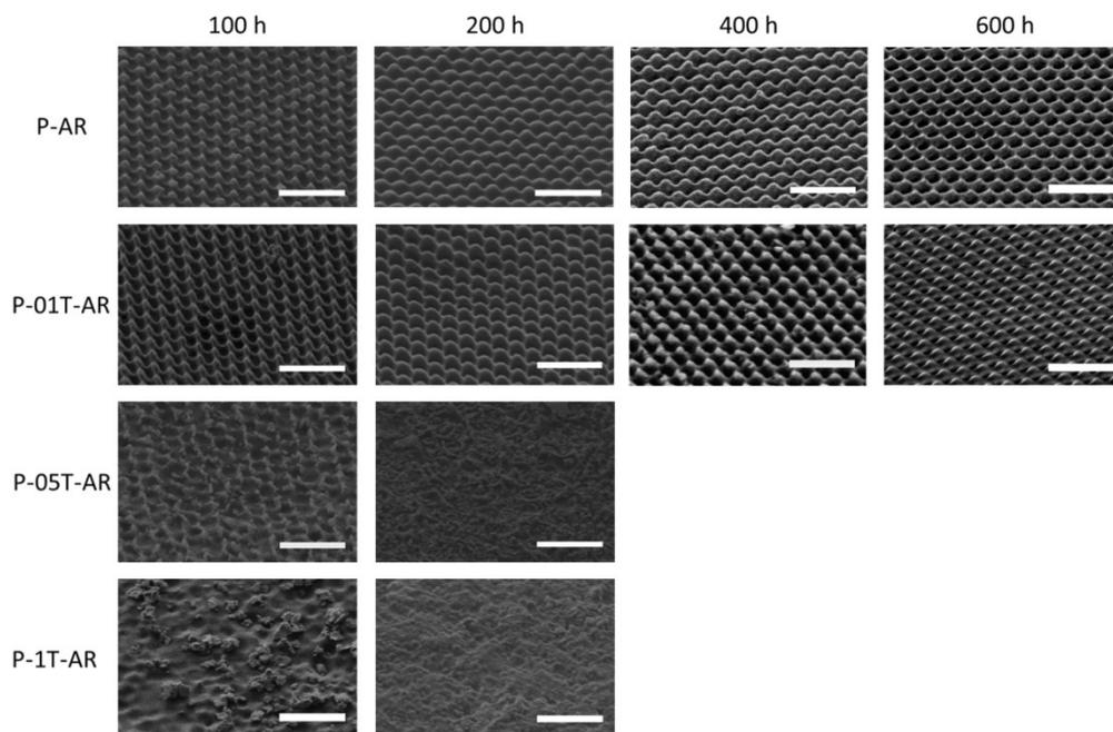
Figure S10. SEM images after the accelerated weathering tests. It can be observed that the moth-eye topography of the P-01T-AR substrate remained after 600h of exposure. However, the P-05T-AR and P-1T-AR substrates suffered substantial photo-degradation after 100 h of exposure. Scale bars correspond to 1 micron.
