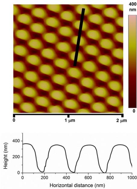
Figure S4: AFM height image of a P-AR substrate and cross-section profile corresponding to the black line.
