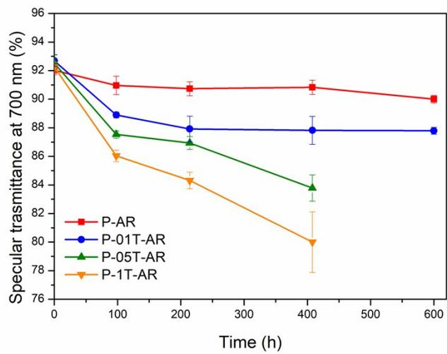
Figure S11. Optical transmittance variation as function of weathering time
