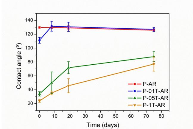
Figure S9. Hydrophobicity recovery of the UV irradiated substrates in wet conditions after a period of storage at room temperature in dry conditions.
