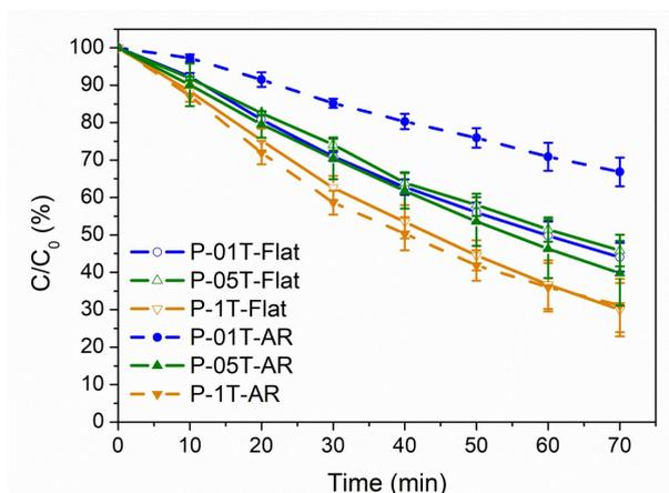
Figure S8. Comparison of photocatalytic activity between imprinted and non-imprinted samples with equal  $\text{TiO}_2$  load.
