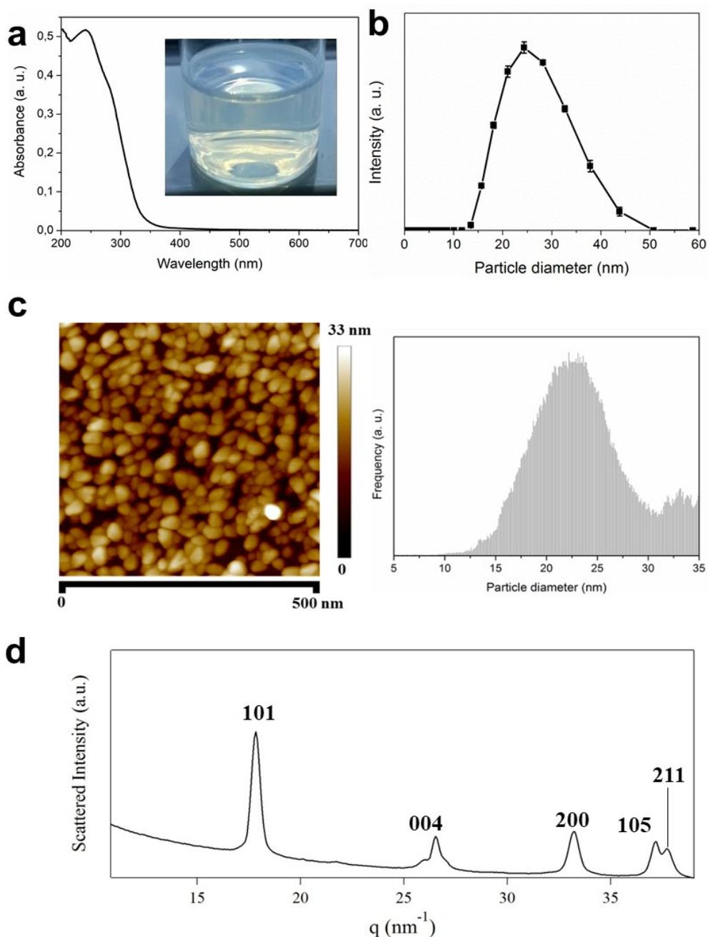
Figure S1: TiO<sub>2</sub> nanoparticle characterization: (a) Absorbance spectrum for synthesized TiO<sub>2</sub> nanoparticles and digital photograph of colloidal nanoparticles dispersion. (b) Dynamic light scattering size measurements. (c) AFM image of TiO<sub>2</sub> layered nanoparticles (1 wt %) prior imprinting. (d) 1D intensity WAXD profiles derived from the radial integration of the 2D diffraction patterns. The Miller indices of the main reflections are indicated.
