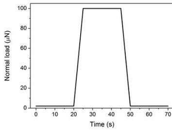
Figure S13. Representative load profile corresponding to a scratch test
