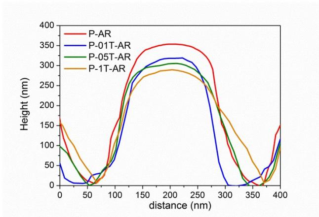
Figure S5. AFM profiles of a single moth-eye cone corresponding to the different TiO<sub>2</sub> composites tested.
