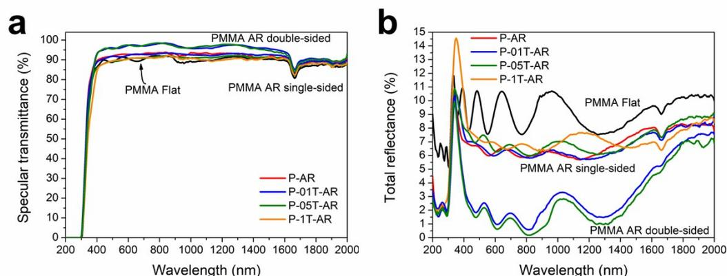
Figure S6. Extended transmission and reflection spectra of the moth-eye imprinted nanocomposite surfaces (200-2000 nm). a) Specular transmission spectra. b) Total reflection spectra.
