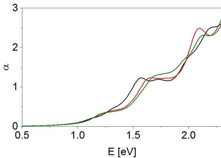
**Figure S2.** Convergence of the absorption spectrum of monolayer WSe<sub>2</sub> with a SV defect with respect to  $k$ -point sampling. Black, red, and green are for  $3\times 3\times 1$ ,  $4\times 4\times 1$ , and  $5\times 5\times 1$   $k$  samplings, respectively.
