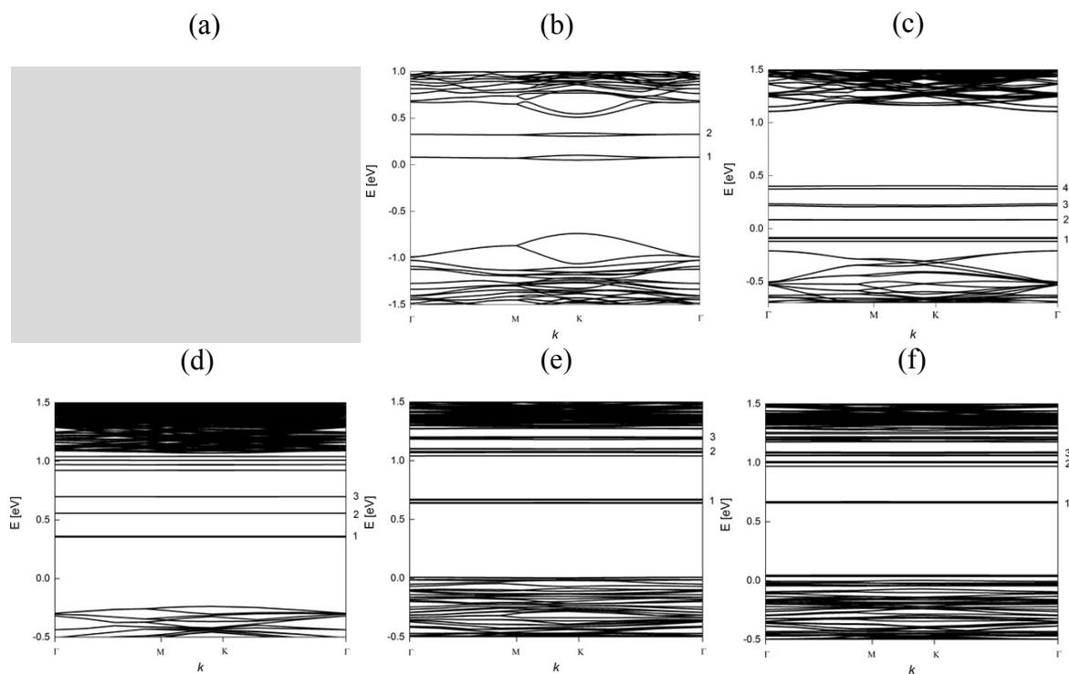
**Figure S3.** PBE+SOC band structures for monolayer WSe<sub>2</sub> with (a) SV, (b) DV, (c) WV, (d) T<sub>1</sub>, (e) T<sub>2</sub>, and (f) T<sub>3</sub> defects. Bound defect bands are numerically labelled.
