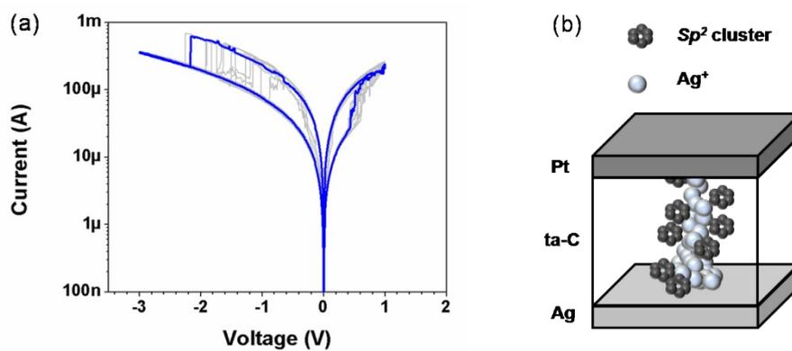
**Figure S7.** (a)  $I$ - $V$  measurements during 10x bipolar switching cycles for a single-layer Ag/ta-C/Pt device. (b) Schematic diagram of the single layer device.
