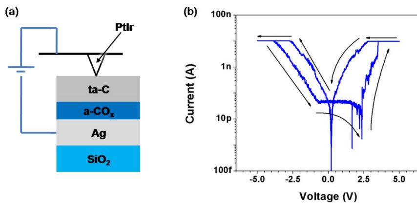
**Figure S5.** (a) Schematic diagram of the C-AFM experiment performed with a PtIr-coated tip of nominal radius  $25 \pm 5$  nm. The root mean square roughness of the device (without the Pt top electrode) was determined to be  $<0.5$  nm. (b) I-V curves obtained from the C-AFM experiments showing reversible bipolar resistive switching on the nanoscale.
