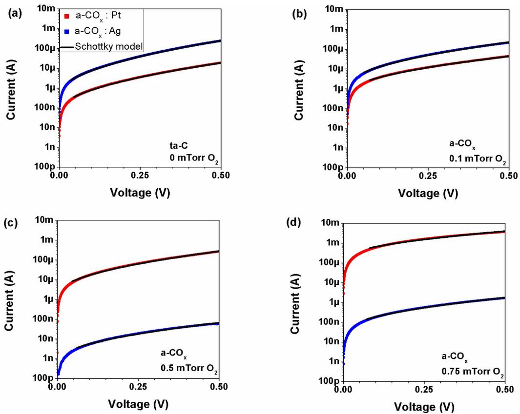
**Figure S3.** Schottky emission model fitting to  $I$ - $V$  curves fitting of the  $a\text{-CO}_x$  films deposited at  $\text{O}_2$  partial pressures of (a) 0 mTorr, (b) 0.1 mTorr, (c) 0.5 mTorr and (d) 0.75 mTorr contacted by Pt (blue) and Ag (red).
