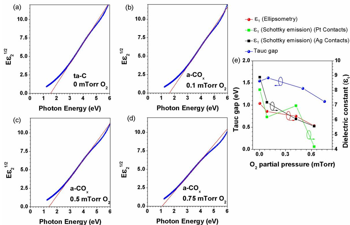
**Figure S4.** Optical properties of a- $CO_x$  films determined by spectroscopic ellipsometry. (a-d) Tauc plots constructed from the imaginary component of the dielectric function,  $\epsilon_2$ . (e) Optical (Tauc) band gap and real dielectric constant measured at 633nm as a function of oxygen partial pressure. The dielectric constants extracted from Schottky emission plots (Supplementary Fig. S2) are also shown for comparison.
