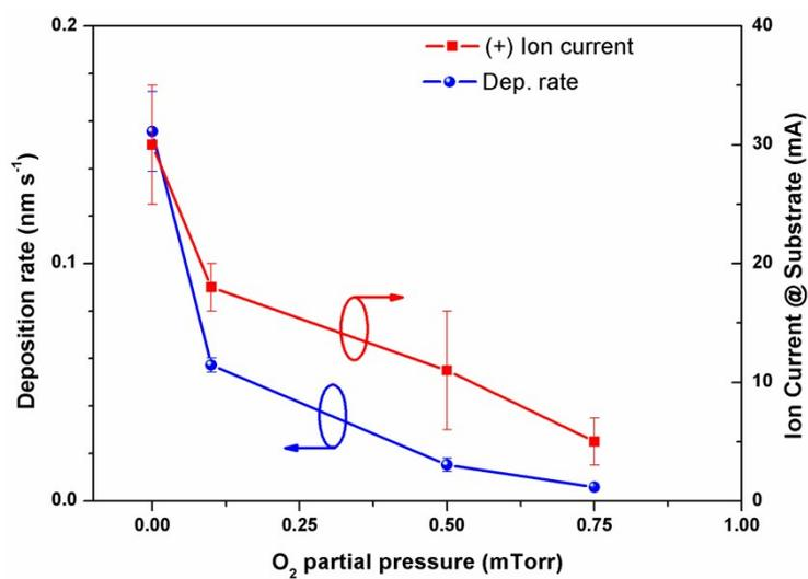
**Figure S2.** Deposition rate and positive ion current at the substrate measured during filtered cathodic vacuum arc (FCVA) deposition of a-CO<sub>x</sub> films in O<sub>2</sub> atmospheres. The ion current and deposition rate are both reduced proportionally as the pressure is increased. The film growth is inhibited by scattering of the depositing ions rather than due to sputtering at the substrate.
