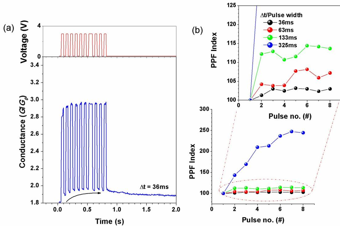
**Figure S6.** (a) Paired-pulse facilitation (PPF) in response to a voltage-pulse train is observed when the post-(1<sup>st</sup>)pulse conductance is low ( $<5 G_0$ ). (b) PPF in response to voltage pulse trains (3V) at time interval  $\Delta t$ . Note, the pulse width during this experiment was made equivalent to  $\Delta t$ . The increase in PPF is due to the increase in pulse width.
