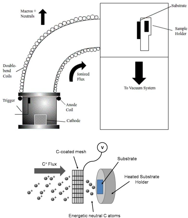
**Figure S1.** Schematic diagrams of FCVA deposition system and biased mesh apparatus for deposition of energetic neutral atoms.
