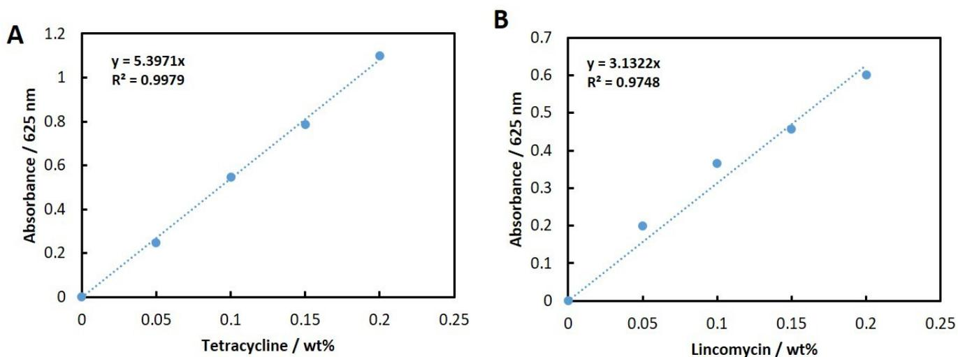
**Figure S2.** Standard calibration graphs of the absorption vs concentrations of (A) tetracycline and (B) lincomycin hydrochloride. Absorbance was measured at 625 nm. Aliquots were prepared by adding antibiotic hydrochlorides to deionized water at specific concentrations.
