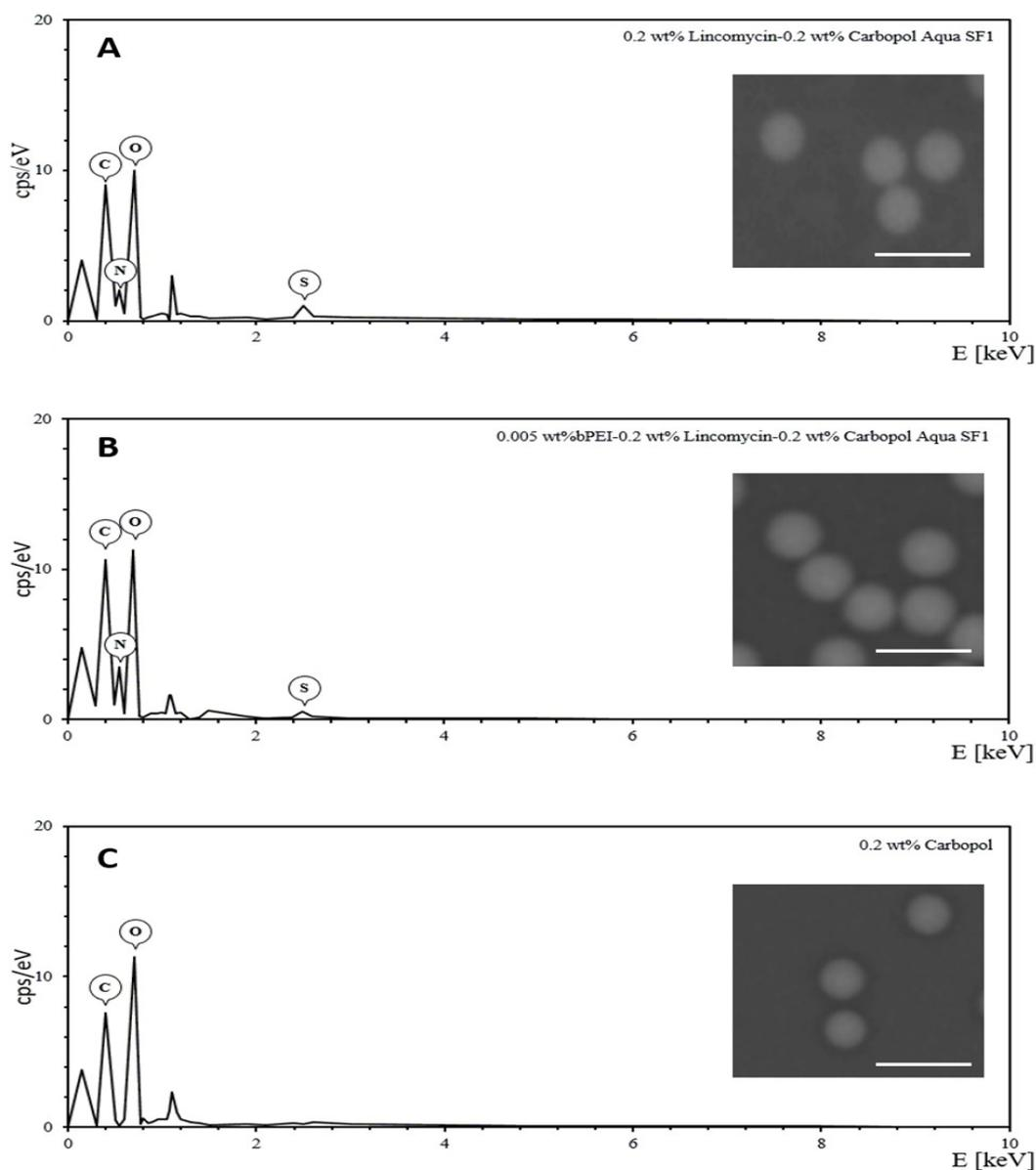
**Figure S4.** SEM images and EDX spectra of Carbopol Aqua SF-1 NPs. (A) shows spectra of 0.2 wt% lincomycin-0.2 wt% Carbopol Aqua SF1, (B) shows 0.005 wt% bPEI-0.2 wt% Lincomycin-0.2 wt%-0.2 wt% Carbopol Aqua SF1, and (C) 0.2 wt% empty Carbopol Aqua SF1. The measurement was taken in the centre of the NPs. Oxford Laboratories micF+ X-stream-2 EHX was used to take measurements, the results were analysed in Aztec One v.3.3. Images were acquired using a TM3030 Plus SEM. Scale bars represent 200 nm.
