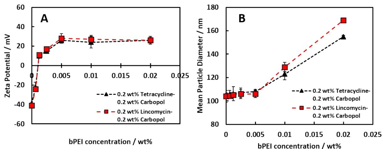
**Figure S3.** (A) The zeta potential of 0.2 wt% tetracycline-0.2 wt% Carbopol and 0.2 wt% lincomycin-0.2 wt% Carbopol NPs coated with various concentrations of bPEI and (B) the mean particle diameter of 0.2 wt% tetracycline-0.2 wt% Carbopol and 0.2 wt% lincomycin-0.2 wt% Carbopol NPs coated with various concentrations of bPEI. Each value represents a triple replicate with  $\pm$  S.D. The lines are guides to the eye.
