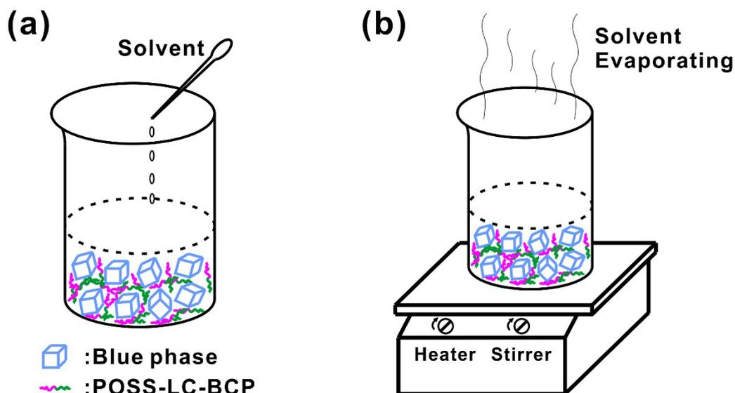
**Scheme S3** Preparation of PHEMAPOSS<sub>40</sub>-*b*-P6CBMA<sub>167</sub> (POSS-LC-BCP) doped BPLC. (a) Mixture of BPLC host and POSS-LC-BCP in dichloromethane. (b) The mixture was stirred at room temperature for at least 1 hour and heated to 50 °C for another 30 min to remove the solvent through evaporation.
