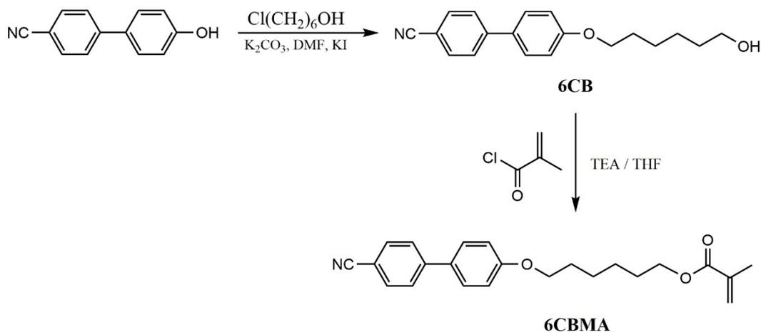
**Scheme S2** Synthesis of 6-(4-cyano-4'-biphenyloxy) hexyl methacrylate (6CBMA).
