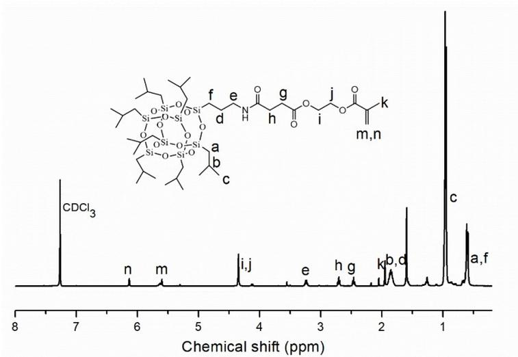
**Fig. S1**  $^1\text{H}$  NMR spectrum of HEMAPOSS in  $\text{CDCl}_3$ .
