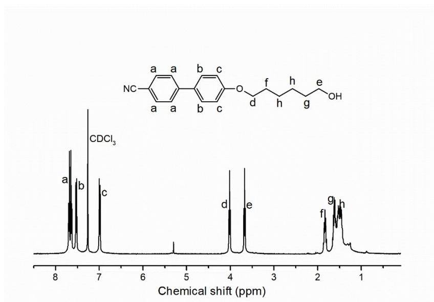
**Fig. S2**  $^1\text{H}$  NMR spectrum of 6CB in  $\text{CDCl}_3$ .
