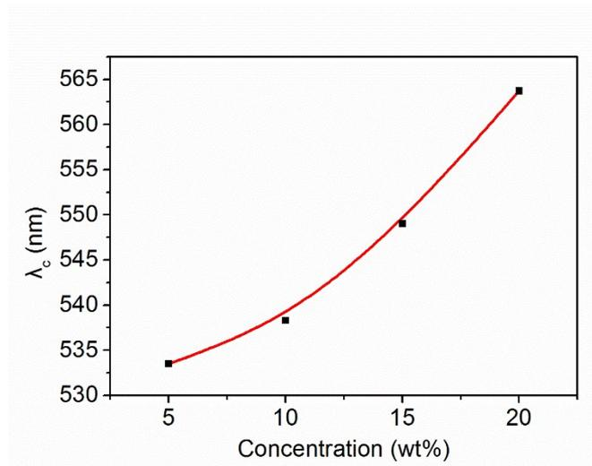
**Fig. S6** The  $\lambda_c$  of the samples with different concentration of LC BCPs.
