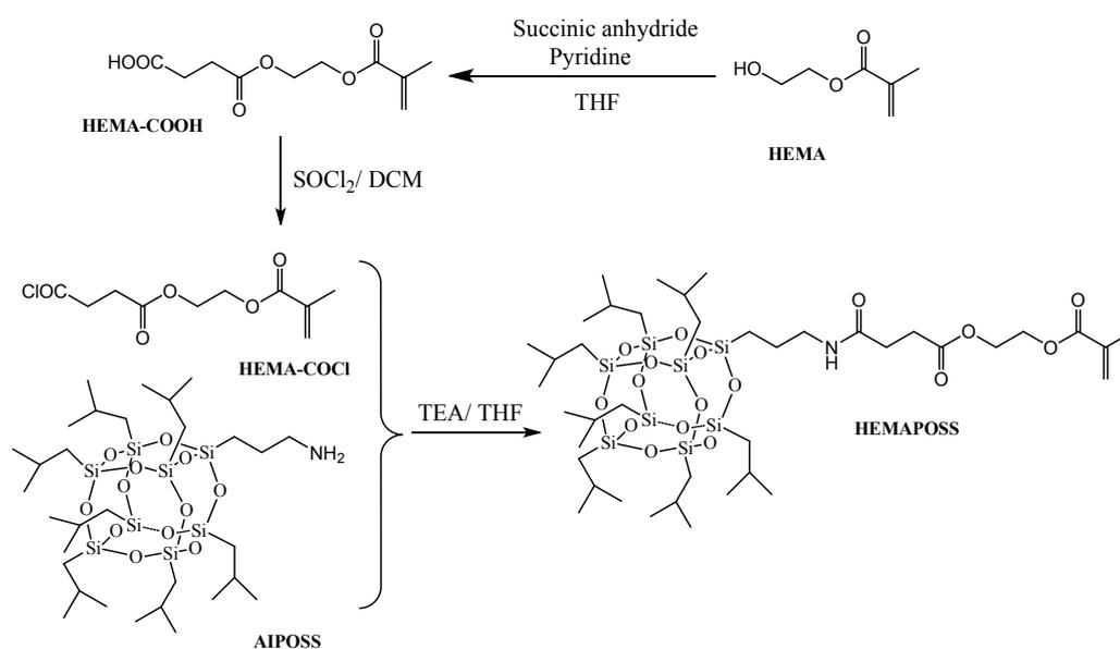
**Scheme S1** Synthesis of methacrylate isobutyl POSS monomer (HEMAPOSS).
