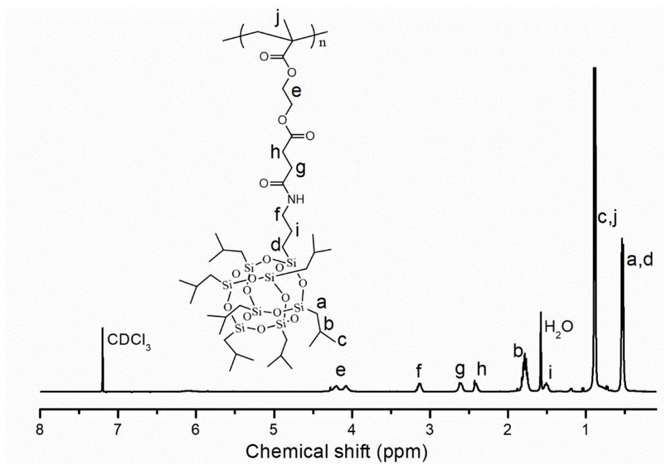
**Fig. S4** <sup>1</sup>H NMR spectrum of PHEMAPOSS<sub>40</sub> in CDCl<sub>3</sub>.
