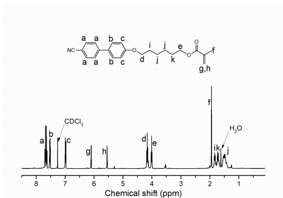
**Fig. S3** <sup>1</sup>H NMR spectrum of 6CBMA in CDCl<sub>3</sub>.
