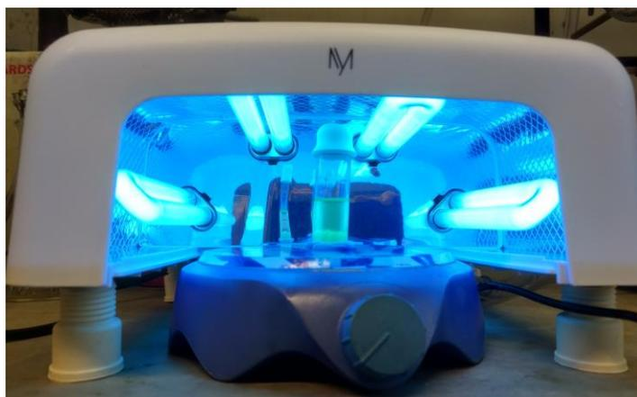
**Figure S1:** UV curing lamp used for polymerizations.
