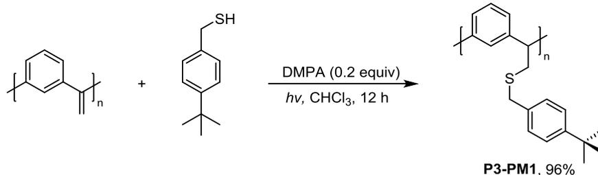
Polymer **P3** (20.4 mg, 0.2 mmol,  $M_n = 4.5$  kDa,  $M_w/M_n = 1.89$ ), (4-(tert-butyl)phenyl)methanethiol (180.3 mg, 1.0 mmol), DMPA (10.3 mg, 0.04 mmol), and  $\text{CHCl}_3$  (2 mL) were added into a 10 ml round-bottom flask. The mixture was stirred under 365 nm UV lamp at room temperature for 12 h and then precipitated into methanol (30 mL). A yellow solid (**P3-PM1**) was obtained in 96% yield after vacuum dryness.  $M_n = 9.4$  kDa,  $M_w/M_n = 3.25$ .
