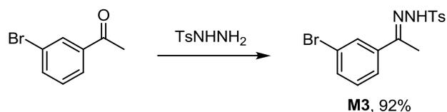
A mixture of 1-(3-bromophenyl)ethan-1-one (1.99 g, 10 mmol) and TsNHNH<sub>2</sub> (1.86 g, 10 mmol) in MeOH (10 mL) was heated to 50 °C until the carbonyl compound disappeared. The *N*-tosylhydrazones precipitated during the reaction. The precipitate was washed twice with MeOH and the white solid (**M3**, 3.3564 g, 92% yield) was obtained and used without further purification.
