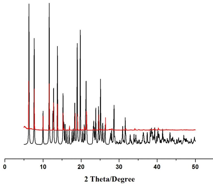
**Fig. S4** Powder X-ray diffraction patterns of simulated **1** (black) and as-synthesized **1** (red).
