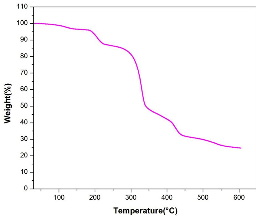
**Fig. S3** TGA plot of complex **1** measured under N<sub>2</sub> atmosphere.
