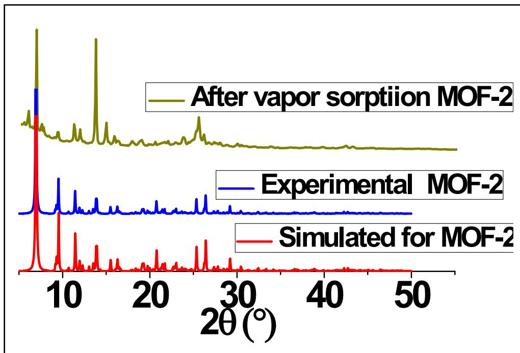
**Figure S25:** Comparison of PXRD pattern of MOF-2 before and after vapor sorption.
