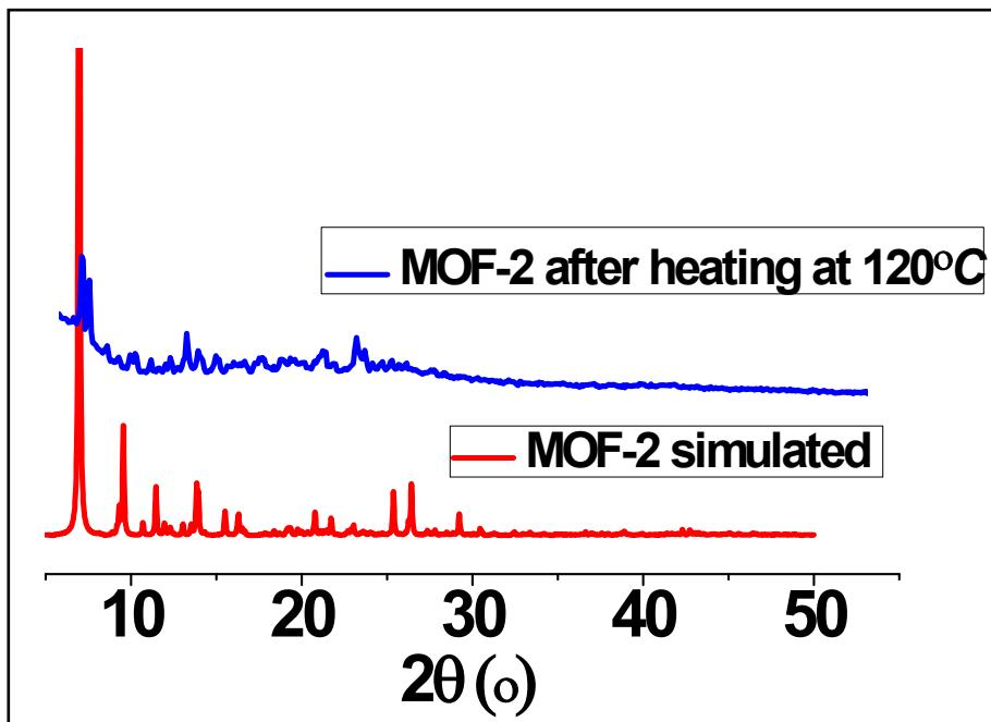
Figure S33: Comparison of PXRD patterns of MOF-2 after heat treatment.
