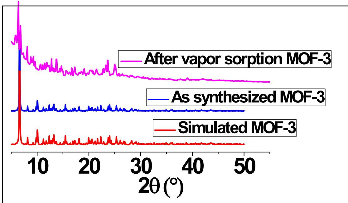
**Figure S26:** Comparison of PXRD patterns of MOF-3 before and after vapor sorption.
