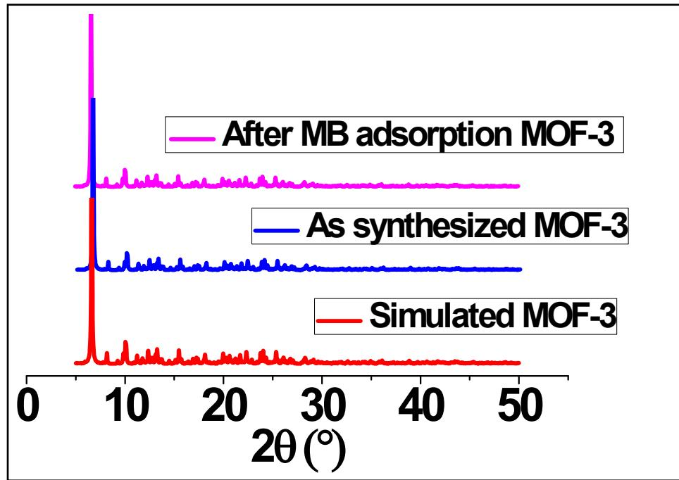
Figure S22: Comparison of PXRD patterns for MOF-3 after dye adsorption
