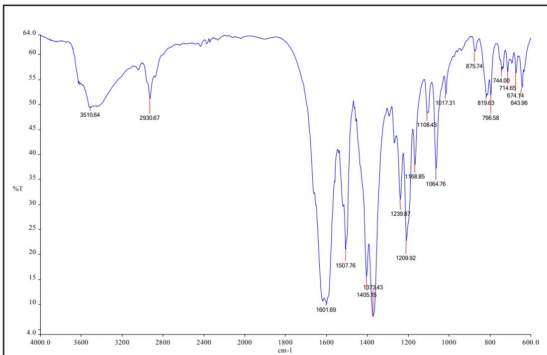
**Figure S10:** FTIR spectra for the MOF-3
