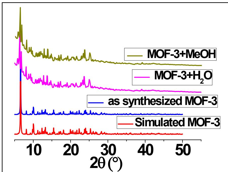
**Figure S30:** Comparison of PXRD patterns of MOF-3 in different solvents
