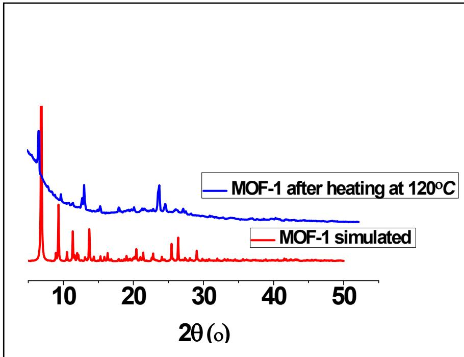
Figure S32: Comparison of PXRD patterns of MOF-1 after heat treatment.
