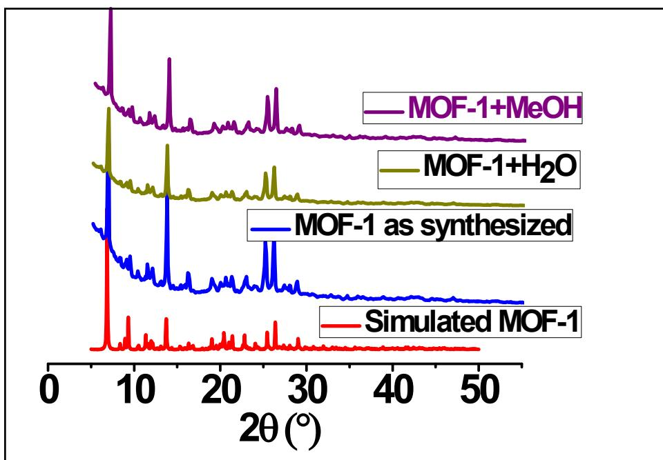
**Figure S28:** Comparison of PXRD patterns of MOF-1 in different solvents.
