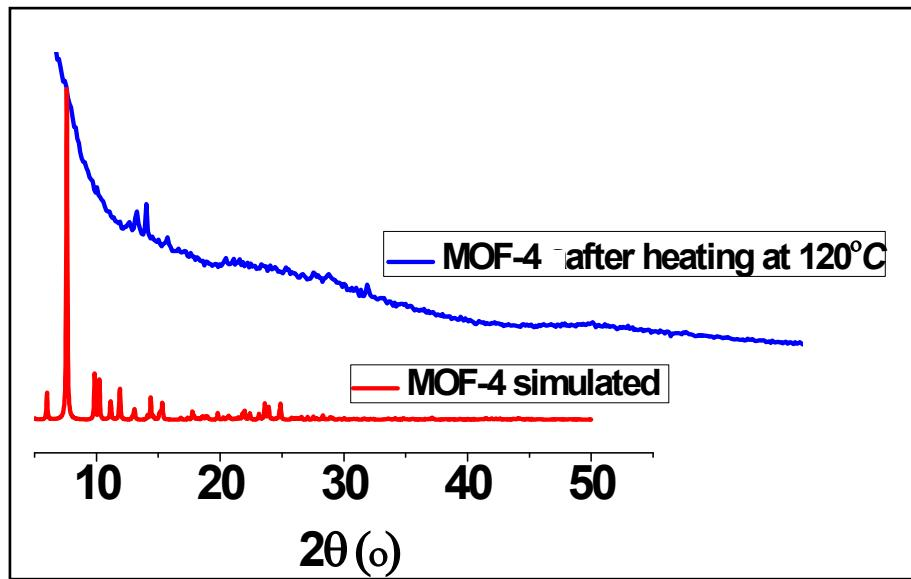
**Figure S35:** Comparison of PXRD patterns of MOF-4 after heat treatment.
