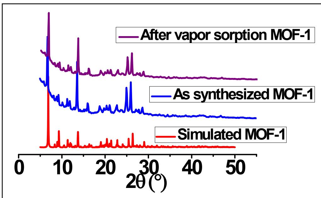
**Figure S24:** Comparison of PXRD patterns for MOF-1 before and after vapor sorption.
