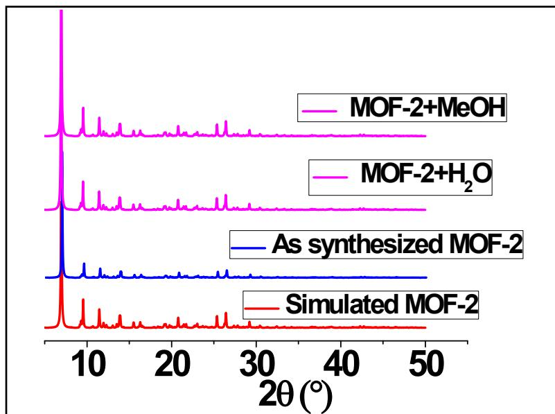
**Figure S29:** Comparison of PXRD patterns of MOF-2 in different solvents.
