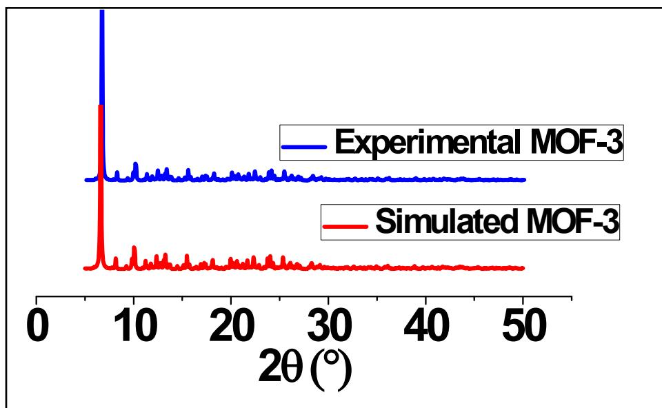
**Figure S5:** PXRD pattern of simulated and experimental for the MOF-3
