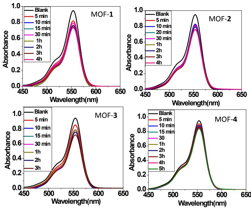
**Figure 19:** UV-vis spectra for the very low uptake of rhodamine B from aqueous solutions at various time intervals for MOFs 1-4 respectively.
