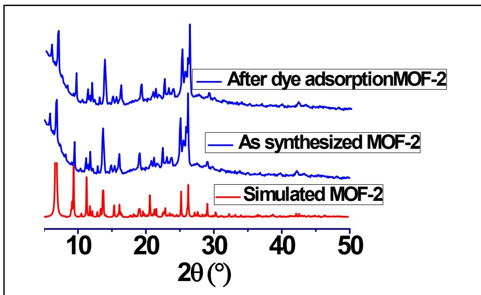
**Figure S21:** Comparison of PXRD patterns for MOF-2 after dye adsorption
