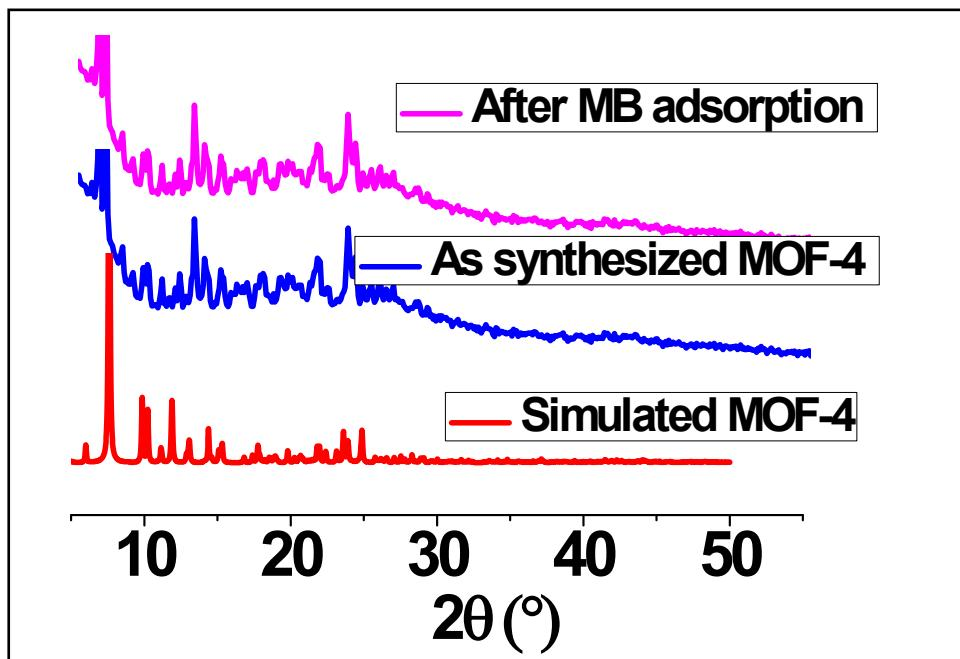
Figure S23: Comparison of PXRD patterns for MOF-4 after dye adsorption
