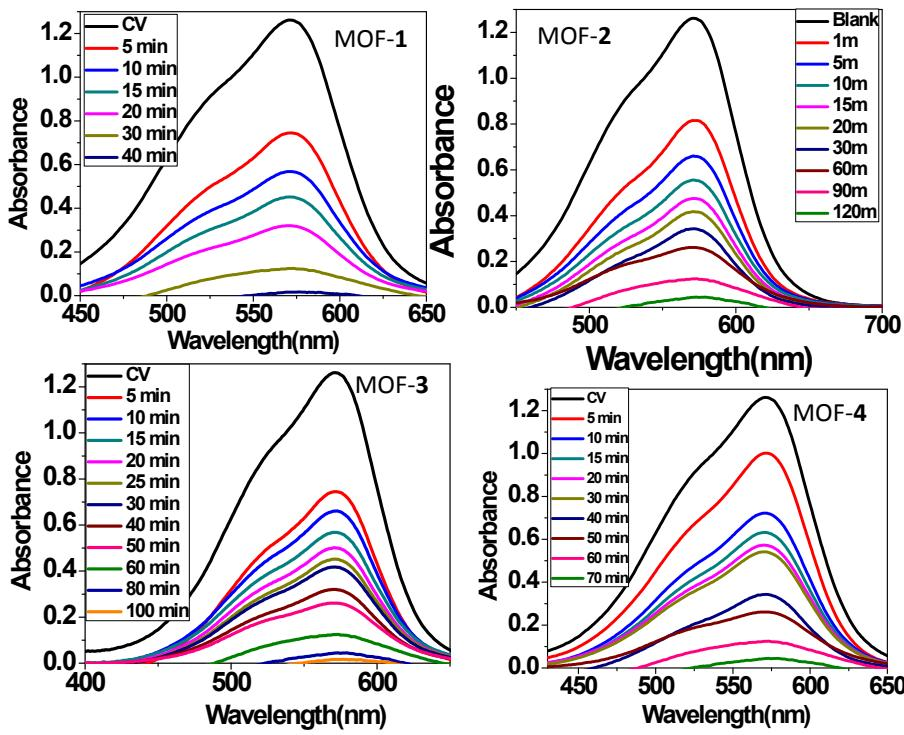
**Figure S18:** UV-vis spectra for the uptake of crystal violet from aqueous solutions at various time intervals for MOFs 1-4 respectively.
