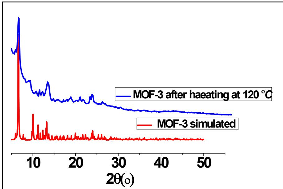
**Figure S34:** Comparison of PXRD patterns of MOF-3 after heat treatment
