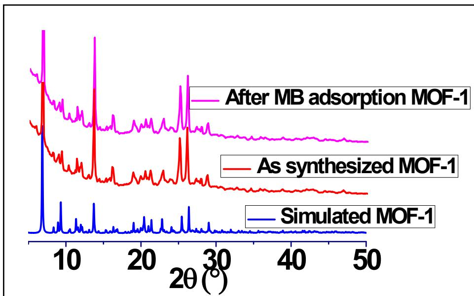
**Figure S20:** Comparison of PXRD patterns for MOF-1 after dye adsorption
