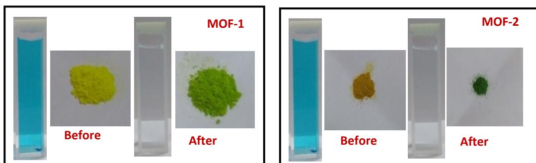
**Figure S16:** Illustration for the change in the color of the material after Methylene blue dye adsorption by MOFs 1-4 in aqueous solution
