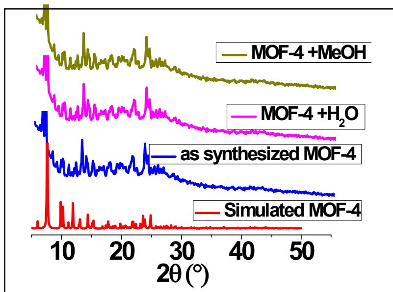
**Figure S31:** Comparison of PXRD patterns of MOF-4 in different solvents.
