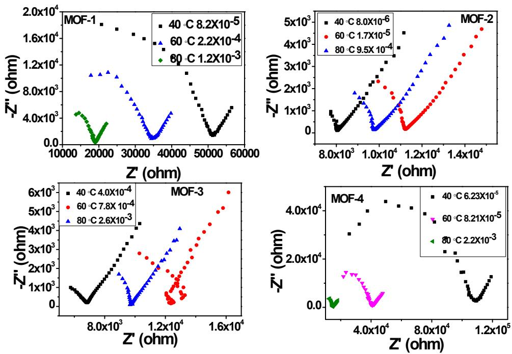
**Figure S14:** Nyquist plots for the MOFs 1-4 at 40, 50 and 60 °C temperature respectively and at 98% (RH).
