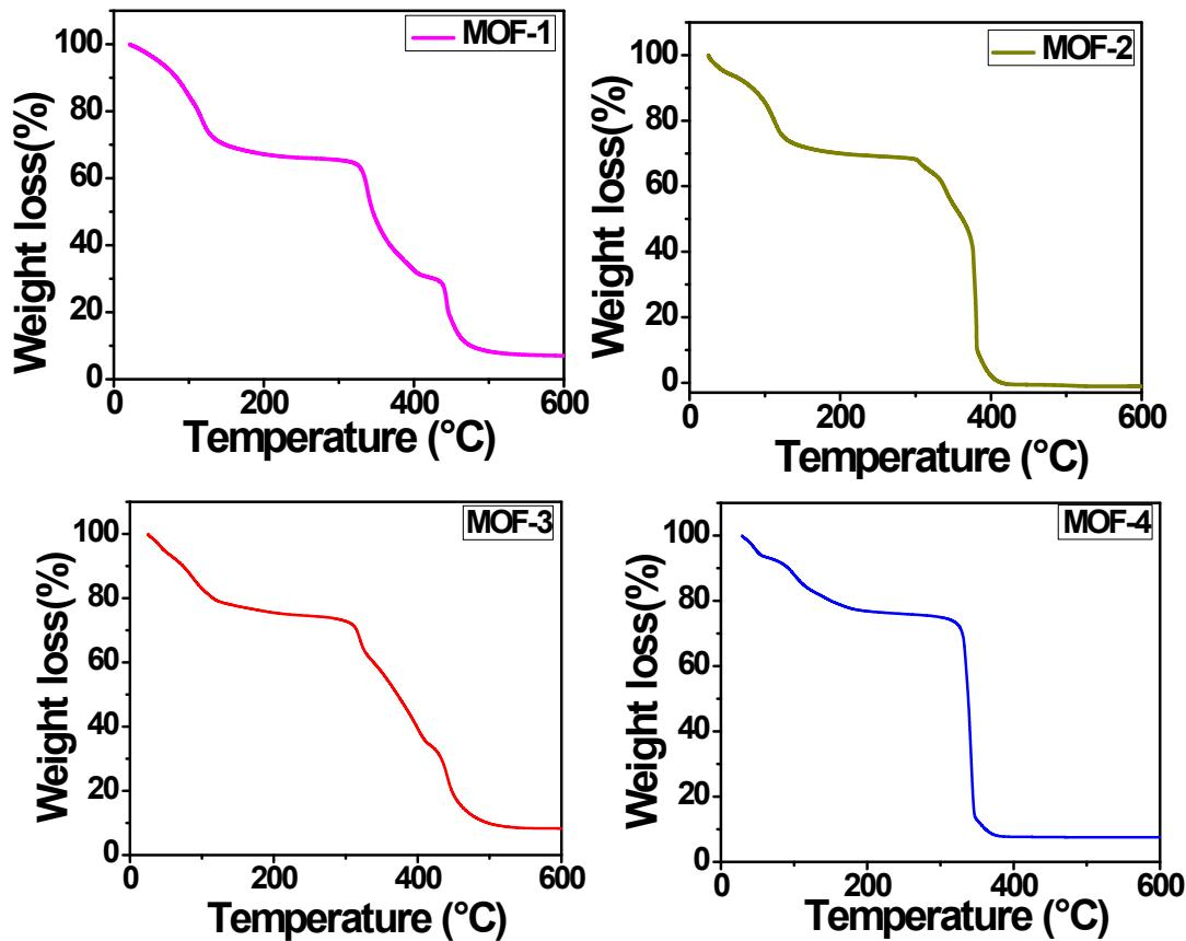
**Figure S12:** Thermogravimetric analysis graphs for the MOFs 1-4
