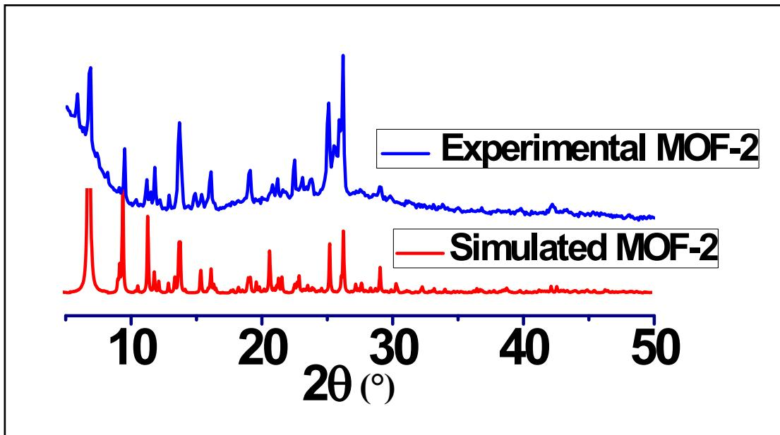
**Figure S4:** PXRD pattern of simulated and experimental for the MOF-2
