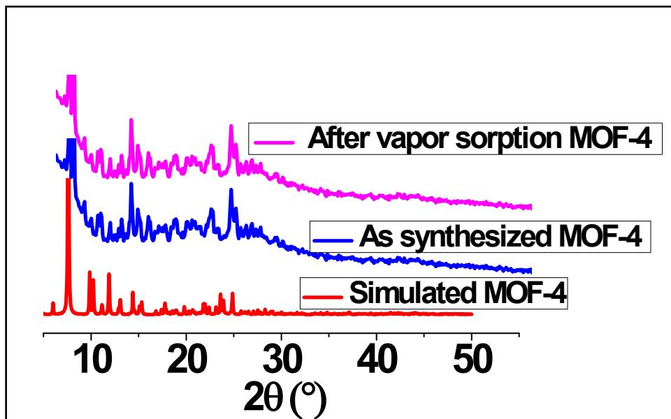
**Figure S27:** Comparison of PXRD patterns of MOF-4 before and after vapor sorption.
