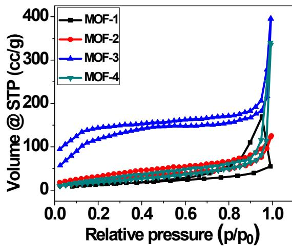
**Figure S13:**  $\text{N}_2$  adsorption and desorption isotherms at 273 K and at one bar for the MOFs 1-4
