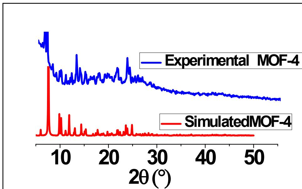
**Figure S6:** PXRD pattern of simulated and experimental for the MOF-4
