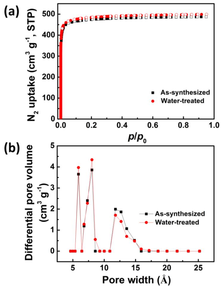
**Fig. S6** (a) N<sub>2</sub> isotherms at 77 K and (b) DFT pore size distributions of **ZJNU-100** before and after immersion in water at room temperature for 24 h.
