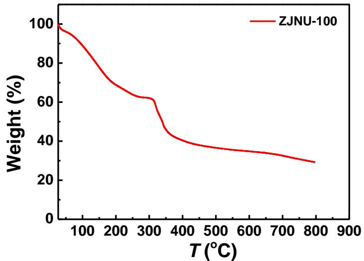
**Fig. S3** The TGA curve of **ZJNU-100** under nitrogen atmosphere.
