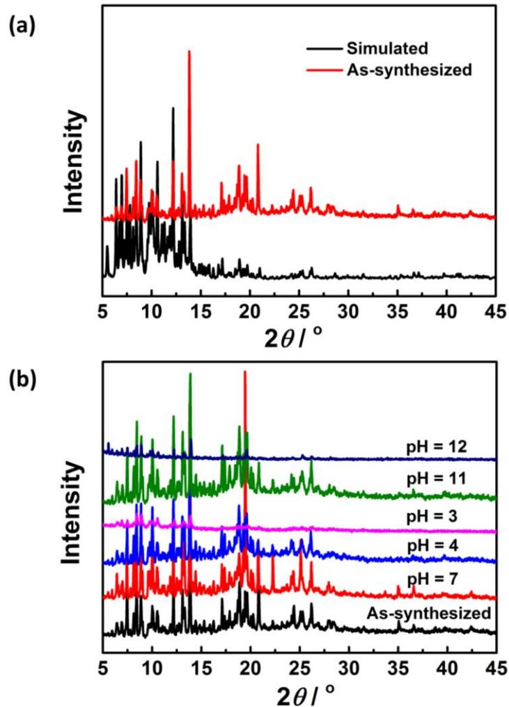
**Fig. S2** (a) The simulated (black) and experimental (red) PXRD patterns of **ZJNU-100**; (b) the PXRD patterns of **ZJNU-100** after immersion in aqueous HCl/NaOH solutions with pH ranging from 3 to 12 for 24 h.
