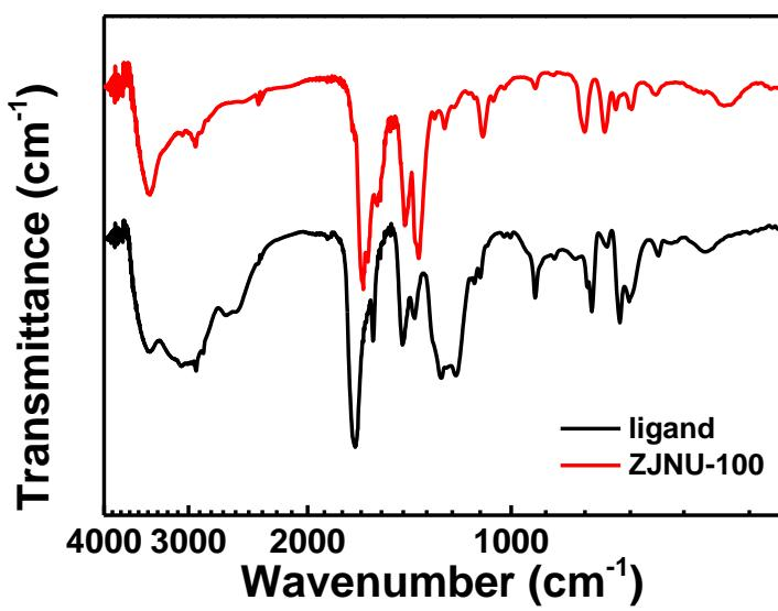
**Fig. S4** Comparison of FTIR spectra of **ZJNU-100** and its corresponding ligand  $\text{H}_6\text{L}$ .
