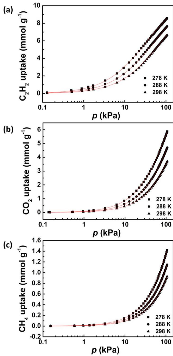
**Fig. S7** Comparison of the pure-component isotherm data for (a)  $\text{C}_2\text{H}_2$ , (b)  $\text{CO}_2$ , and (c)  $\text{CH}_4$  in **ZJNU-100** with the fitted isotherms at 278 K, 288 K, and 298 K.
