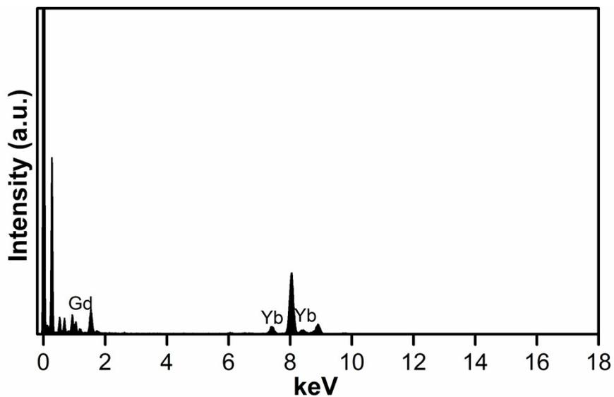
**Figure S9.** EDXA spectrum of the monodisperse 5.5 nm  $\beta$ -NaYbF<sub>4</sub>:Gd/Er(10/2%) prepared by reacting at 300 °C for 15 min.
