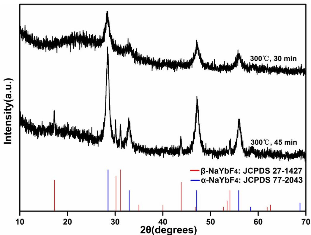
**Figure S5.** XRD patterns of  $\text{NaYbF}_4:\text{Er}$  prepared by using NaOA-based solvothermal strategy at the  $\text{NaOA}/\text{NH}_4\text{F}/\text{RE}$  ratio of 2.5:3.5:1 and different reaction time. The results showed pure  $\beta\text{-NaYbF}_4:\text{Er}$  could not be achieved even after reacting at 300 °C for 45 min by using such fluoride-deficient solvothermal environment.
