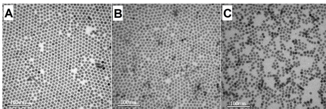
**Figure S1.** TEM images of  $\beta$ -NaYbF<sub>4</sub>:Er prepared by using NaOA-based solvothermal strategy with respective NH<sub>4</sub>F/RE ratio of 4.25:1 (A), 4.75:1 (B) and 5:1 (C). All the NC growth reactions were performed at 300 °C for 20 min.
