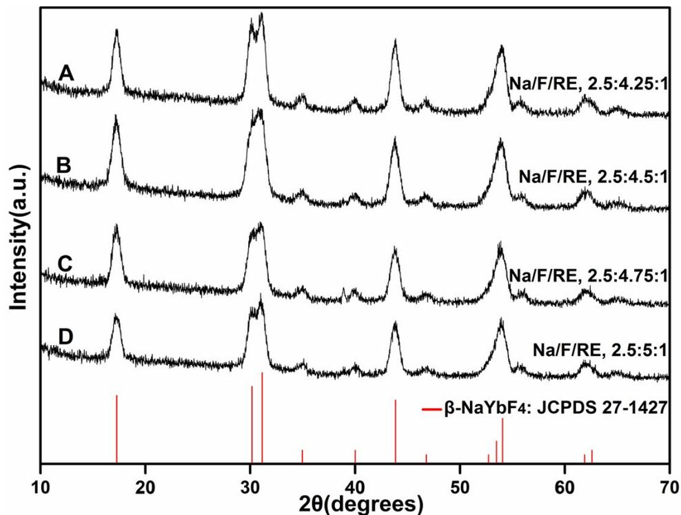
**Figure S2.** XRD patterns of NaYbF<sub>4</sub>:Er prepared by using NaOA-based solvothermal strategy but different Na/F/RE ratios. All the NC growth reactions were performed at 300 °C for 20 min.
