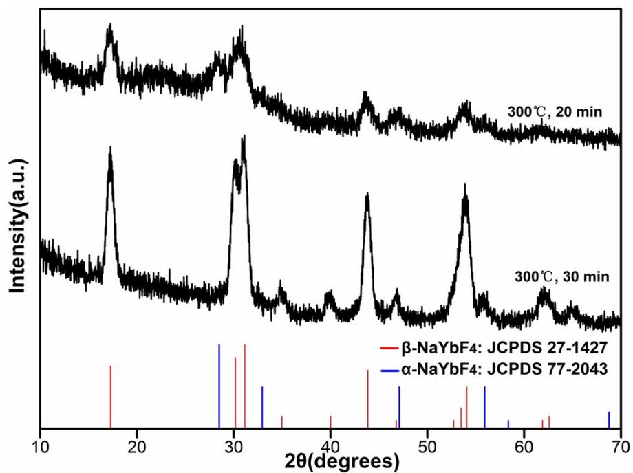
**Figure S6.** XRD patterns of NaYbF<sub>4</sub>:Er prepared by using NaOA-based solvothermal strategy at the NaOA/NH<sub>4</sub>F/RE ratio of 1.9:4.5:1 and different reaction times.
