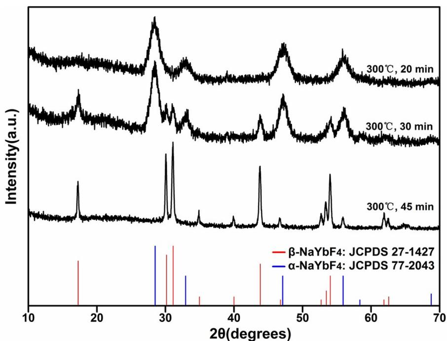
**Figure S3.** XRD patterns of NaYbF<sub>4</sub>:Er prepared by using NaOA-based solvothermal strategy at the NaOA/NH<sub>4</sub>F/RE ratio of 2.5:6:1 and different reaction times.
