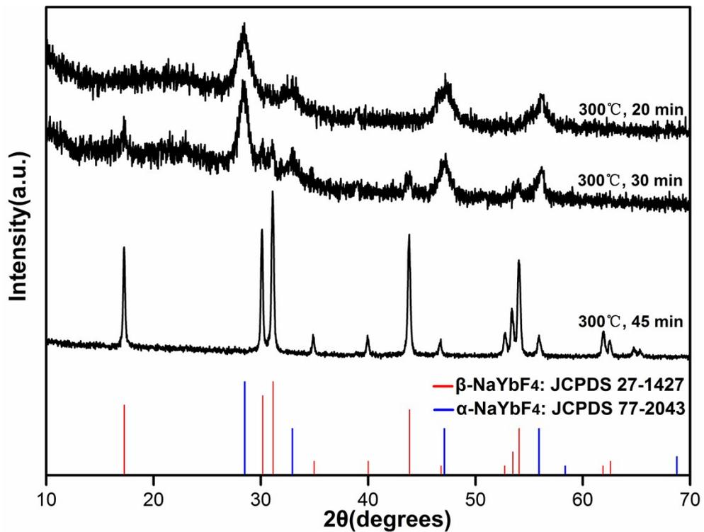
**Figure S8.** XRD patterns of NaYbF<sub>4</sub>:Er prepared by using NaOA-based solvothermal strategy at the NaOA/NH<sub>4</sub>F/RE ratio of 3:6:1 and different reaction times.
