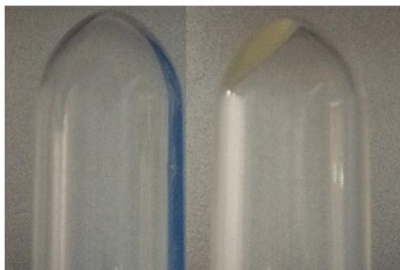
**Figure S4.** Digital photo of the collected precipitate *via* direct centrifugation for the optimized  $\text{NH}_4\text{F}/\text{RE}$  ratio (4.5:1)-based solvothermal system (left) and the high  $\text{NH}_4\text{F}/\text{RE}$  ratio (6:1)-based solvothermal system (right). Both reactions were performed according to NaOA-based solvothermal strategy and were stopped after reacting at 160 °C for 0 min.
