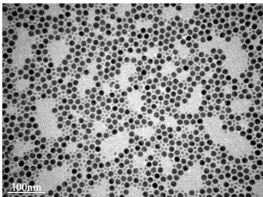
**Figure S7.** TEM image of NaYbF<sub>4</sub>:Er prepared by using NaOA-based solvothermal strategy at the NaOA/NH<sub>4</sub>F/RE ratio of 1.5:4.5:1. The NC growth reaction were performed at 300 °C for 30 min. Narrowly size distributed β-NaYbF<sub>4</sub>:Er can be observed in the TEM image, while there is also a large number of small-sized NCs, indicating the α-to-β transition is still not finished completely.
