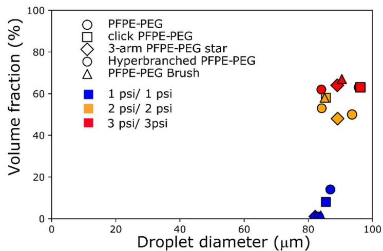
**Supplemental Figure 3.** Characterization of the generation of PBS containing droplets with the different surfactants dissolved at 3% weight in HFE 7500 for three characteristic pressure sets used to flow the oil and the aqueous phases.
