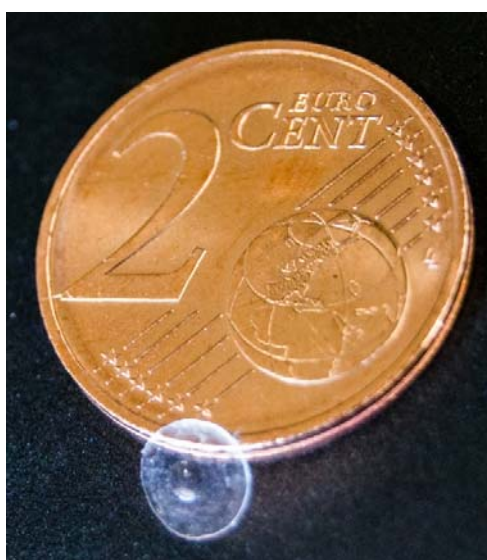
Fig. S4 FEP film with a thickness of 0.05 mm after mechanical stress test.
